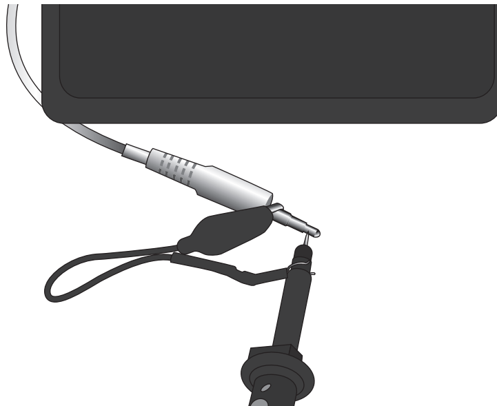
Figure 9-5: Connecting an oscilloscope probe to an audio plug.
