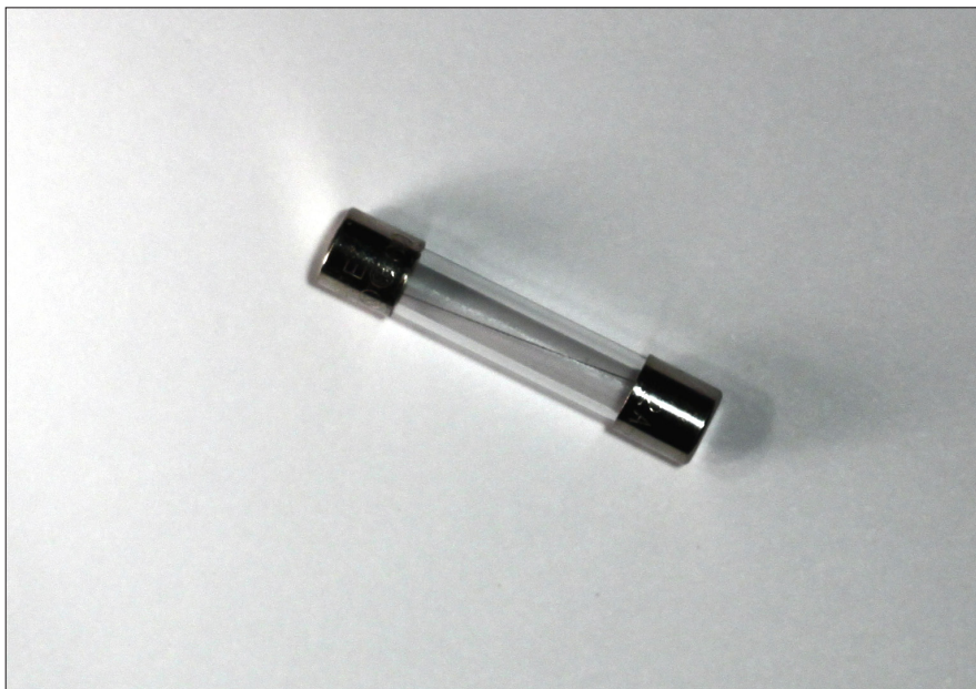
Figure 2-6: A 2 A, 1-1/4" x 1/4" AGC fuse.
