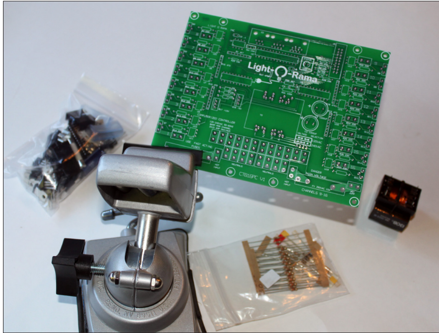
Figure 3-3: Assembling the ShowTime PC circuit board.
