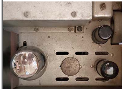
The hole plug for the deleted 6V6 tube socket
