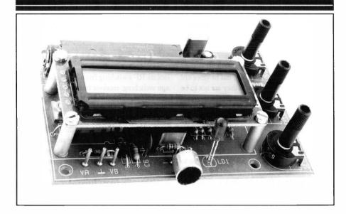
Velleman Kits of Belgium has in its line a Morse Decoder kit which we found to be exceptional in several features. The components are very high quality, including the display. The PCB is one of the best we've seen, with understandable parts-layout design and location, though some very close soldering is required in some instances.
