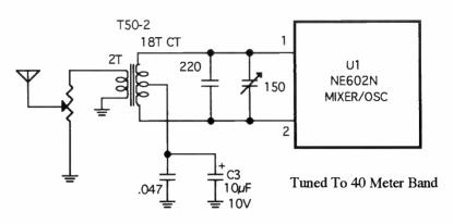
This revision reduces (but does not eliminate) AM broadcast station pickup. I believe the reduction is due to the balanced input, but it might be due to the new High-Q input circuit.
