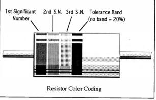
second band specifies the second significant number. The third band specifies the number of zeros to be added to the significant numbers. If there is no fourth band, the tolerance is 20%. If the fourth band is gold, the tolerance is 5%, and if it is silver, tolerance is 10%. The coding system for 1% resistors adds an additional significant number, and thus will have five bands.
