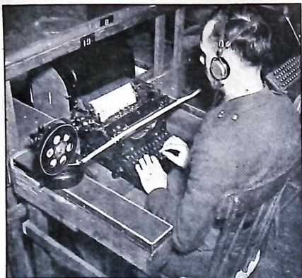
A student at the Enlisted Men's School at the Signal Corps' Fort Monmouth, N. J., Enlisted Men's Division gets slip-reading practice at a high-speed operating position transcribing inked tape on a typewriter.
