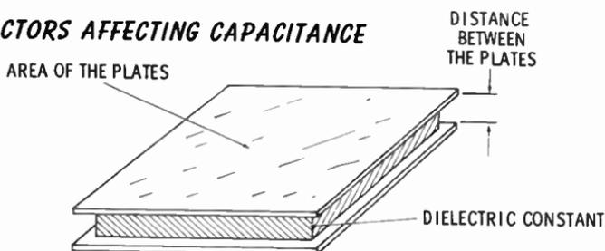
Capacitance (farads) is determined by three factors:
