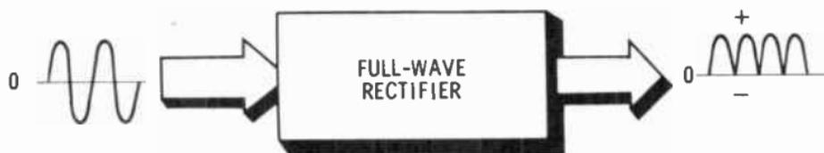
When AC voltage is applied to a full-wave rectifier, the load receives current during both half cycles. Notice that the negative half cycles have been inverted so that all the half cycles are positive at the output of the rectifier. This type of pulsating DC is much easier to smooth (filter) than the output of the half-wave rectifier. Thus, smaller and less expensive components can be used in the filter section.
