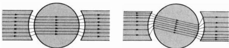
*No Armature Reaction*      *With Armature Reaction*
