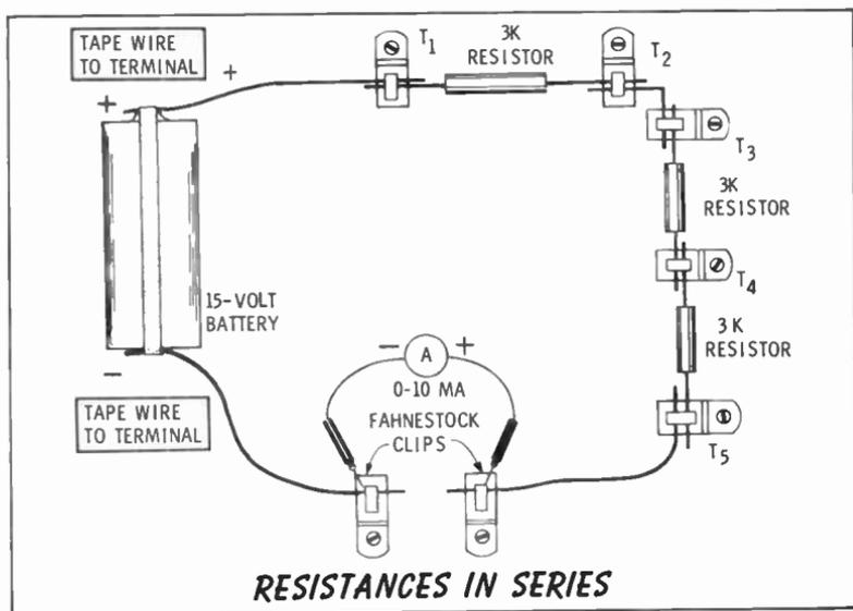
This is logical, because the total resistance in the circuit determines the amount of current allowed to flow with a given voltage source. Therefore, to find the total resistance in a circuit, add the values of the individual resistances.
