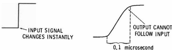
travel from cathode to plate in a vacuum tube is no longer negligible. For the same reason, the time for holes or electrons to diffuse from emitter to collector in a transistor must be considered.
