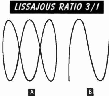
the starting point. The figure is continuous; it has no beginning or end. Figure B, however, is not continuous; it has a beginning and an end. Its pattern is **open**.
