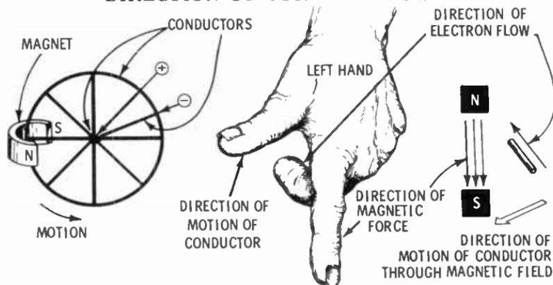
will be. Another factor is the speed at which the lines of force are cut by the wires. The faster the relative motion between the two, the greater the force generating electron flow will be. Finally, the greater the number of wires cutting through the magnetic field, the greater will be the number of electrons that flow.
