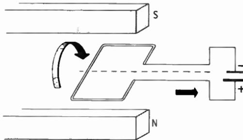
The simple motor shown in the figure above is not very practical. The coil cannot rotate very far because the current always moves through the wire in the same direction. When opposing poles appear opposite each other, the loop stops. Furthermore, any permanent connections to the loop of wire will not allow it to rotate very far.
