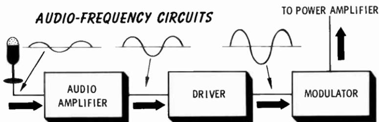
**The Driver**—Like most circuits, the driver obtains its name from its purpose. The driver amplifies the AF to the voltage level required to "drive" the tubes of the modulator. The modulator tubes require large changes in signal amplitude to operate properly.
