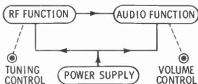
nated as an audio function; the power supply, its filter network, and power cord become the power-supply function.
