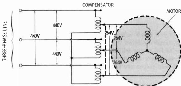
The autotransformer method is shown above. The group of autotransformers used to limit starting current is called a **compensator**. When the motor reaches running speed, the compensator is bypassed and the full voltage is applied. The
