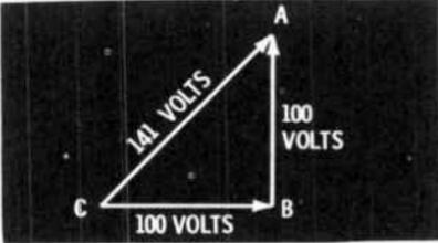
In the figure above, single-phase voltages of 100V exist between A and B and between B and C. The voltage between A and C is 1.41 times the single-phase voltage if the two phase voltages are equal.
