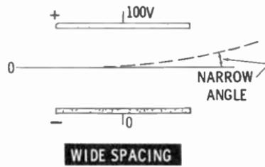
**Difference of Potential**—Intensity of the electric force can also be varied by the difference of potential on the plates.
