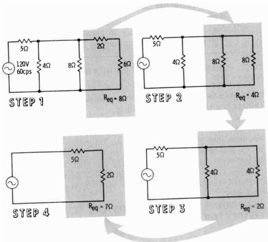
**Q20.** Find the equivalent resistance of the following circuit.
