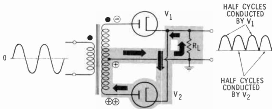
Notice the difference between the pulsating DC from a half-wave rectifier and from a full-wave rectifier. The variation in the output from the half-wave rectifier has half the frequency of the variation from the full-wave rectifier.
