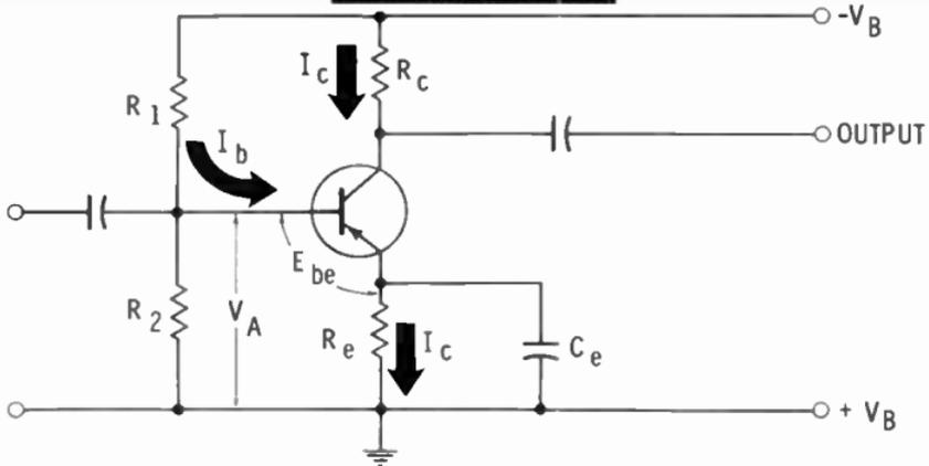
Capacitor  $C_e$  is connected across  $R_e$  to bypass the AC signal current. If this capacitor were not used, signal voltage would be present across  $R_e$ . If this happened, the action just described would tend to reduce the gain of the amplifier. This is one type of negative feedback and is the same action that takes place in a triode amplifier in which the cathode resistor is not bypassed.
