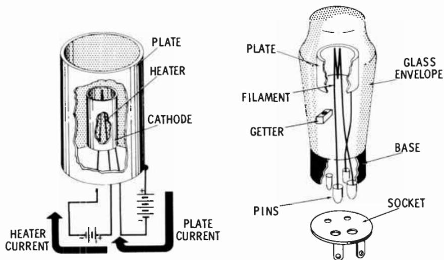
**Indirectly Heated Cathode      Directly Heated Cathode**
