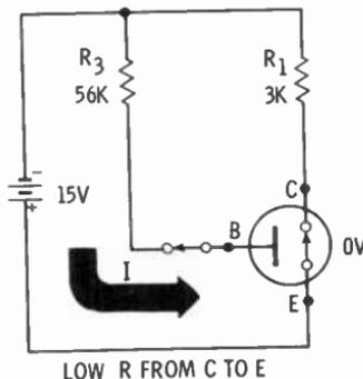
Q7. When a small amount of current enters the B terminal, the transistor acts as a(an) ----- switch and almost (all, none) of the source voltage appears across it.
