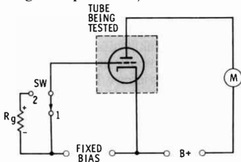
the meter reading if very little or no gas is present. However, if positive gas ions are present, current will flow through  $R_g$  and develop a positive polarity from the grid to cathode. Bias will be reduced, plate current will increase, and an increased reading of the meter will be noted.
