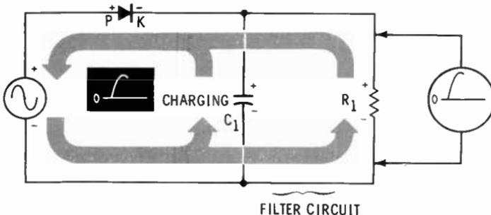
As the source voltage rises to maximum positive, current flows through  $R_1$  and the diode. Some of the current also charges the capacitor to the value of the source voltage.
