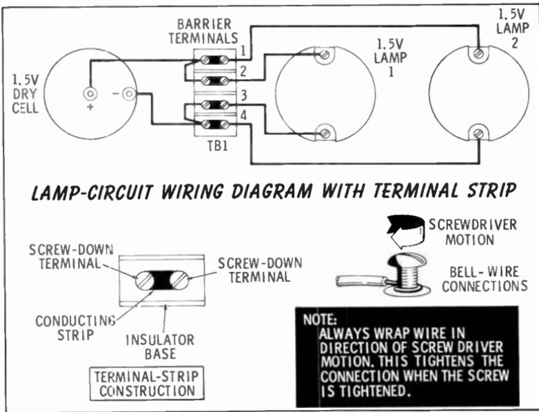
A new part has been added—a terminal board (TB1). As shown in its construction detail, a terminal board has a metal strip with two screws on either end, mounted on an insulating material. These boards serve as connecting points for wires.
