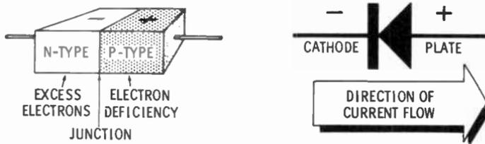
Voltage polarities necessary for current to flow are labeled on the symbol. Current flows through the diode toward the arrowhead.
