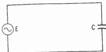
Because the circuit above contains no resistance, the voltage across the capacitor will be the same value as the source voltage at every instant.
