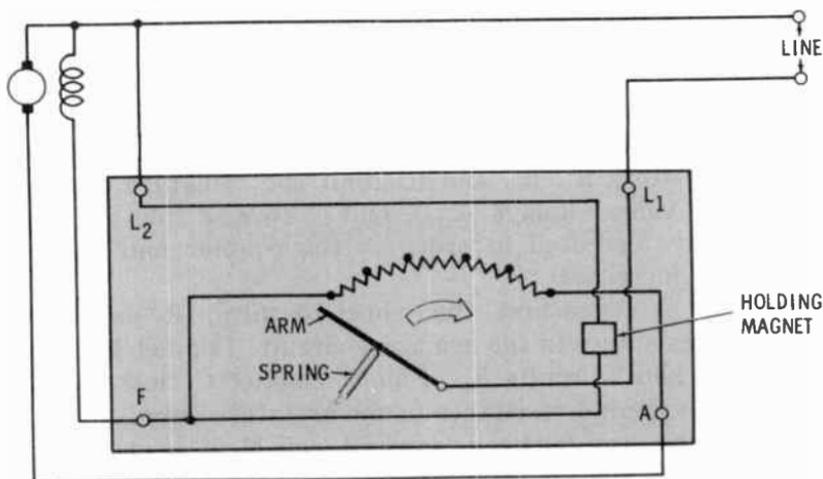
The operation of the **four-point** starting box is similar to that of the **three-point** starting box. However, the holding magnet releases the arm when the voltage, rather than the field current, is lost. The **four-point** box is the more common.
