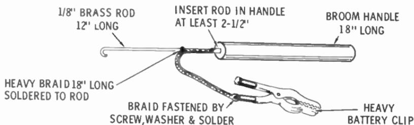
Fasten the clip of the grounding tool to the bare metal of the chassis. Touch the terminals or leads of the capacitor with the tip of the rod.
