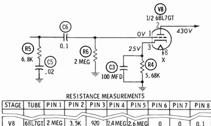
As in the previous example, part numbers and their values are shown on the schematic. If the trouble is isolated to one section of the circuit, the individual parts can then be measured. If, for example, something other than 25V and 920 ohms were read from pin 3 to ground, either  $C_3$  or  $R_4$  would be suspected of causing the trouble.
