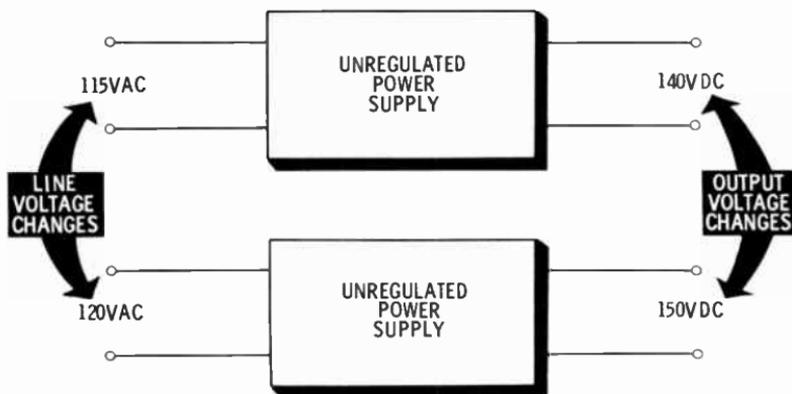
The figure shows an unregulated power supply fed by a line voltage of 115 volts AC. It provides an output voltage of 140 volts DC to its load. Now suppose the line voltage changes to 120 volts AC.
