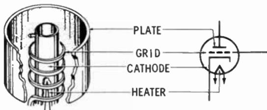
De Forest's experiments proved that the triode could do something that had never been done before—it could make small signals larger. The process of making strong signals out of weak signals is called **amplification**. The triode is often used as an amplifier.
