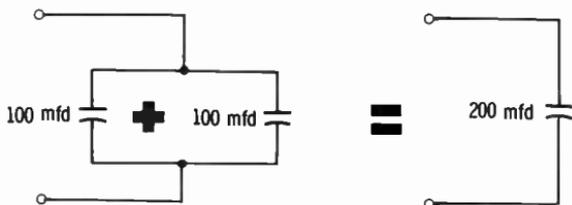
If two capacitors are connected in parallel, you can find their equivalent capacitance by adding their values.
