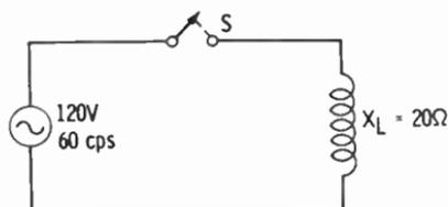
Inductive reactance in a circuit changes with frequency, but inductance stays the same. To find how the above circuit behaves at other frequencies, you must determine the inductance. Use the formula:
