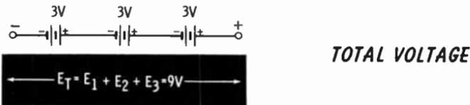
There is a separate problem in the calculation of total voltage, however. Some of the voltage sources may be in opposition to others, in which case the total voltage will not be the simple numerical sum of all the voltages. If the polarities of all the voltage sources are in the same direction, the voltage values are added together. If the polarities are in opposite directions, the values are subtracted, and the polarity of  $E_T$  is that of the larger voltage source.
