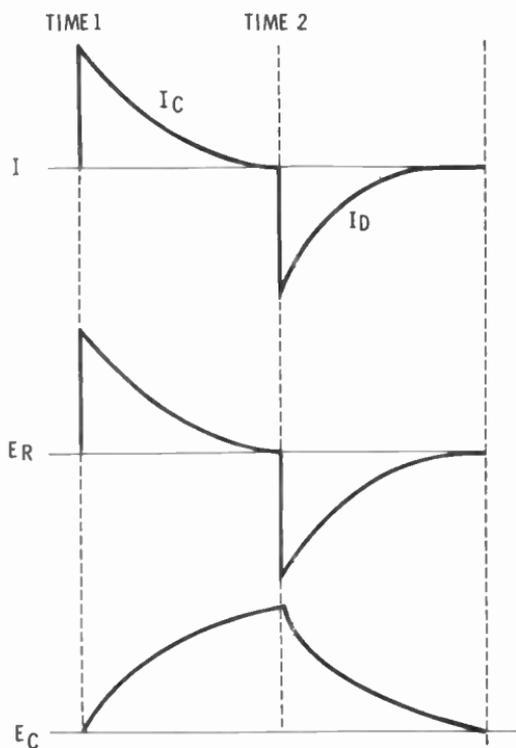
Q62. Refer to the top figure on the facing page. At the instant the switch is placed in position 1, is  $E_R$  equal to, greater than, or less than  $E_c$ ?
