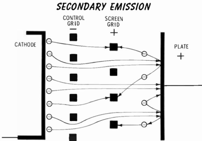
When the screen-grid voltage is equal to or greater than the plate voltage, the amount of current drawn by the screen grid is enough to disturb the operation of the tube. This problem was solved by the development of the **pentode**.
