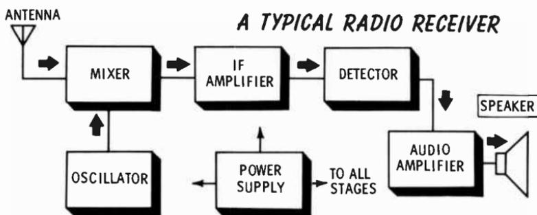
The purpose of the radio receiver is to convert the amplitude modulation on the carrier back to its original sound. As the carrier increases in ever-widening circles on leaving the transmitter antenna—like ripples in a pool—its energy decreases in amplitude. The increasing circumference of the circles causes power in the waveform to be distributed over an ever-increasing area. By the time the signal reaches the receiver antenna it is rather weak, usually around a few
