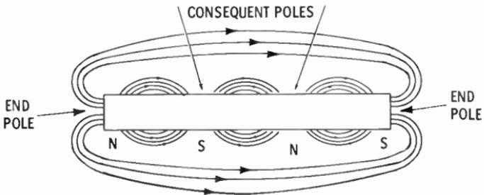
The poles between the ends of a magnet are called **consequent poles**. Notice there are magnetic fields existing between the consequent poles and the end poles. These fields are the same as the field that exists between the end poles. The magnetic lines of force leave a north-seeking pole and enter a south-seeking pole.
