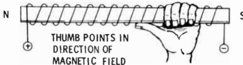
FINGERS POINT IN DIRECTION OF ELECTRON FLOW THROUGH WIRE.
