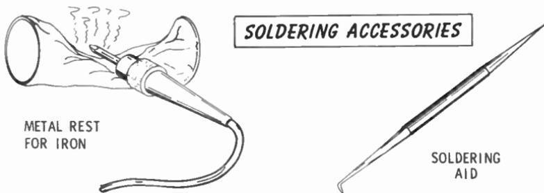
**Soldering Aids**—Soldering aids come in several shapes. They are used primarily to remove excess solder during soldering and unsoldering. The one shown above has a sharp point and hook. An ice pick can also be used.
