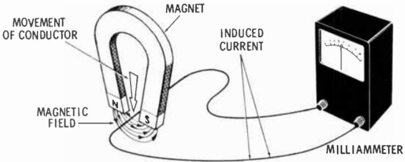
If a coil is connected to an ammeter and a bar magnet is moved through the coil, the ammeter will show that an electric current flows. This current is **induced** by the magnetic field only. If you move the bar magnet back and forth through the coil continuously, the induced current will be AC. Use the lowest amperage range on the multimeter for this experiment.
