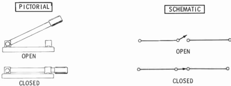
The arrowhead has no real significance other than helping to identify the symbol as a switch when it is shown in a closed position. Without the arrowhead, the symbol would look like a wire between two terminals.
