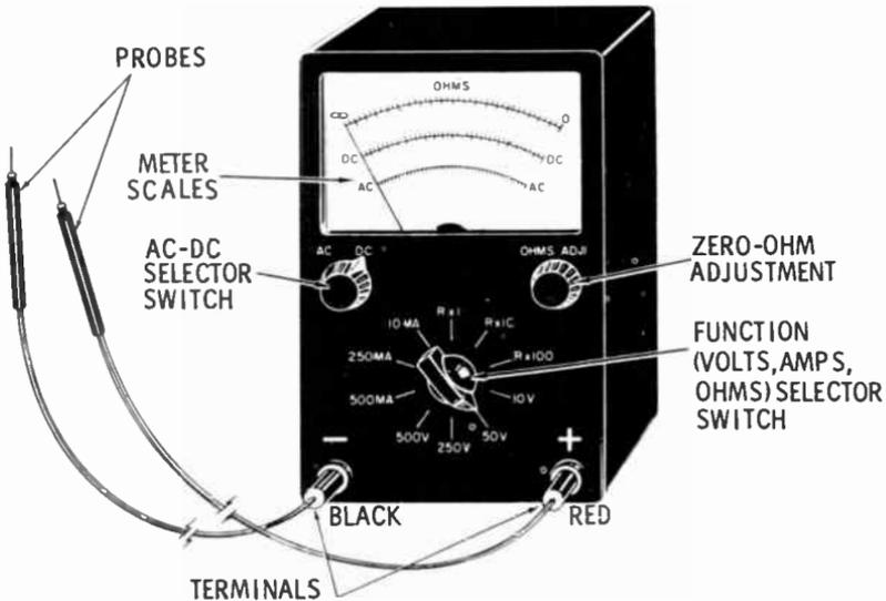
The front panels of some multimeters do not look like this one. Each, however, has a similar means of accomplishing the same measuring tasks.
