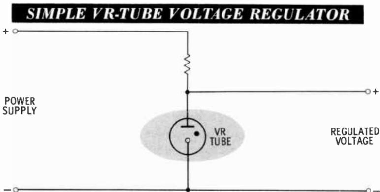
The limiting resistor in series with the VR tube is selected to limit the current through the tube to a safe value. Gaseous voltage regulators keep the output voltage constant to within about 1%. They come in a number of specific voltage
