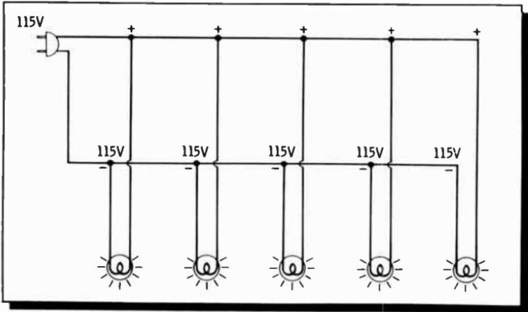
Another form of parallel circuit uses more than one voltage source in parallel to increase the availability of current. The greater the amount of stored energy available, the longer the source can produce a current at a given voltage.
