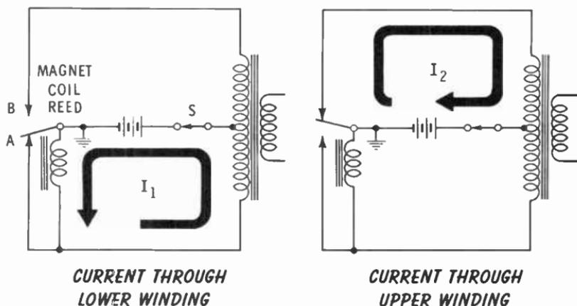
The vibrating reed causes the current to flow through first the lower section of the transformer primary and then the upper section. This is very much like having an alternating current flowing in the primary. This action causes an AC voltage to be induced in the secondary of the transformer. The voltage is not a sine wave, however, but has a generally rectangular shape. Filtering action can smooth out the waveform.
