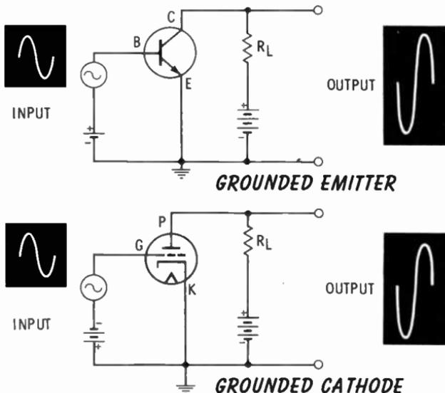
tively. A phase reversal of  $180^\circ$  occurs between the input and the output. This phase reversal will be explained in the chapter on triode amplifiers. The common-emitter amplifier has these characteristics:
