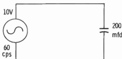
You have already learned that when a sine-wave AC voltage is applied, the current in a capacitor always leads the voltage by  $90^\circ$ . You have also learned that a capacitance consumes no power; all the energy it takes out of a circuit in one quarter cycle is returned in the next quarter cycle.
