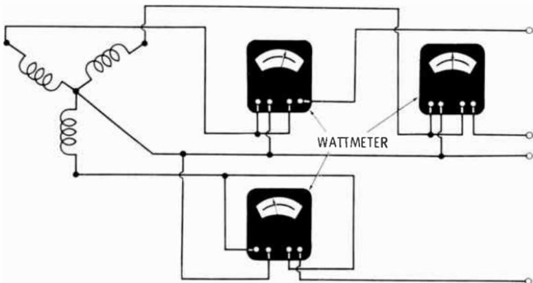
anced and unbalanced systems. Three wattmeters are simply used to measure the power in all three phases. A typical connection is shown at the bottom of the opposite page.
