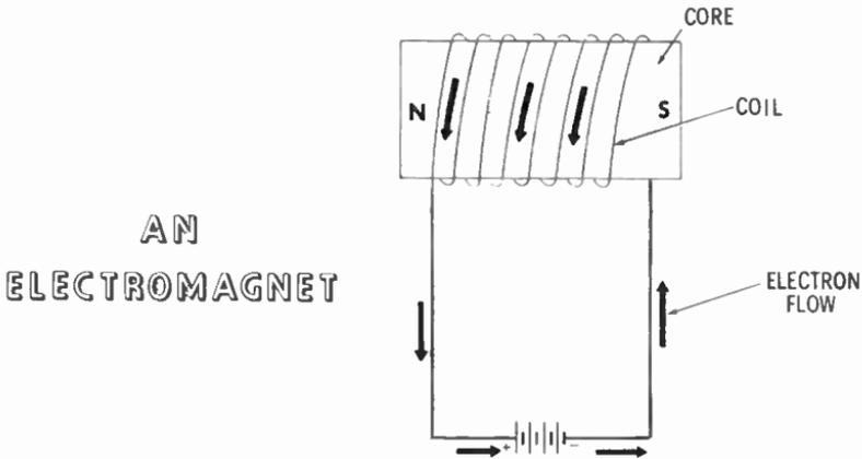
When a current flows through the coil, a magnetic field is produced around the coil. If the core conducts the magnetic lines of force easily, it becomes a temporary magnet when current flows through the coil. The current supplied to an electromagnet is DC, since AC would cause the polarity to constantly change.
