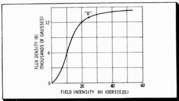
The flux density increases rapidly with only a slight increase in the magnetizing force when the core material is at a point of low field intensity (only a few thousand magnetic lines of force). At a point of high field intensity, a large change in the magnetizing force is required to cause a small change in flux density. Point X indicates the point of saturation.
