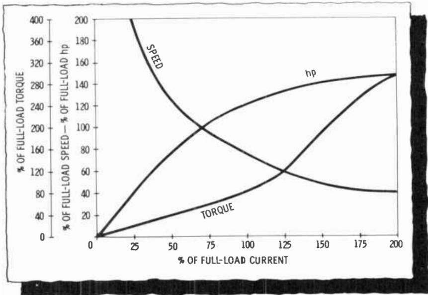
a heavy load and faster with a light load. If a DC series motor is run without any load, it may run so fast that it may damage itself. Series motors are seldom used in applications requiring belt coupling to the load; if the belt should break, the motor would be without a load. A typical use of a series motor is the automobile starter.
