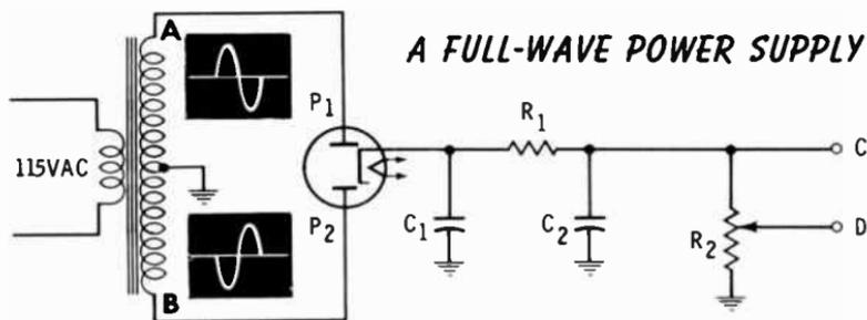
The transformer steps 115 volts AC up to the value desired on the secondary. Each terminal of the secondary is connected to a separate plate of the **twin diode**. The secondary winding of the transformer is center-tapped to ground.
