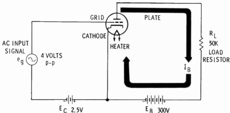
the grid voltage for a particular type of tube used in the circuit shown above. The plate current changes from 1.2 to
