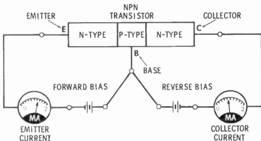
The figure shows an NPN transistor biased properly to operate as an amplifier. Addition of certain resistors (which you will see later) would complete the picture.
