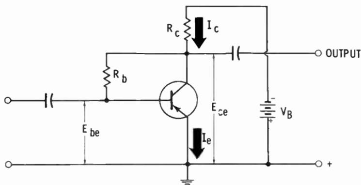
If  $I_c$  increases in the above circuit, the voltage drop across  $R_c$  increases. Since the supply voltage ( $V_B$ ) is relatively constant,  $E_{ce}$  must decrease as the voltage across  $R_c$  increases. The base-emitter junction and  $R_b$  are connected in series across  $E_{ce}$ . Therefore, the base current depends on  $E_{ce}$ . This means that as  $E_{ce}$  decreases, base current and  $I_c$  decrease, and the original increase in  $I_c$  is opposed.
