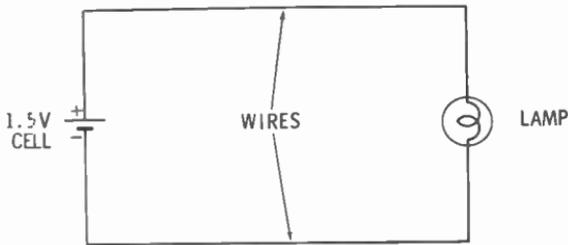
The lamp and cell symbols are connected by lines representing wires. Note that the lines run in only two directions—horizontal and vertical. Slanted or curved lines lessen the clarity of a diagram. Also note that a voltage value and polarity markings appear on the cell.
