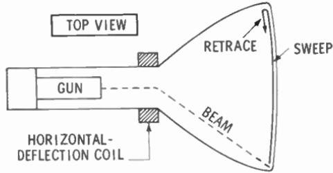
A horizontal-deflection coil wrapped around the neck of the tube moves the beam from side to side. Current moving through the coil sets up a magnetic field which has an attracting and a repelling effect on electrons similar to positive and negative voltage. The stronger the field, the greater is its effect on the beam. To increase the strength of the field requires an increase in current through the coil. The illustration shows the beam deflected to the left.
