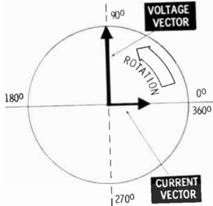
Inductance, unlike resistance, **consumes no power**. When the current in the circuit is **increasing**, inductance takes energy out of the circuit. It converts this energy into a magnetic field. When the current in the circuit is **decreasing**, however, this magnetic field collapses, and **all the energy returns to the circuit**. Energy is borrowed, but none is used.
