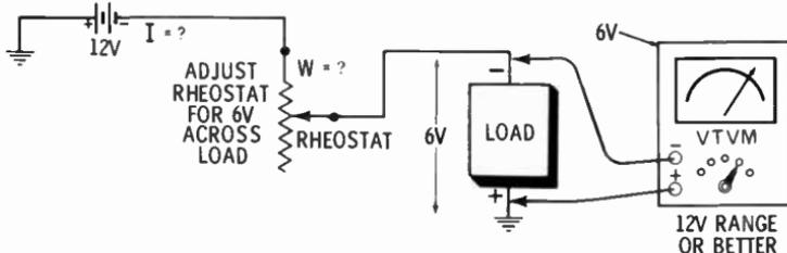
permit the desired amount of current to flow through the device. It must also have the proper wattage rating as determined by its current and voltage drop. A rheostat
