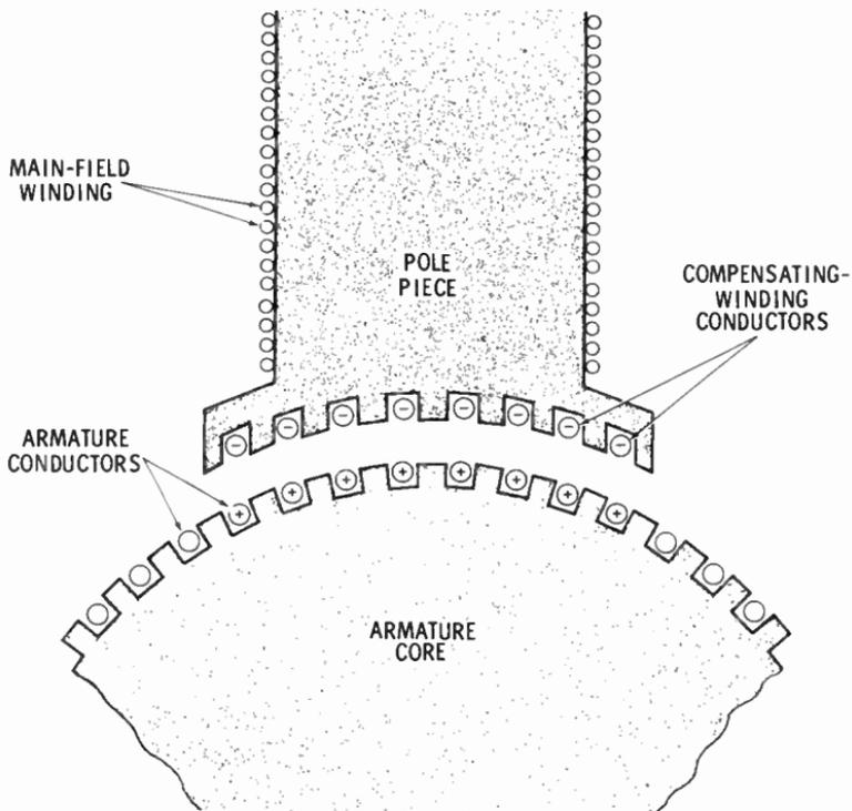
in the faces of the pole pieces. They are connected in series with the armature coils, like interpoles, but are wound in the opposite direction from the armature coils. The field
