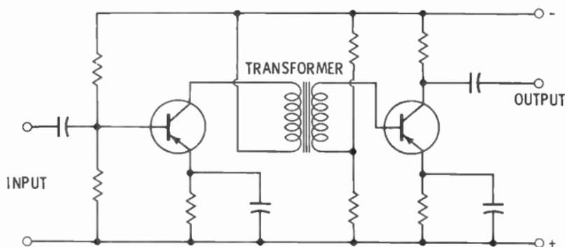
Suppose the output impedance of the first stage is 25K and the input impedance of the second stage is 1,000 ohms. What turns ratio would the coupling transformer need? In a transformer, the impedance ratio is equal to the square of the turns ratio. The required turns ratio may be calculated as follows:
