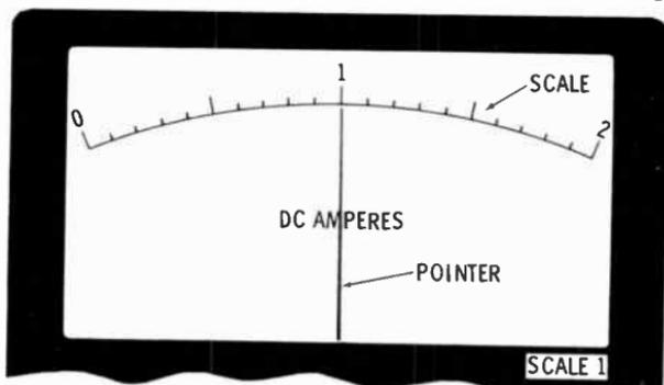
If the needle points to a division mark between two numbers, the decimal value of the division is added to the lower number.
