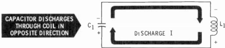
um level across  $L_1$ . As discharge current begins to decrease, the field starts to collapse, developing a coil current in the same direction as the capacitor current.
