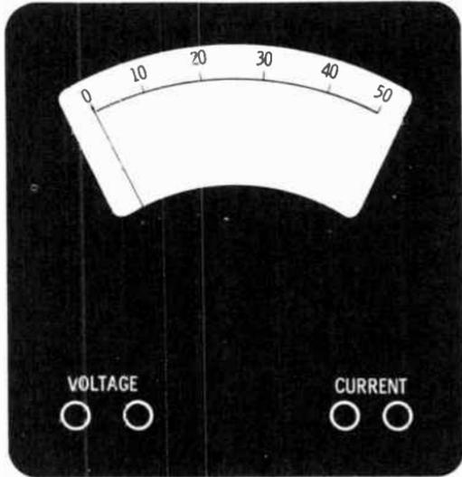
voltage and phase current and gives a reading indicating phase power. In order to find the total power, add all three readings directly.
