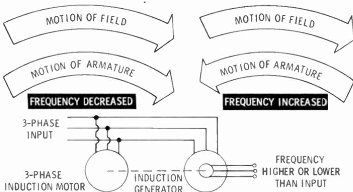
The power source is used to drive an AC motor. At the same time, it is used to establish a rotating magnetic field.
