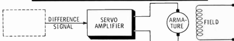
Voltage across the shunt field is obtained from a source separate from the servo system. This produces a uniform magnetic field. Voltage fed to the armature is controlled by the output of the servo amplifier (DC). Speed of the motor is determined by the magnitude of the voltage difference between terminals 1 and 2. Direction of armature rotation is determined by the polarity of these voltages.
