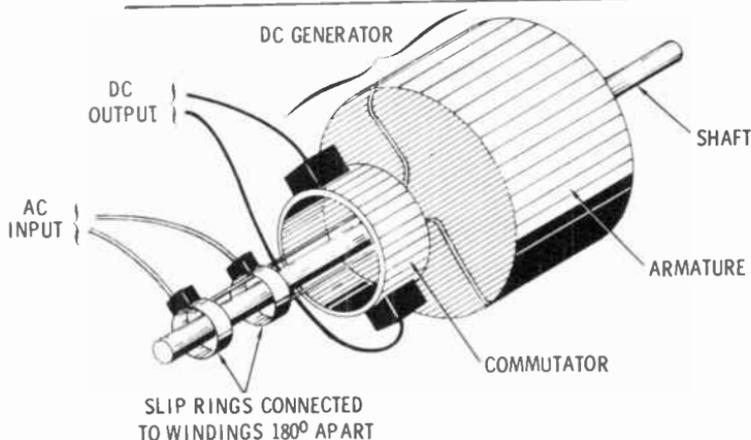
Under ordinary conditions, an alternating voltage is connected to the motor portion of the converter through slip rings, causing the machine to rotate at synchronous speed like an AC synchronous motor. At the same time, the machine also acts like a DC generator. This DC output is taken from the commutator by brushes and can be used to provide current for the field winding. This DC output can, in addition to energizing the field winding, furnish DC to an external load.
