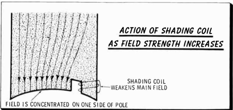
site side of the pole piece. The result is that the field in the part of the pole piece inside the shading coil reaches a maximum intensity later than the rest of the field. As the field in the part of the pole opposite the shading coil begins to decrease, the shading-coil field will start aiding the main field, and the concentration of flux moves to the other edge of the pole piece. The resulting field in the part of the pole piece inside the shading coil reaches zero after the main field.
