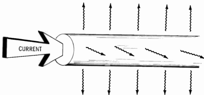
given off by a wire is determined by the type of metal in the wire and the quantity of current that is forced through it. A large current produces more heat in the same size and type of wire than a smaller current. If the current is the same, a smaller wire gives off more heat than one that
