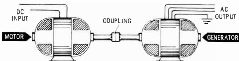
A DC motor chosen as the prime mover in an M-G set must have speed characteristics that are very constant. If the speed of the motor varies considerably as the load increases, the frequency of the AC generator will vary accordingly. (Frequency is directly proportional to the speed of the prime mover.) One suitable type of DC motor is the shunt motor, although compound motors are also used to a great extent. A series motor could not normally be used because of its poor speed control.
