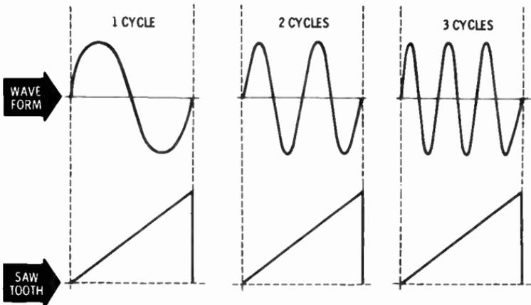
The sweep frequency should always be kept lower than or equal to the waveform frequency; it should never be higher. If the sweep frequency were higher, only a portion of the waveform would be presented on the scope.
