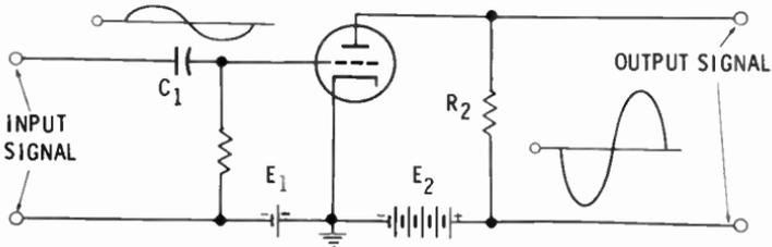
The changing current of the tube passes through  $R_2$  on its return to voltage source  $E_2$ , causing the voltage across  $R_2$  to change in the same manner as the changes of the signal voltage. Since a small change in grid voltage causes a large change in tube current, the changes in output voltage across  $R_2$  are greater than the corresponding input changes on the grid. Thus, the signal has been **amplified.**
