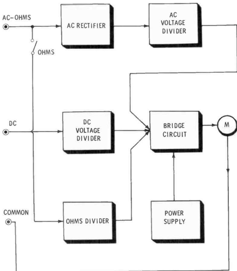
The above block diagram of a VTVM shows three input jacks for test leads. By following the arrows, you can see that when measuring AC, the input current flows through a rectifier, a voltage divider, a bridge circuit, and the meter before it returns through the **COMMON** pin jack. Current, representing DC and ohm readings, flows through the respective divider networks in the circuit to the bridge circuit and the meter. From there it returns to the **COMMON** jack.
