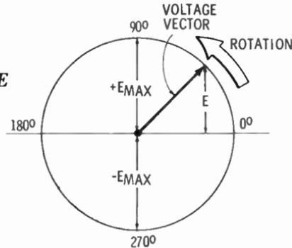
One complete cycle of a sine wave (from zero to a positive peak, down to a negative peak, and back to zero) simply represents one complete rotation of the voltage vector.
