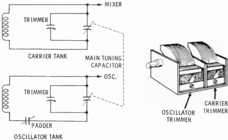
To arrive at the best tuning, the trimmers and padder are adjusted for a maximum reading on the output indicator. As shown in the diagram above, the trimmers are in parallel across the respective sections of the main tuning capacitor. The padder is in series with the coil and main capacitor section of the oscillator tank.
