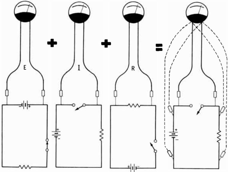
A multimeter can be used to measure voltage, current, and resistance within the limits of several ranges of values. From the technician's point of view, all multimeters consist of three basic sections—meter, circuitry, and front panel.
