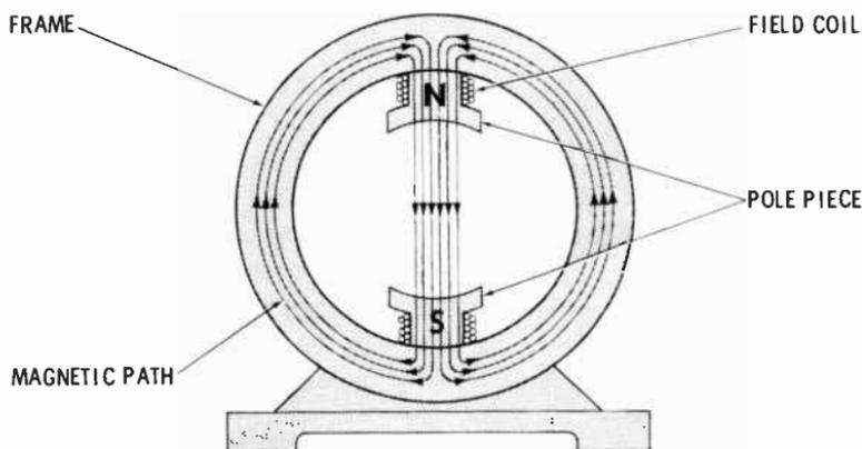
At one time, most generator frames were made of cast iron. Cast iron is heavier than steel and has a poorer **permeability** (ability to conduct magnetic lines of force), so it is used less frequently now. The frames of large generators are made of steel castings; those of smaller generators are made of rolled sheet steel. The frame of the generator also includes a base or mounting brackets.
