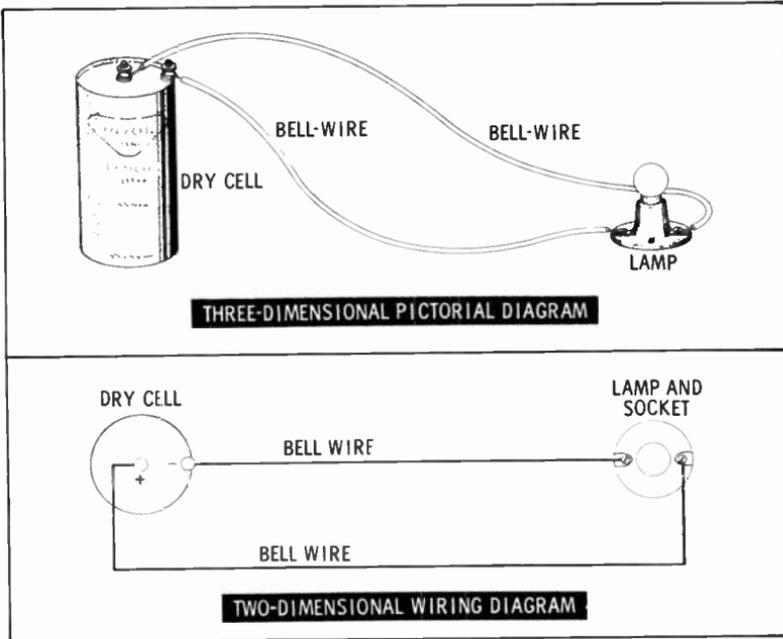
Note how easy it would be to follow the two-dimensional diagram if you were to construct the circuit. The symbols are easily identifiable. The dry cell is a flat circle (top view) with terminals in the correct positions and polarity markings shown. The lamp symbol is two circles, a bulb in a base, plus two terminals. Wires are straight lines, and the parts are labeled.
