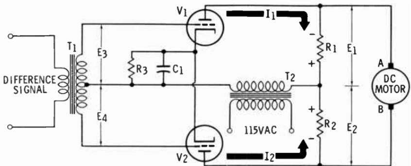
The servomotor used in such a circuit will probably be one with permanent-magnet poles. The secondary of  $T_2$  applies an AC voltage to the plate of  $V_1$  and  $V_2$ . As can be seen, the plate voltages are in phase. The difference signal enters through  $T_1$  and is applied to the two grids  $180^\circ$  out of phase.  $C_1$  and  $R_3$  form the common-cathode bias for both tubes. With no signal applied across the primary of  $T_1$ , each
