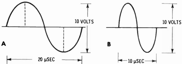
The time line for a waveform usually represents the duration of one cycle. In Part A above, it is 20 μsec and in part B it is 10 μsec. From this, the duration of a portion of a cycle can be determined. In part A, a half wave (half of a full cycle) is 10 μsec. A quarter wave (fourth of a full cycle) in part A is 5 μsec.
