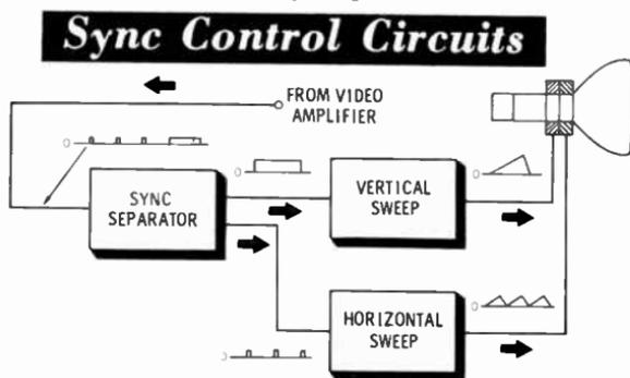
**Sync Separator**—Sync pulses arrive at the sync separator from the video amplifier. There is one narrow sync pulse for each line of scan. This pulse is intended to control the starting time of each horizontal sweep across the screen. When one field of  $262\frac{1}{2}$  lines has been completed, the video waveforms are followed by a sync pulse many times wider than the horizontal sync pulses.
