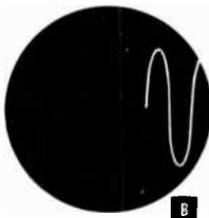
Which control would you adjust for figure A? Which would you adjust for figure B? The waveform in figure A can be adjusted by turning the **VERT POS** control to bring the waveform to the center of the screen. The waveform in figure B can be adjusted by turning the **HOR POS** control to bring the waveform to the center of the screen.
