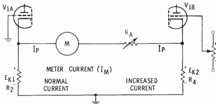
Suppose a positive voltage is applied to the grid of V<sub>1B</sub>. Plate current in V<sub>1B</sub> will increase, raising the voltage across R<sub>4</sub>. E<sub>K2</sub> will now be a larger positive voltage than E<sub>K1</sub>. Current will therefore flow from left to right through the meter.
