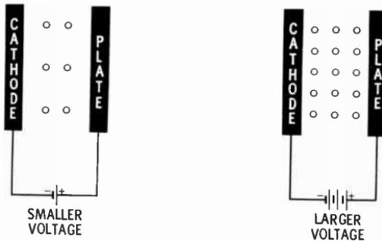
**CURRENT FLOW IS AFFECTED BY PLATE VOLTAGE**
