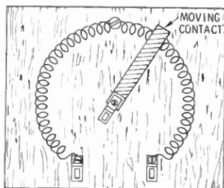
By inserting the rheostat into a circuit with one wire connected to the rotating arm and the other to one of the terminals, a desired value of resistance can be selected.
