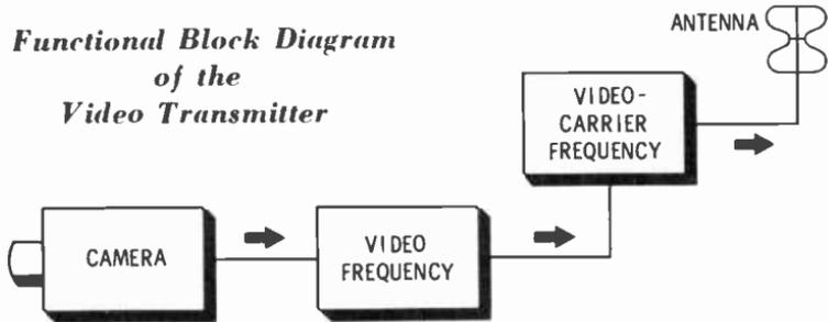
In the video-frequency section, video signals from the camera are amplified and fed to the final power amplifier of the carrier-frequency section. Here, the carrier is amplitude-modulated by the video.
