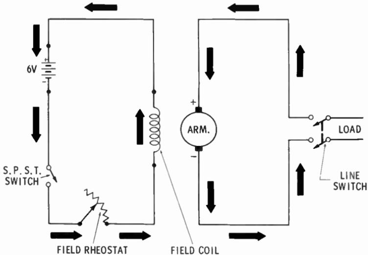
Notice that the separately excited magnetic-field circuit is completely independent of the generator circuit. The strength of the externally excited magnetic field depends directly on the amount of current supplied by the external DC source. A rheostat is used to vary the strength of the magnetic field. This provides a very sensitive control of the generator output.
