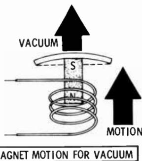
As in other phones, this diaphragm vibrates at the frequency of the sound waves striking it. As it vibrates, the bar magnet moves back and forth within the coil. This induces a current which changes direction at the same frequency as the sound. If the transmitter is connected to a sound-powered receiver, current will flow back and forth through the circuit.
