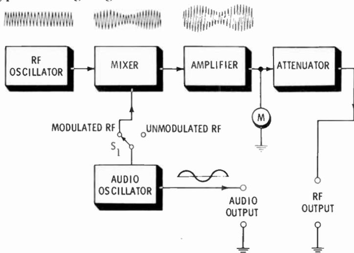
Notice that the RF and audio oscillators are connected to a mixer stage when  $S_1$  is in the MODULATED RF position. The mixer circuit superimposes the audio on the RF carrier and feeds the modulated wave to the output through the amplifier, attenuator, and meter. When  $S_1$  is in the UNMODULATED RF position, a pure carrier frequency appears at the RF OUTPUT and an audio signal is fed to the AUDIO.
