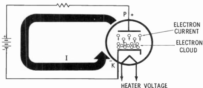
**The Plate**—The plate (sometimes called an **anode**) is a metal cylinder mounted around the cathode. With a battery connected to the diode as shown in the diagram, current flows through the tube. Negative voltage on the cathode (symbol K) repels the negative electrons from the cloud toward the plate (symbol P). Positive voltage on the plate attracts the electrons. Current flows from the plate through the external load, through the battery, and back to the tube via the cathode.
