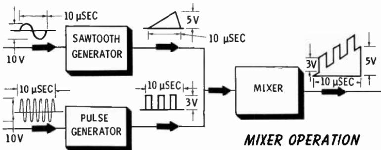
The sawtooth and pulse generators have sine-wave inputs of different frequencies. The input frequency of the pulse
