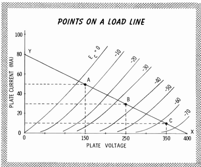
If the amplitude of the AC input signal is known, it can be marked off along the load line, as shown in the figure.
