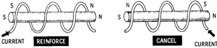
When current flows in the coil, the electromagnet will either add to, neutralize (cancel out), or subtract from the magnetic field of the permanent magnet. Polarized electromagnets are used in telephone and telegraph circuits. The figure below shows a diagram of a telephone-bell circuit.
