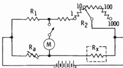
$R_a$  may be a single wirewound potentiometer with values calibrated on a front-panel scale, or it may be several decade (10-position) switches in series. One switch adds resistances in multiples of one, a second in multiples of 10, etc.
