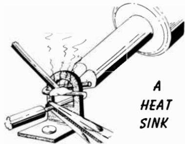
The correct positions of iron, connection, and solder while soldering splices is shown below. Let the solder flow to the iron through the connection.
