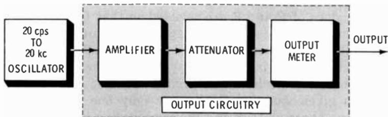
Usually the output circuitry contains an amplifier with a network or attachment that permits matching the impedance of the external circuit to that of the generator. If the impedance mismatch is severe, the generator may be loaded down enough to change the oscillator frequency.
