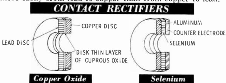
The **selenium** rectifier is made by depositing a layer of selenium on an aluminum plate. An alloy with a low melting point is then sprayed onto the selenium surface. This alloy is called the **counterelectrode**. The current-blocking layer is the surface between the selenium and the alloy. Electrons flow through this surface easily in one direction but not in the other.
