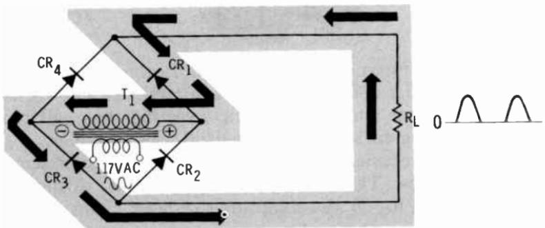
On the positive half cycle, current flows through CR<sub>3</sub>, up through the load resistor, and back through CR<sub>1</sub>. CR<sub>2</sub> and CR<sub>4</sub> are reverse-biased and act like open switches.
