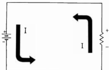
**A3.** A basic circuit is a fundamental series circuit.
