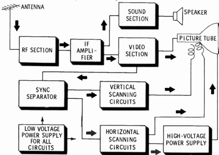
The illustration above shows a single antenna bringing both the FM sound carrier and the AM video carrier to the RF (radio frequency) circuits. This is satisfactory since the sound- and video-carrier frequencies are fairly close together (the sound carrier is 4.5 megacycles higher).
