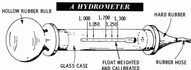
If the hydrometer reading is 1.210 to 1.220, the cell has a full charge. If the reading is 1.180 or less, the battery needs to be charged. If the reading is as low as 1.060, the battery is completely dead. A battery will rarely have the same reading for all cells. When using the hydrometer to check the battery, always keep the small tube or tip over the cell being checked so the electrolyte will drip back into the cell. After using the hydrometer, rinse it with water to remove any acid.
