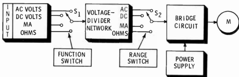
shown. The function switch ( $S_1$ ) connects the jacks to the proper voltage-dividing networks. The range switch ( $S_2$ ) selects the proper network, usually resistive, to supply the bridge circuit with the correct voltage. The bridge circuit provides the amount of current that should flow through the meter for the correct pointer deflection. The power supply provides filament and  $B+$  voltage to the vacuum tubes.
