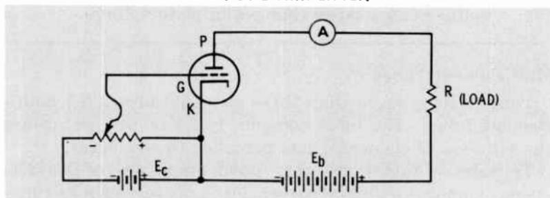
Battery  $E_b$  is connected in such a way that the plate is positive with respect to the cathode. In an actual circuit the positive voltage for the plate is normally obtained from a power supply. Battery  $E_c$  places a negative voltage on the grid with respect to the cathode. A resistor takes the place of this battery in an actual circuit.
