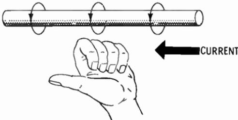
**A16. In what plane do the magnetic lines around a current-carrying conductor lie?**
