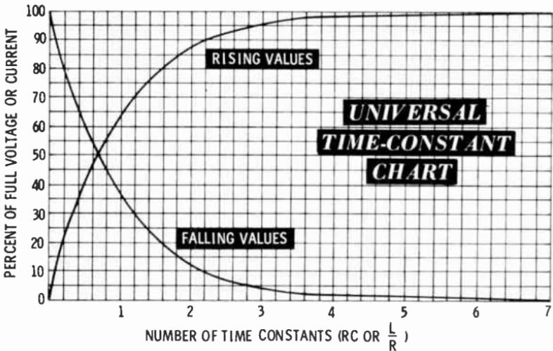
A **universal time-constant chart** can be used to calculate the growth and decay of voltage and currents in any RL or RC circuit to which a sudden step voltage is applied. All you have to know is the final voltage and current, and the time constant of the circuit.
