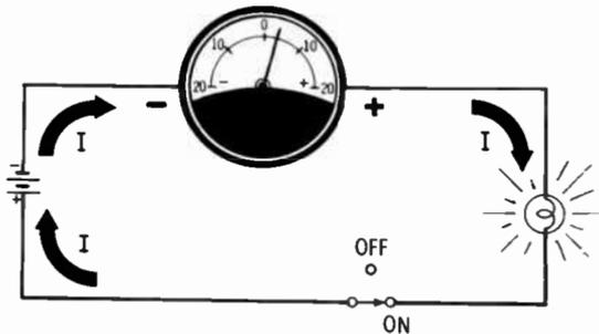
indicates plus, the auto is getting electrical power from the generator and, at the same time, the battery is being charged. Therefore, a minus meter reading indicates the battery is being used, and a positive meter reading indicates the battery is being charged. Before the days of long trips and dependable voltage regulators on the automobile, the operator had to watch the ammeter very closely.
