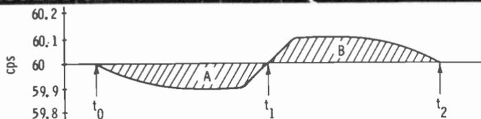
At time  $t_0$ , a situation such as a heavy load lowered the frequency to 59.9 cps. At time  $t_1$ , the automatic device sensed the loss and forced the frequency to 60.1 cps until time  $t_2$ . At that time the machine had caught up with itself. Shaded areas A and B on the diagram must be equal in order for the machine to be caught up.
