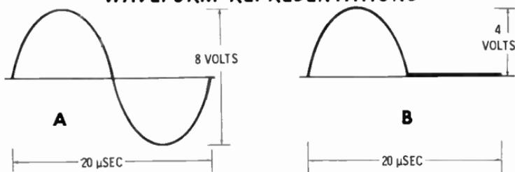
Part A above shows the same sine wave as on the preceding page. The dimensions are 8 volts from its positive peak to its negative peak. The time duration of one cycle is 20  $\mu\text{sec}$  (microseconds). (A microsecond is one-millionth of a second.) Part B shows the same waveform after it has been rectified (using a diode circuit, for example). The single peak remaining is 4 volts from zero to maximum positive. The time duration of the cycle is still the same 20  $\mu\text{sec}$ .
