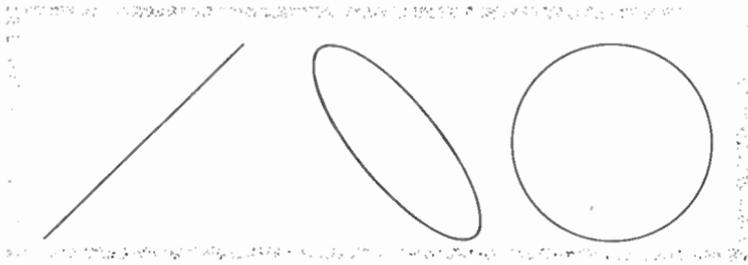
Frequency relationships can be determined by the number of loops or points that touch the top (or bottom) and one of the sides of the pattern. In the figures you have seen so far, there is one point of tangency at the top and one at the side. The frequency ratio is 1/1; the unknown has the same frequency as the standard.
