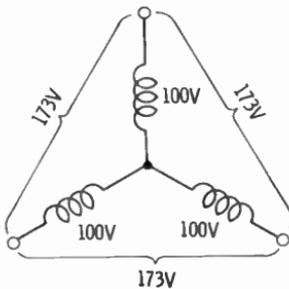
**VOLTAGES IN A WYE-CONNECTED, THREE-PHASE ALTERNATOR**
