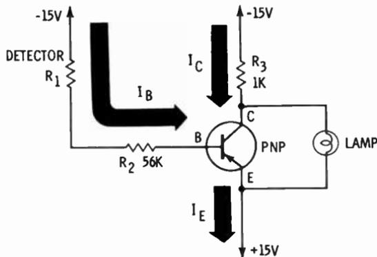
*Current Flow in the Transistor Alarm Circuit*
