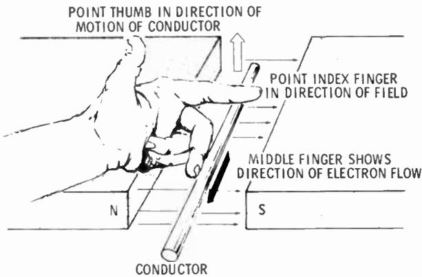
The left-hand rule for generators is shown above. This is an easy way of remembering the relationship between the direction of the magnetic field, the direction of motion of the conductor, and the direction of the induced current.
