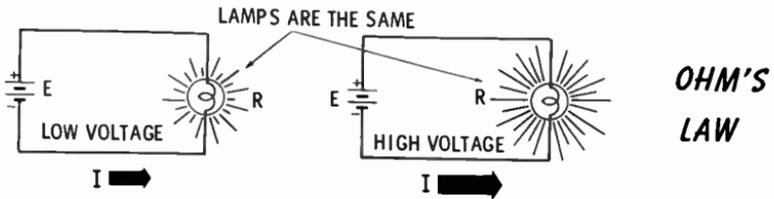
The circuit with the lower voltage will not have as much current flow as the other. The current will therefore be greater in the circuit on the right.
