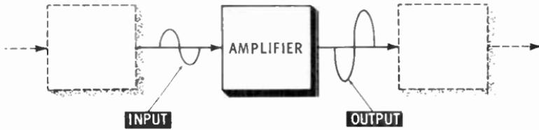
An amplifier, for example, usually receives a small signal from a preceding stage and converts it to a larger signal. In other words, the stage amplifies the signal.
