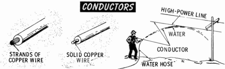
Some materials are better conductors of electricity than others. The availability of more free electrons in silver and copper, for example, makes them better conductors than iron or steel.
