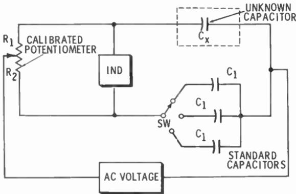
By manipulating a switch, one of several capacitors can be selected as a standard, depending on the size of unknown  $C_x$ . A calibrated potentiometer adjusts the bridge ratio ( $R_1/R_2$ ) for a null reading on the indicator. With this arrangement the arm of the potentiometer can be connected to a pointer that moves on a scale calibrated in capacitance values. This will be true only if all of the standard capacitors increase in value by the same multiple.
