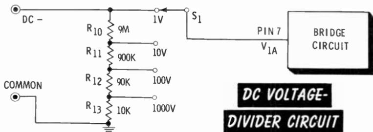
to the COMMON jack. A schematic representation of a four-position switch is shown at the right of the voltage divider. Each position represents a tap in the resistor string. Each tap corresponds to a range setting.
