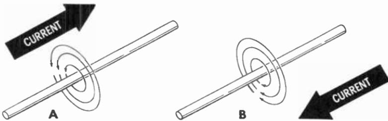
2. **Magnetic lines of force cutting through a conductor cause current to flow in that conductor.** The field must be **moving**. In a single conductor, the current is very small. If the conductor is formed into a coil, many turns will be cut by the moving field, thus developing a larger current. An example is shown below.
