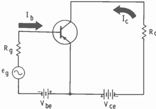
The voltage across load resistance  $R_L$  (which is a separate property of the circuit) is  $\Delta I_c R_L$ , where  $\Delta I_c$  is the signal current in the collector circuit.
