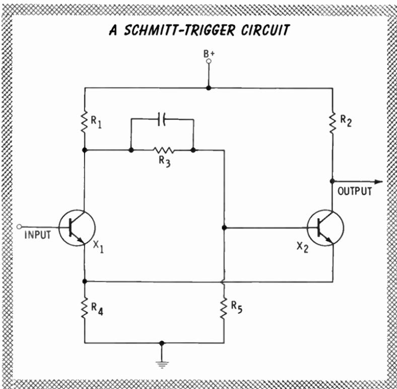
With no input, transistor  $X_1$  is cut off, and its collector voltage equals the battery voltage. This voltage is coupled to the base of  $X_2$  through  $R_3$ . Transistor  $X_2$  is therefore saturated. Due to the emitter current of  $X_2$ , the top of resistor  $R_4$  is positive.
