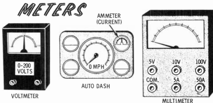
These devices indicate an approximate measurement of charges. Yet, these measurements are sufficiently accurate to serve as standards on which electrical and electronics personnel base their evaluations.
