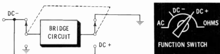
allows the input voltage to be switched to the grid of the proper tube in the circuit. The same direction of current flow through the meter can thus be maintained regardless of the polarity of the input voltage.
