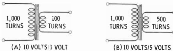
Parts A and B both have 1,000 primary turns each. (This is an example only—a transformer might have many more.) The secondary winding of the transformer in Part A has 100 turns. The turns ratio is therefore 1000/100, or 10/1. If ten volts were placed across the primary, the turns ratio would produce 1 volt in the secondary. If 20 volts were applied to the primary (providing the wire could handle the increased current), the output would be 2 volts, etc.
