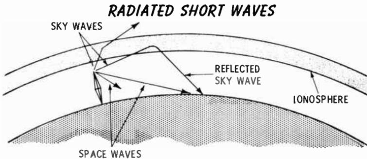
High frequencies radiate a space wave and a sky wave. Both of these waves travel essentially in straight lines. To receive a space wave, the receiving antenna must be within line-of-sight of the transmitting antenna. If the receiving antenna is beyond the horizon, the space wave (if it still retains sufficient power) passes over it.
