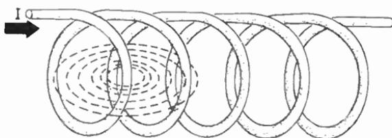
Reactance is directly related to frequency. The amount of reactance in a coil is determined by the frequency of the current and by the number of turns of wire in the coil. The greater the number of times the magnetic field changes direction in a second, the more times adjacent turns will be cut, and the greater will be the opposing current.
