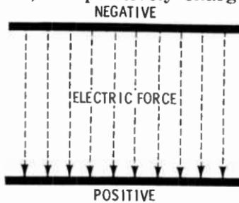
would be moved upward (positive to negative). Like charges repel, and unlike charges attract. Do you recall how an electrostatic field is formed?
