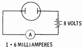
The resistance of the 4-volt circuit is 2,000 ohms. The resistance of the 8-volt circuit is 1,333 ohms. It can be seen that as the voltage between the plates increases, the resistance between the plates decreases.
