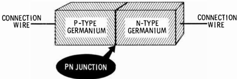
occurring at the junction of the materials is responsible for the unidirectional property of the diode. The contacting surface is called the **PN junction**.
