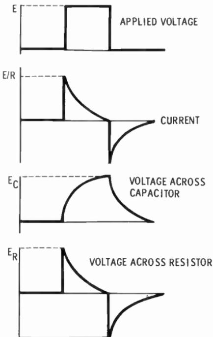
The voltage across the capacitor will start at zero and will build up smoothly until it equals source voltage  $E$ . The voltage across the resistor will, at any instant, equal the difference between the source voltage and the voltage across the capacitor; it will also be a spike as shown.
