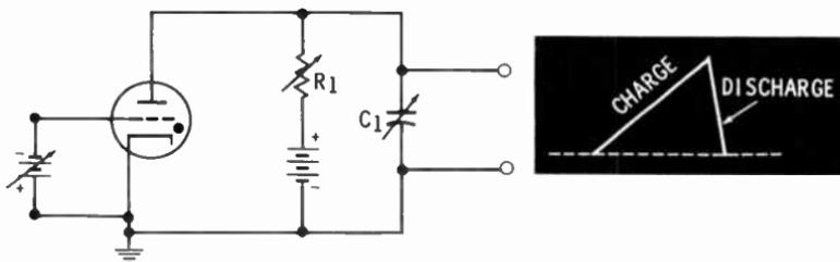
A thyratron is a triode containing an ionizing gas. B+ current flows through  $R_1$  and charges  $C_1$ . When the voltage across  $C_1$  reaches a certain potential, the gas ionizes.
