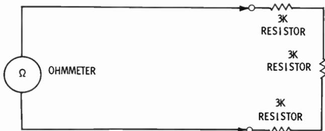
**A46.** Current =  $\frac{\text{voltage applied}}{\text{total resistance}} = \frac{15}{9,000}$
