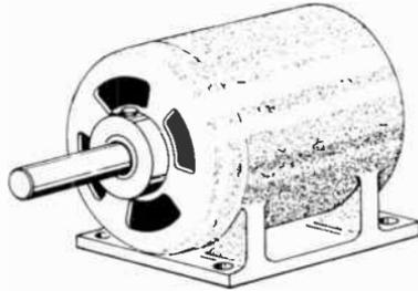
The magnetic forces in a motor attract and repel each other. This causes the **armature** (rotating part of the motor) to turn.
