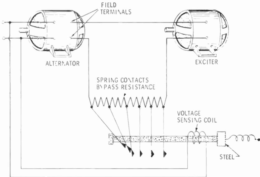
the resistance between the exciter and the alternator increases. This causes less field current to flow to the alternator, and the output voltage decreases to normal. If the voltage falls, the spring is able to pull the steel piece away from the coil. This closes more of the contacts. The resistance then decreases and the field current and output voltage increase. The resistance could also be placed in the exciter shunt-field circuit.
