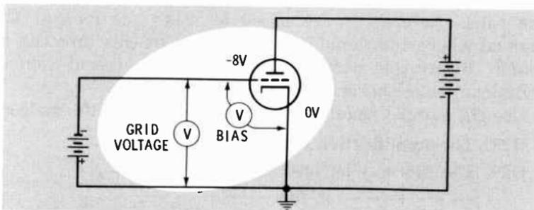
The bias on the tube above is equal to the difference between the grid voltage ( $-8$  volts in the figure) and the cathode voltage ( $0$  volts in the figure). Therefore the bias in this case is equal to  $-8$  volts.
