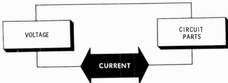
Voltage, as you know, is an electrical pressure that causes current to flow under proper conditions. Current flows if there is a closed loop (complete path) from one side of the voltage source through the circuit components to the other side. The amount and type of voltage to be applied and how much current will flow is dependent on the type and value of components used in the circuit. As an example, you have seen circuits similar to those shown in the schematic diagrams below.
