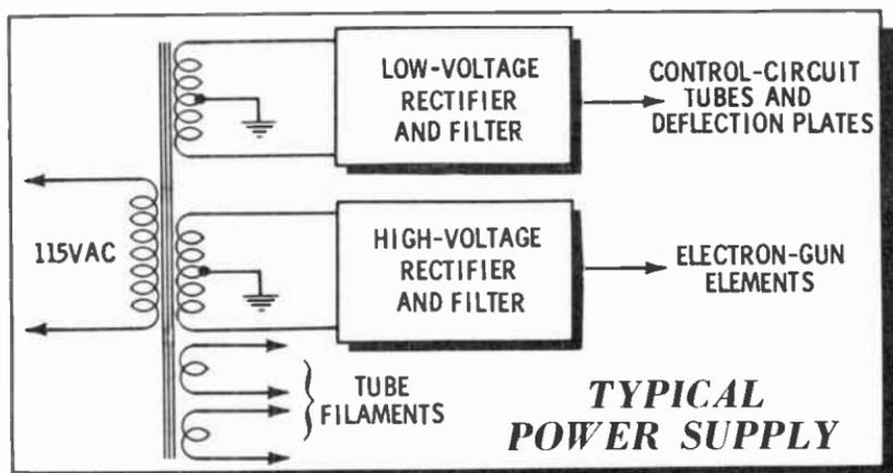
Most test scopes have both high-voltage and low-voltage power-supply sections fed by a single transformer. The high-voltage, low-current section takes care of the electron-gun requirements. Voltage needs for the remainder of the circuits are supplied by the low-voltage section. This section may provide potentials as high as 300 or 400V. A third or fourth winding on the transformer provides voltage and current for the vacuum-tube heaters.
