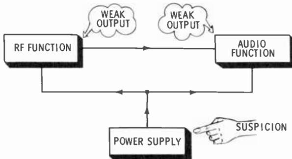
The new Step-2 conclusion places the probable location of the trouble in the power-supply function. A Step-3 check of the schematic for the receiver indicates that there should be a pulsating DC output of 90V. With a VTVM or multimeter, the DC reading shows less than half this value. The faulty function has been confirmed.
