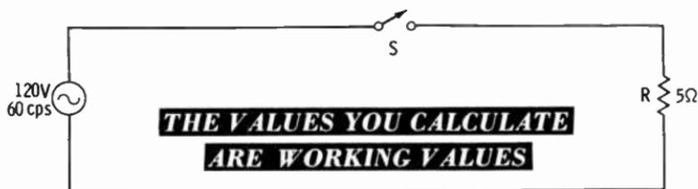
From Ohm's law we find that the current in the above circuit will be  $I = \frac{120}{5} = 24$  amperes. But, since this is an AC circuit, we also know that both the 120 volts and the 24 amperes are rms values; that is, they are the working values. Since AC voltage and currents appear as sine waves, the voltage actually varies. The current also varies, but its numerical value is always five times smaller than that of the voltage.
