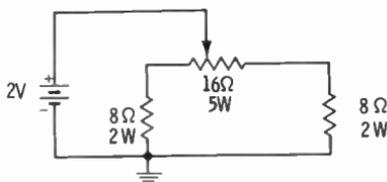
If the wiper of the potentiometer is centered, the resistance from either side to ground will be equal.
