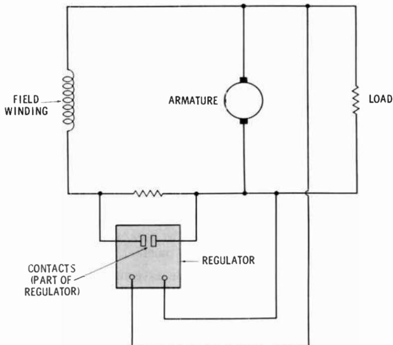
More complicated arrangements are sometimes used to regulate the voltage of shunt generators. However, they all operate by controlling the amount of current flow in the shunt field winding.
