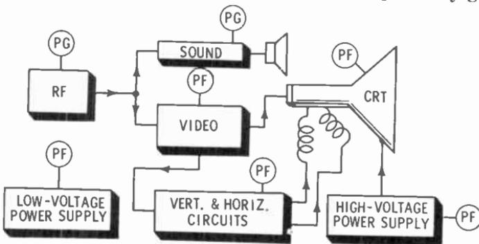
Five functions are suspected as being probably faulty. In which order should they be tested to arrive at a Step-3 conclusion (exposure of the single faulty function)?
