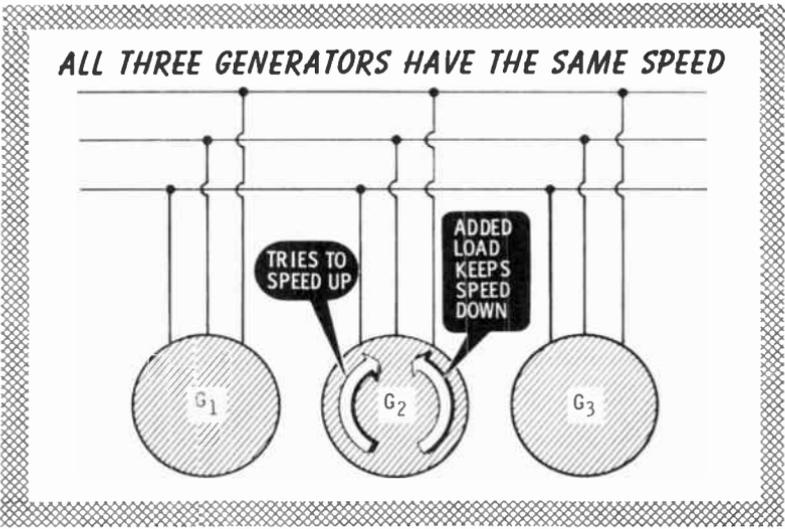
For instance, say that  $G_2$  in the figure above tries to speed up. Additional load is immediately placed on this generator. This tends to hold the speed down. This action keeps all of the generators operating at the same speed.
