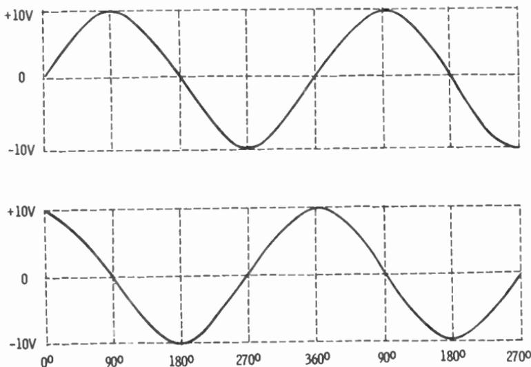
The top waveform (sine wave) rises from zero to 10 volts positive in  $90^\circ$  (one-quarter cycle). During the same time period the bottom sine wave decreases from 10 volts to zero. In other words, the two are  $90^\circ$  out of phase.
