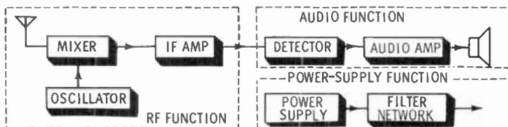
In smaller equipment such as the radio receiver illustrated above, the number of circuit-group functions may be limited. Further limitations are imposed by the receiver, which has only two controls—tuning and volume. However, the antenna, mixer, oscillator, and IF amplifiers of the set shown can be grouped within a radio-frequency function. The combination of detector, audio amplifier, and speaker is desig-
