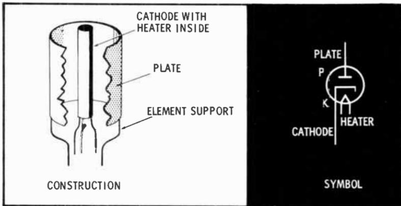
**Cathode Temperature**—The number of electrons that form in a cloud around the cathode depends on the cathode temperature. The temperature of the cathode is controlled by the heat generated by the filament. There is an upper limit, however, beyond which a further increase in temperature will not cause an increase in electron emission. This is called **cathode-temperature saturation**.
