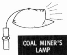
Other applications for a thermocouple are in low-power devices such as small transistor radios and carbide lamps used by miners and hunters. A mixture of carbide and water produces a gas that will burn. The flame from a carbide burner heats the junctions of several thermocouples. The cooler ends are connected in series and produce a voltage which is then used to light an electric lamp.
