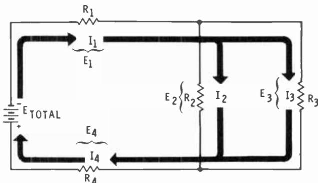
If you are solving for **total current**, you must use only the values that truly represent **total voltage** and **total resistance**. You cannot use  $E_1$  (voltage across  $R_1$ ) because it is not the total voltage. You cannot use the equivalent parallel resistance because it is not the total circuit resistance.
