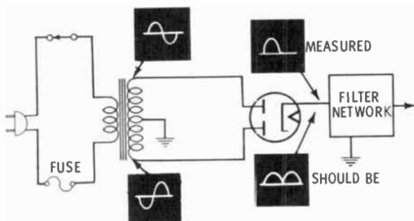
Shown above is a faulty full-wave rectifier circuit with measured input and output waveforms. The proper output waveform is also included. Half of the output cycle is missing. A study of the schematic diagram and the waveforms reveal that you should concentrate your search in the lower plate section of the diode.
