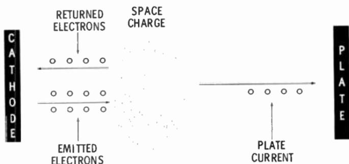
(plate current). The remaining or surplus electrons not required by the plate are returned to the cathode. The quantity returned is the difference between the amount of electrons originally emitted by the cathode and the amount going to make up the plate current. The result of all this is that the space charge is maintained at a constant size. In other words, it reaches and stays in a state of equilibrium.
