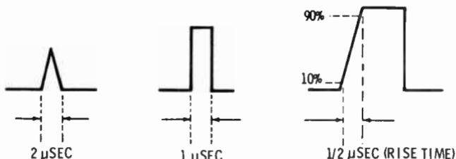
Another way to examine the response of a scope is in terms of **rise time**. The rise time is the time between the 10% and 90% amplitude points on the leading edge of a pulse. The minimum rise time that a scope can reproduce is determined mainly by the charge time of certain capacitances in the scope.
