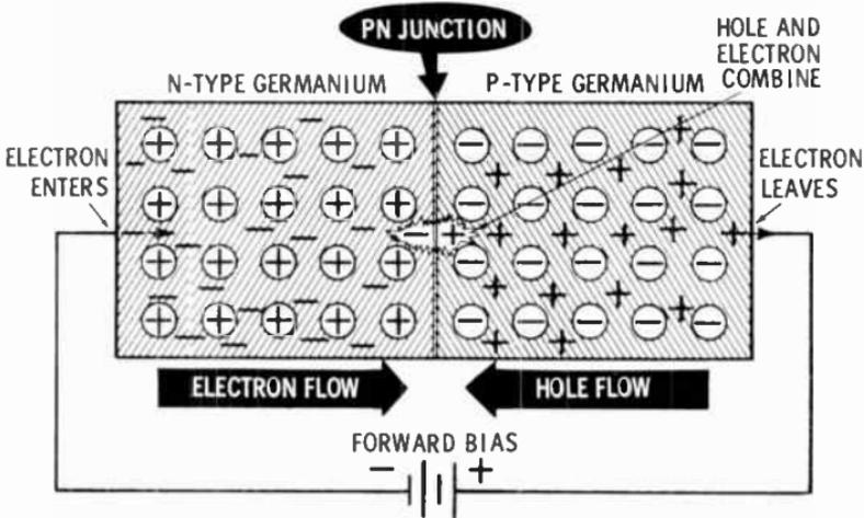
comes negative when a hole combines with an electron at the barrier. Thus, it gives up an electron to the positive battery terminal. A solid-state diode symbol is shown below.
