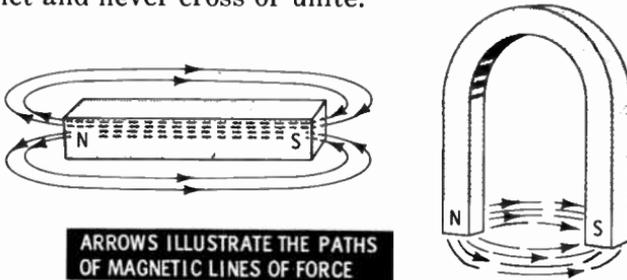
The lines formed by the magnetic loops are called **magnetic lines of force**. The area occupied by these lines is called the **magnetic field**. The magnetic field is the induced energy surrounding the magnet or the space through which the influence of these magnetic lines of force can be measured. The strength of the magnetic field is measured by determining the number of magnetic lines of force per unit area surrounding the magnet.
