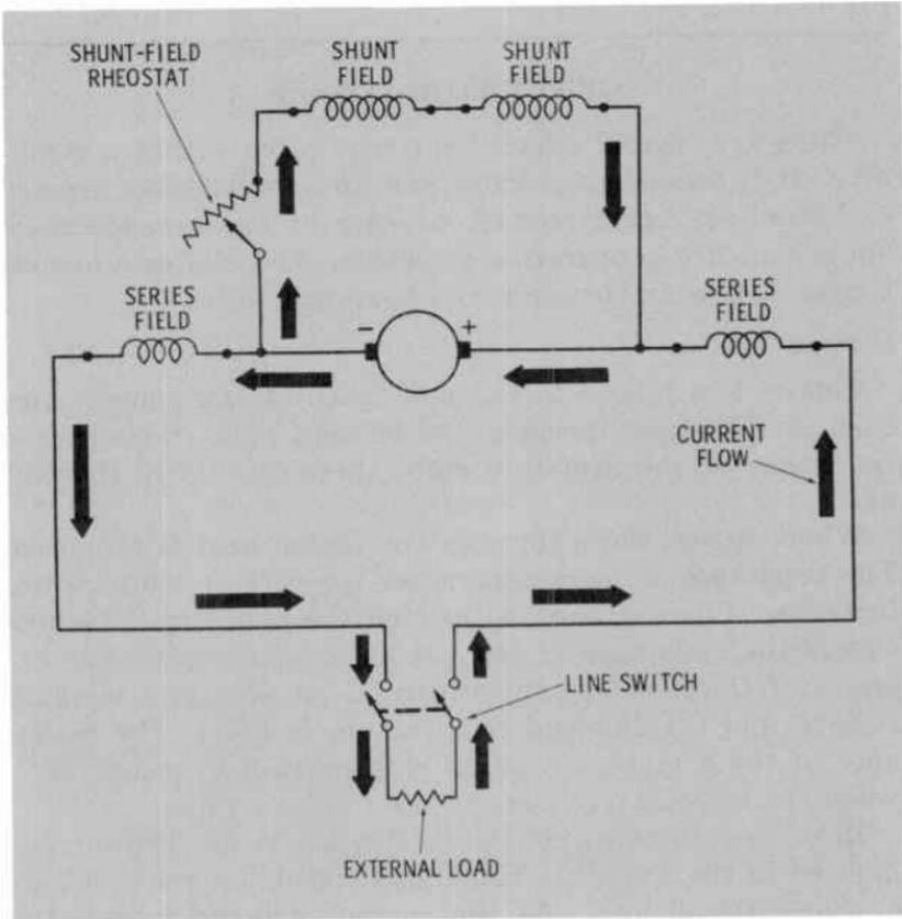
There is no difference between the short- and long-shunt compound generators as far as the operation and output are concerned. The only difference is in the point where the series field is connected.
