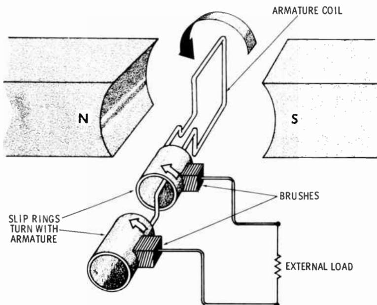
the armature coils, the ends of the coils are connected to **slip rings** which rotate with the armature. Stationary con-
