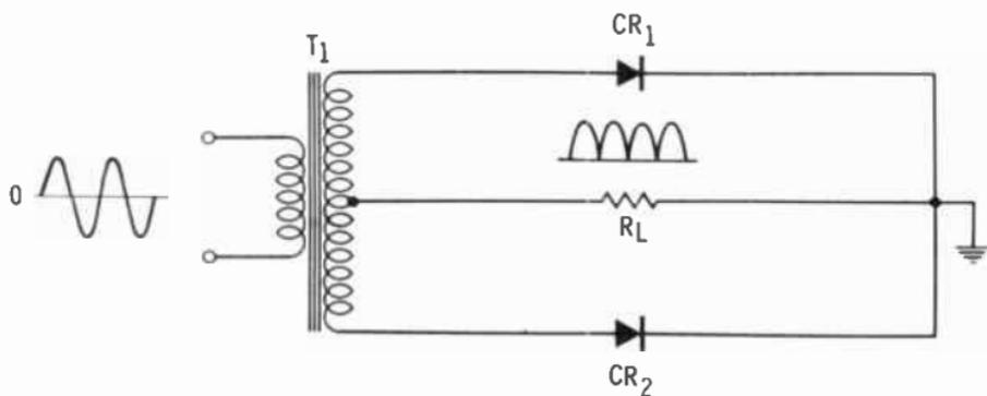
Q14. A full-wave rectifier uses a transformer with a ----- secondary.
