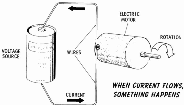
Current flows through the wires of an electrical or electronic device in much the same way water flows through pipes.
