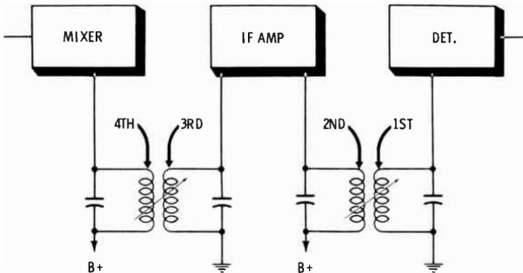
During this and all following alignment steps, keep the gain of the signal generator no higher than necessary to give an indication on the output indicator used. If the gain is too high, receiver stages will overload or saturate, and output readings will be invalid. Readjust all coils until you are sure they have been peaked to maximum.
