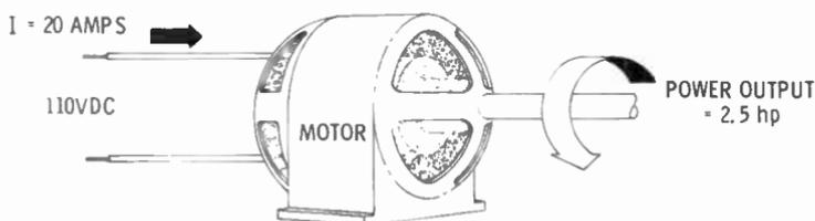
To find the efficiency of the motor above, you must calculate the power input (in watts) and power output (in watts), and then use the formula to find efficiency.
