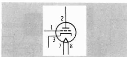
In nearly all examples the elements of a tube are marked with their pin numbers, as shown above. Transistor leads are identified by the elements shown in the schematic. A notation on the diagram identifies the type of instrument used in making the measurements. For example, **DC voltage measurements are taken with a 20,000-ohms-per-volt meter, and AC voltages with a 1,000-ohms-per-volt meter.**
