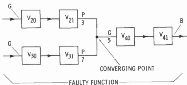
The diagram above shows the test results of Step 3. Inputs to both channels of the function are good, but the single output is bad. The decision of where to make the first Step-4 test depends on the nature of the bad output.
