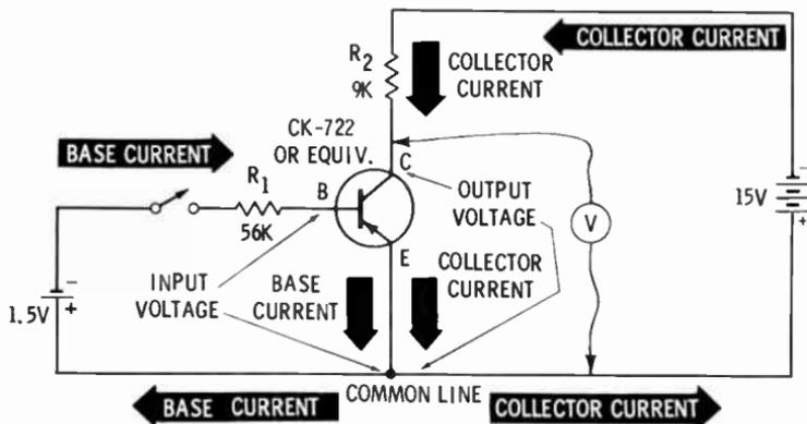
The input to this amplifier is maintained at 1.5 volts by the dry cell shown. An AC signal applied to the base will rise above and below this reference voltage.
