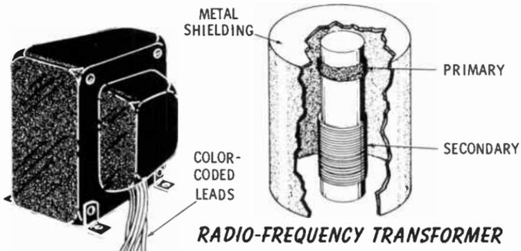
Most transformers are designed to transfer power. Others, however, are built to transfer only signal voltages.
