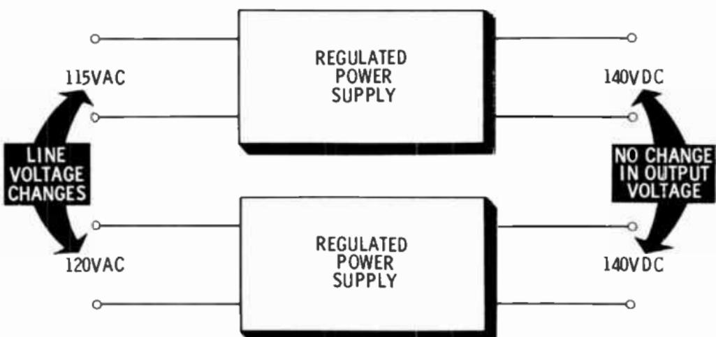
signed to prevent changes under these conditions as well. Notice that many voltage regulators can be manually controlled, incorporating an adjustment used for selecting a particular voltage output.
