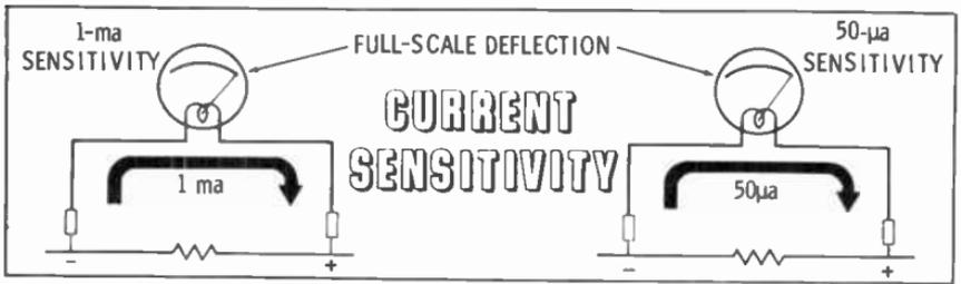
**Ohms-per-Volt Sensitivity**—Ohms-per-volt sensitivity is determined by the total resistance that must be in series in the meter circuit to obtain full-scale deflection when 1 volt is applied. The resistance value can be determined by Ohm's law:
