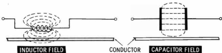
however, is mostly contained within the capacitor. An additional advantage of the capacitor is that it does not pick up stray fields as a coil does.
