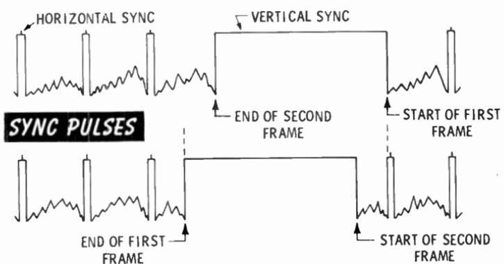
The above illustration shows the comparative widths of the horizontal and vertical sync pulses and the relative starting times of the first and second frames. The sync pulses are removed from the complete video waveform and sent to the sync separator.
