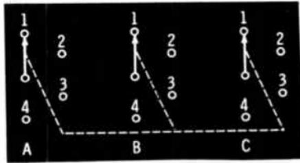
above, the switch has three wafers (A, B, and C). Again, the dashed line represents mechanical connection whereby all wafers are actuated at the same time. In this case the switch is said to be a **three- (triple) pole, quadruple-throw (four position), or TPQT (triple-pole, quadruple-throw)**.
