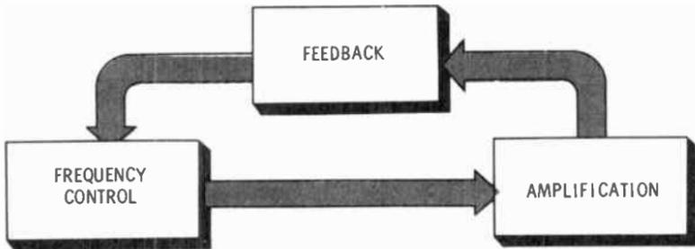
**Amplification**—An amplifier with plate current flowing will normally amplify any spurious signals appearing at the grid. A spurious signal is any unwanted signal generated either in the equipment itself or externally.
