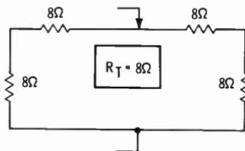
The total current will equal:  $2\text{V}/8\Omega = 0.25 \text{ amp}$
