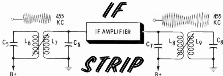
converter will be allowed to enter the IF strip. **IF strip** is a common term that includes the IF-amplifier tubes and transformers.
