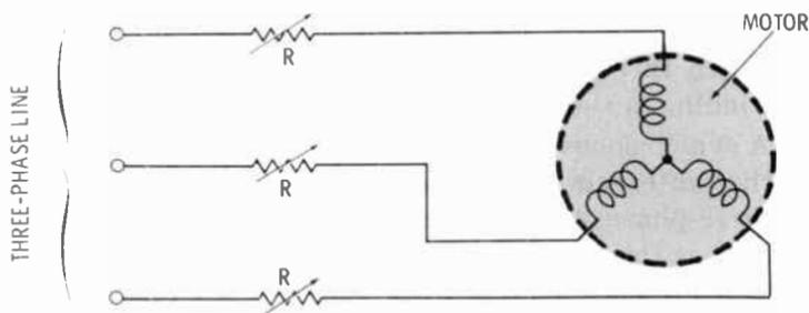
A third method of starting a squirrel-cage motor is to use series coils (reactors). A coil with relatively high inductive reactance is inserted in series with each of the motor coils as shown below. When the motor has picked up speed, the switches are closed to bypass the reactors.
