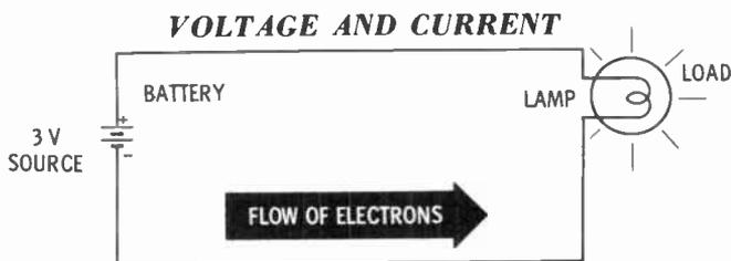
Voltage (electrical pressure) is an excess of negatively charged particles at one terminal of a source with respect to the other terminal.
