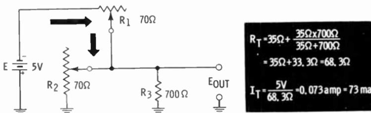
The voltage across  $R_1$  will equal 73 ma times 35 ohms, or 2.555 volts. This leaves 2.445 volts for the output. Dividing 2.445 volts by  $R_3$  equals approximately 3.49 ma.
