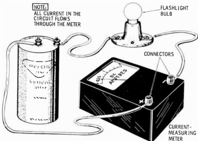
Meters are read by noting to which number (or division mark between numbers) on the scale the needle is pointing.
