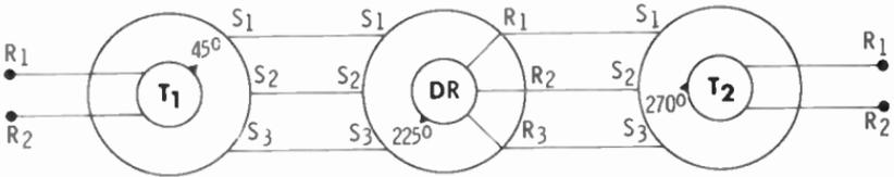
Addition with a differential receiver recording a sum of two angles is accomplished by the following connections.
