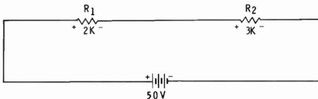
A54. Voltage across  $R_1$  is 20 volts.
