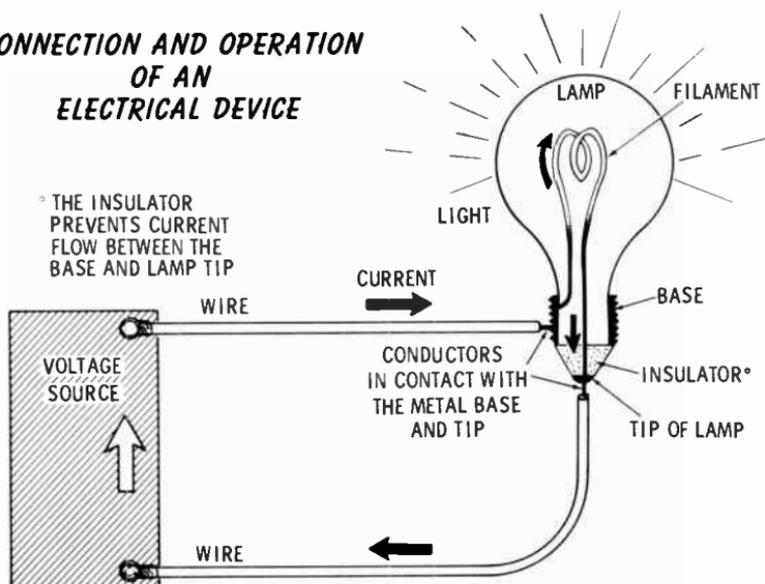
Wires, connectors, and terminals allow current to flow in a circuit because they are made of conducting metals. Care must be taken, however, when joining these parts to each other. Metal at the contact points must be clean and free from the insulating properties of dirt, grease, etc. Sandpaper or a small file can be used to clean these junction points when necessary. After a wire has been stripped, it should be cleaned of any remaining insulation.
