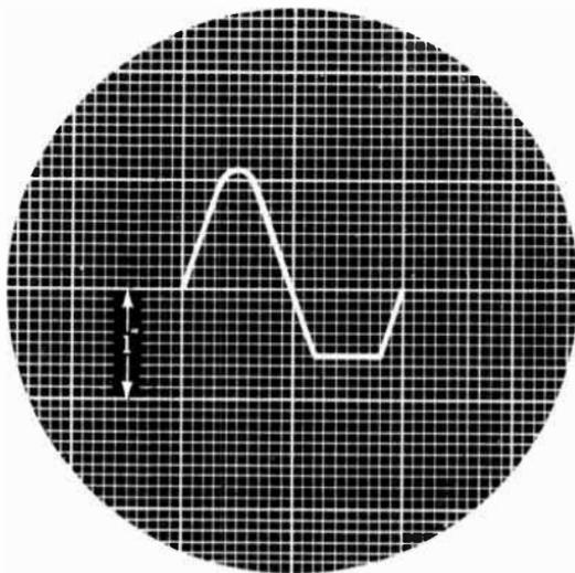
The graticule can be used to determine the voltage of waveforms because the **deflection sensitivity** of a CRT is uniform throughout the vertical plane of the screen. Deflection sensitivity is a constant which is dependent on the construction of the tube. It states the number of inches, centimeters, or millimeters the beam will be deflected for each volt of potential difference applied to the deflection plates. Deflection sensitivity is directly proportional to the
