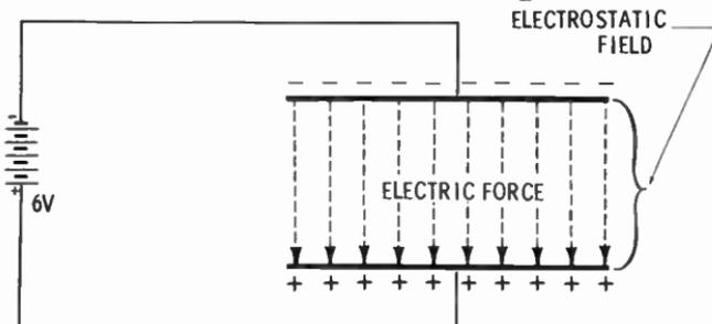
If a 6-volt battery is connected to the plates in the manner shown on the opposite page, the battery will draw electrons from the bottom plate and deposit them on the top plate until the difference in potential between the plates equals the battery voltage. The potential of the plate having an excess of electrons will be negative. The other plate, being deficient in electrons, will be positive.
