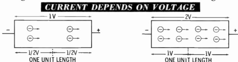
resistance. One volt is distributed (dropped) across each half of the resistance, increasing the current that flows through its section.
