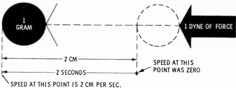
A force of one dyne produces an **acceleration** of 1 centimeter per second per second on a 1-gram mass.
