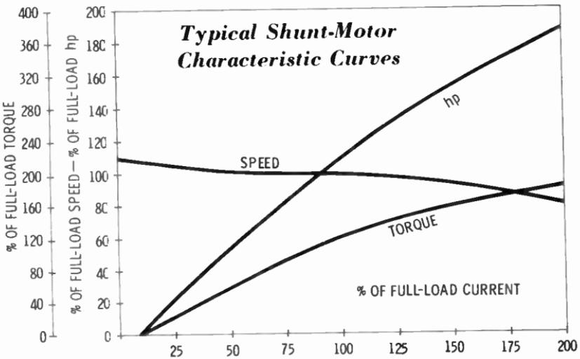
The main characteristics of a shunt motor are its constant speed and low starting torque. This means that DC shunt motors cannot be used for hard-starting loads.
