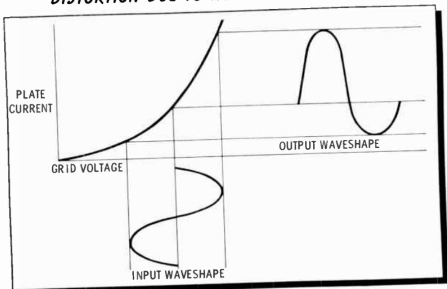
signal are equal, but because of the shape of the curve, the positive and negative halves of the output are quite unequal.
