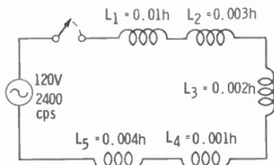
**Q7. How much current will flow in this circuit?**
