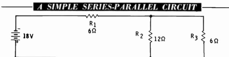
The best way to work with a series-parallel circuit is to reduce all parallel combinations to an equivalent resistance. When this is done, the total current or the total resistance for the resulting series circuit can be readily found.
