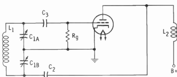
$C_{1A}$ ,  $C_{1B}$ , and  $L_1$  make up the tank circuit. The resonant frequency of the tank is changed by varying  $C_{1A}$  and  $C_{1B}$ . (These capacitors are usually on a common shaft so that both of them can be adjusted at the same time.) The output of the amplifier is introduced into the tank circuit through capacitors  $C_2$  and  $C_{1B}$ . The tank-circuit voltage is introduced into the grid of the amplifier by the coupling network consisting of  $C_3$  and  $R_g$ .
