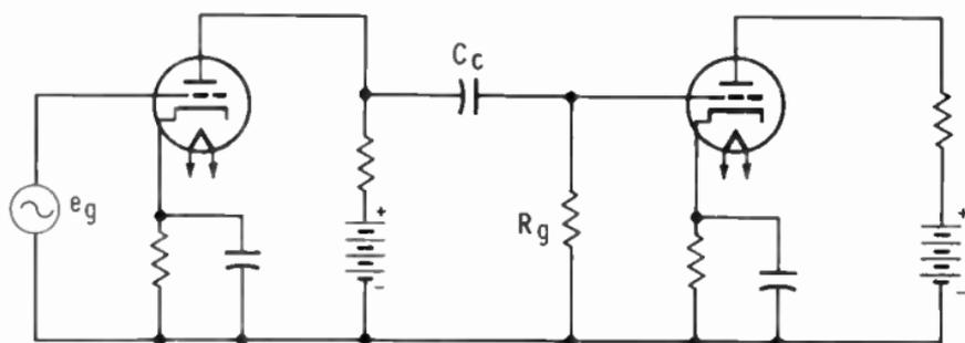
Resistor  $R_g$  is called the **grid-leak resistor**. This resistor serves to keep the grid at ground potential, thus preserving the voltage difference between the grid and cathode. This resistor actually serves a dual purpose, also being used as the component across which the signal voltage from the preceding stage is developed.
