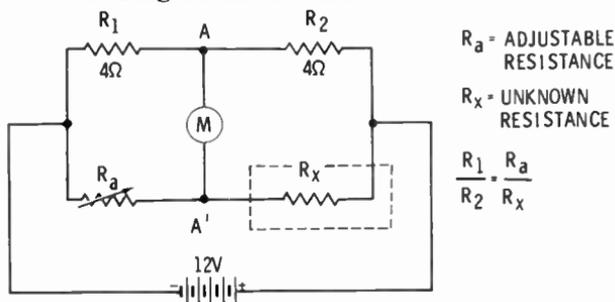
When the resistance ratios in the legs are not equal, there will be a voltage difference between A and A'. Current will flow through the meter. When  $R_a$  is adjusted to register zero current,  $R_1/R_2 = R_a/R_x$ . If there were a means provided to show the value of  $R_a$  at this setting, how could you determine the value of  $R_x$ ?
