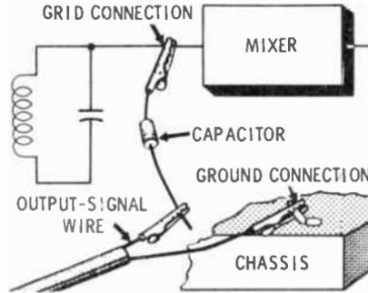
There is a choice of output indicators available. Whichever you choose, adjustments are made for maximum output indication and not for a precise numerical reading.
