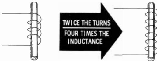
The diameter also affects the inductance of a coil. The larger the diameter, the more inductance it will have.
