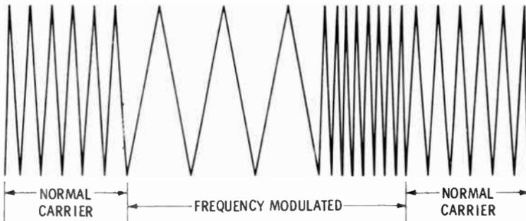
Notice in the diagram above that the frequency of the FM carrier varies, but its amplitude remains the same. Study the following diagrams.
