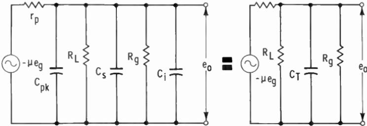
In the high-frequency range, three unwanted capacitances become important. They are the plate-cathode capacitance ( $C_{pk}$ ), the stray capacitance of the wiring ( $C_s$ ), and the capacitance of the input circuit of the second stage ( $C_i$ ). Since the equivalent circuit is a parallel one, all three capacitances may be combined into a total stray capacitance ( $C_T$ ).
