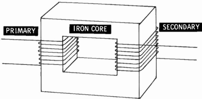
An iron core is used to increase the magnetic flux and to channel it to the secondary coil. The primary coil sets up a magnetic field in the core, and the secondary coil converts the field back to electric current. Power is actually transferred from the primary to the secondary. A lamp or other load placed in the secondary circuit will operate.
