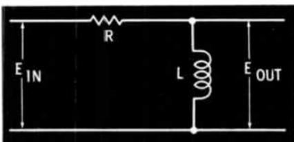
If you have a signal generator, you can build a simple filter circuit like the one shown below and see how it reacts to different frequencies.
