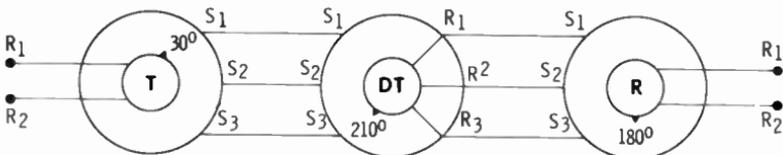
**SUBTRACTION BY A T-DT-R SYNCHRO SYSTEM**
