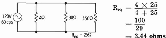
$$\begin{aligned} R_{eq} &= \frac{4 \times 25}{4 + 25} \\ &= \frac{100}{29} \\ &= 3.44 \text{ ohms} \end{aligned}$$
