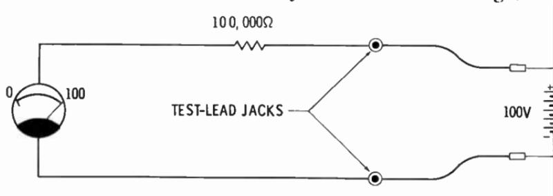
In the diagram above, a 100,000-ohm resistor was selected to give a full-scale meter reading of 100 volts. If the resistor had a tolerance of 20%, the full-scale reading could be off about 20 volts in either direction. A 10% resistor could cause readings between the extremes of about 90 volts and 110 volts. A 5% resistor could result in an error of 5 volts above or below 100 volts. None of these readings would be close enough for most purposes.
