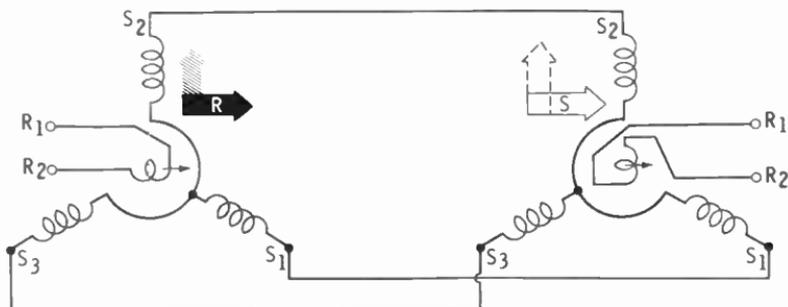
Assume that the T rotor has been turned clockwise from  $0^\circ$  to  $90^\circ$ . The CT stator field will make the same rotation. If the CT rotor remains at  $0^\circ$ , maximum voltage in phase with the AC line voltage can be measured across R<sub>1</sub> and R<sub>2</sub>. If the CT rotor is now turned to  $90^\circ$ , the voltage reading will reduce to zero. In this position the rotor winding is at right angles to the stator field.
