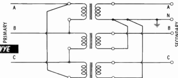
Q23. Name the four ways in which transformers can be connected in a three-phase system.
