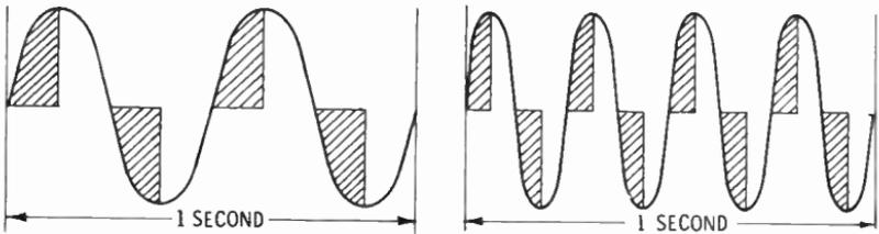
What does this mean? The frequency was doubled, and this doubled the current flowing into the capacitor—yet, the input voltage remained the same. A pure capacitance lets twice as much current flow if the frequency is doubled.
