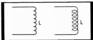
The unit of inductance is the **henry**. A coil is said to have an inductance of 1 henry if the current through it, changing at a rate of 1 ampere per second, encounters an opposition, or counter voltage, of 1 volt. This means that the **opposition to current change** shows up as a voltage opposing the applied voltage.
