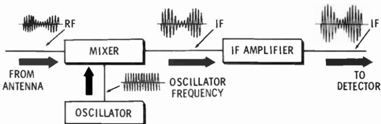
**The Mixer**—The carrier and oscillator frequencies combine in the mixer tube and four different frequencies appear at the output. One of these four is the **difference** between the oscillator and the carrier frequencies, and is usually 456 kilocycles. The other three are rejected by the next stage.
