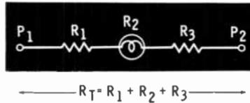
The lamp shown above does have a resistance, even though it is not a resistor. Therefore it is marked as  $R_2$  for calculation purposes.
