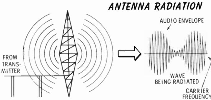
Power is fed to the antenna in the form of both current and voltage. Voltage sets up an electric field along the length of the antenna. Current, in traveling through the antenna (a conductor), sets up a corresponding magnetic field. Both fields vary at the rate of the carrier frequency and at the amplitude and frequency of its audio envelope.
