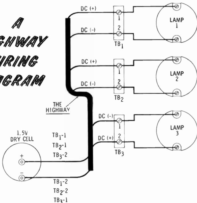
TB1 is the abbreviation for terminal board 1. TB2-1 (terminal 1 of terminal board 2) is positive and therefore connected to the positive pole of the cell. Although only two wires are shown connected to the cell, there are actually three at each pole as indicated by the TB listings.
