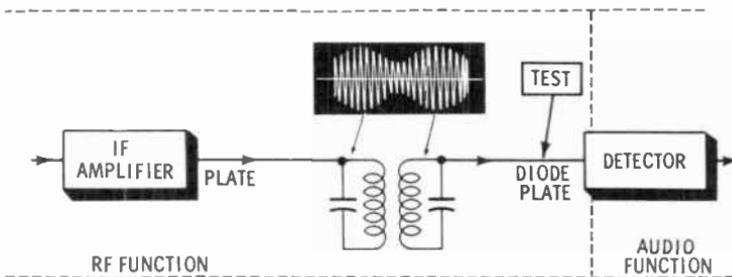
From the schematic diagram of the receiver, locate the pin number of the upper diode plate of the detector. Connect the oscilloscope to the proper socket terminal and rotate the tuning control. If no audio-modulated signal is noted at several station settings, the RF function is not operating properly.
