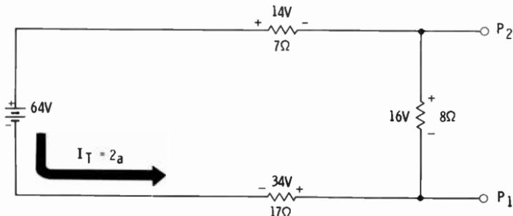
of its resistance. That is, the 17-ohm resistor in the above circuit will have 34V (2 amps times 17  $\Omega$ ) developed across it. The other voltages are determined similarly. Thus the voltage between  $P_1$  and  $P_2$  is 16V.
