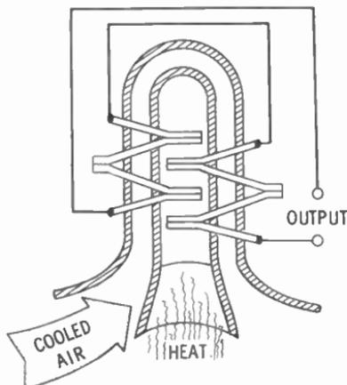
How can you make a thermocouple? One way is to twist the ends of an iron and a copper wire together. Heat the twisted junction over a flame. If the free ends are connected to a milliammeter, a small current reading may be observed.
