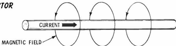
A good way to remember the direction of the induced magnetic field is the **left-hand rule**. With your left hand grasping the wire and your thumb pointing in the direction of the current, the curved fingers of your hand indicate the direction of the field. The direction of the magnetic field is always the direction toward the north-seeking pole of the magnet.
