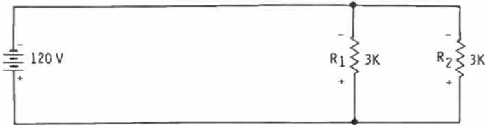
To find the current through  $R_1$ , divide the voltage across the resistor by the value of  $R_1$ . The result of this calculation is 0.04 amp. Since both resistances are equal and have the same voltage source, the current through  $R_2$  must also be 0.04 amp. Both currents are supplied by the same voltage source, so the total current drawn must be 0.08 amp.
