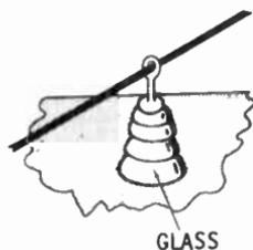
Any insulator, however, will become a conductor of electric current if subjected to a sufficiently high voltage. This is true because of the atomic structure of all elements. The insulators in the following list will remain insulators under normal values of house voltage (120 volts).
