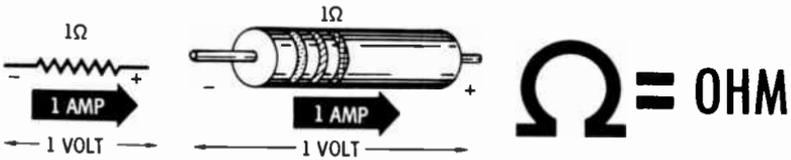
The symbol for the ohm is the Greek letter, **omega**. The uppercase omega ( $\Omega$ ) is used to represent ohm. The amount of resistance in a circuit is designated by a number of ohms.
