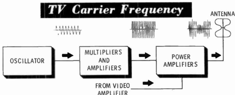
For VHF (very high frequency—channels 2 to 13), the frequency of the carrier is between 54 and 216 megacycles. For UHF (ultra high frequency—channels 14 to 83), the carrier is between 470 and 890 megacycles. Transmission of signals at these frequencies is quite different from that for the lower radio frequencies. High frequencies have short wavelengths. A **wavelength** is the time duration, or length, of one cycle. The higher the frequency of a signal, the shorter is its wavelength.
