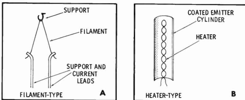
Part A shows a filament-cathode. The single wire serves as both the filament and cathode; it is made of a material (normally coated or uncoated tungsten) that emits electrons when hot.
