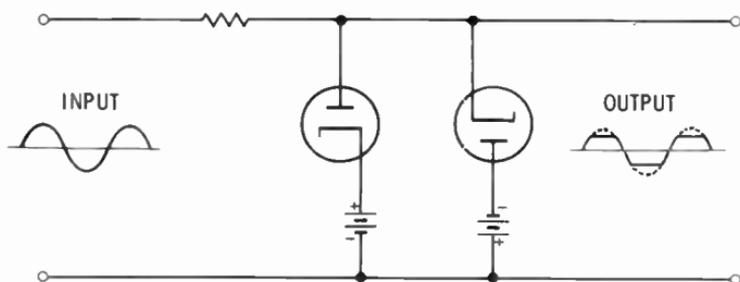
**Q30. How could the limiter circuit at the top of this page be used for negative limiting?**
