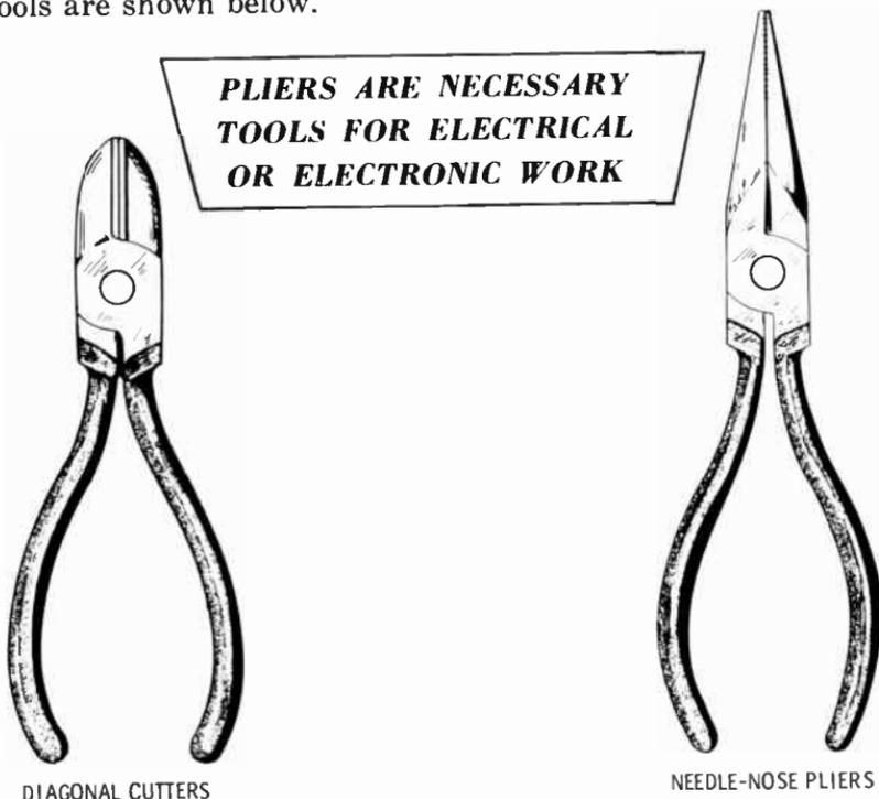
**Diagonal Cutters**—Diagonal cutters, also called “dikes,” are used for cutting wire, trimming leads and terminals to length, and stripping insulation from wire.
