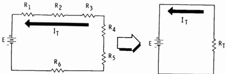
$$R_T = R_1 + R_2 + R_3 + R_4 + R_5 + R_6$$
