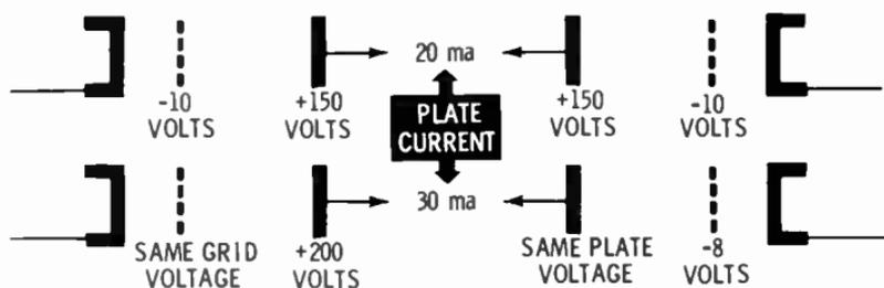
The constant use of the terms plate voltage, grid voltage, and filament voltage has led to the use of some simple shorthand notations, as shown in the figure below.
