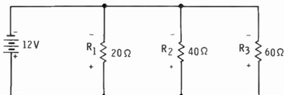
A60. I in R<sub>1</sub> = 0.6 amp. I in R<sub>2</sub> = 0.3 amp. I in R<sub>3</sub> equals 0.2 amp. Total I = 1.1 amps.
