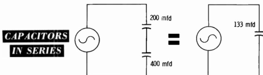
**Q1. What is the equivalent capacitance of the following circuit?**
