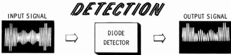
In the figure above, the diode is used as a **detector**. A typical TV picture signal is shown. It is passed through a diode detector which selects only the positive half of the signal.
