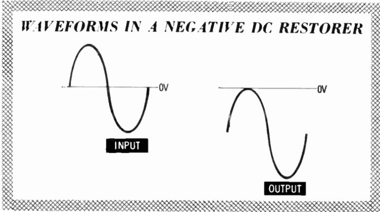
In this way the entire waveform has been shifted below the zero level to clamp the top of the waveform to zero volts. This circuit is known as a **negative DC restorer**. A **positive DC restorer** can be obtained by reversing the diode. In this
