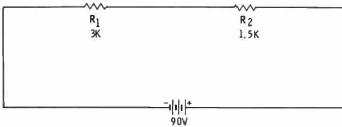
$R_1$  is twice the value of  $R_2$  in the above circuit. Both are in series across 90 volts. How do you find the voltage drop across each resistor?
