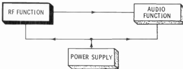
The only purpose of Step 3 is to locate the single function that is causing the equipment to operate improperly. In the example above, either a scope or a VTVM can be used.
