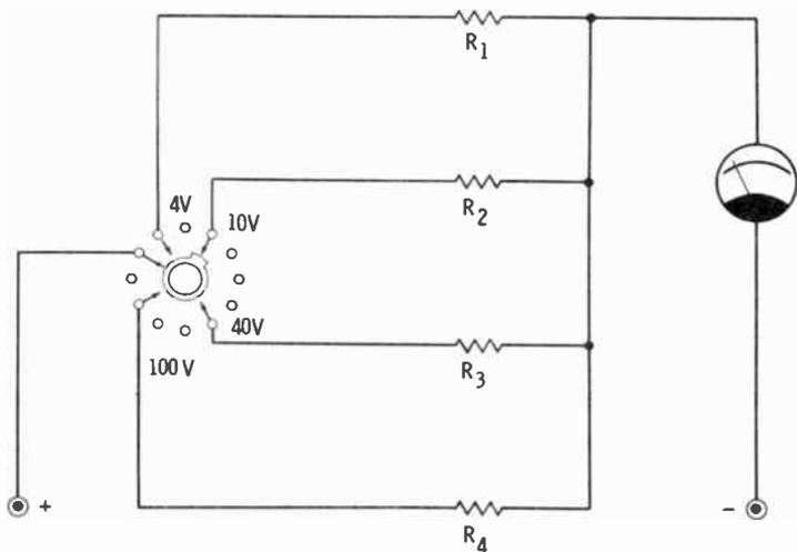
A multimeter may have only a single rotary switch with enough wafers to select both the function (ohmmeter, milliammeter, DC voltmeter, or AC voltmeter) and the appropriate range for each function. In a multimeter having two rotary switches, one switch usually selects the meter function, and the other selects the range.
