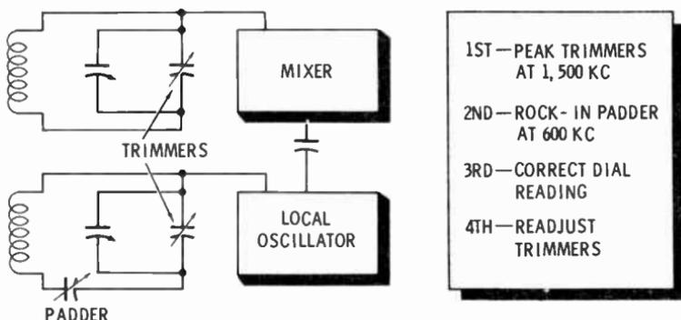
Now, set the generator and receiver dials to 600 kc. **Rock-in** the padder tuning by making the same adjustment at several settings on either side of the 600-kc dial reading. The setting at which the highest output reading is noted is the true 600-kc position. Adjust the receiver dial pointer to indicate 600 kc. Recheck the trimmers for maximum output again, first at 1,500 kc and then at 600 kc. If no change is evident, tuning is completed.
