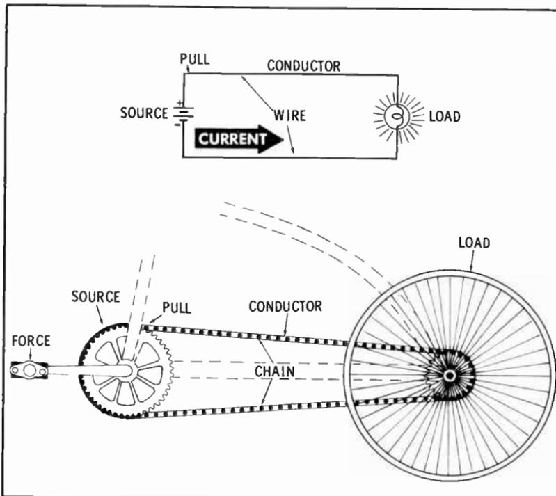
An electrical/electronic circuit must form a complete loop from the voltage source to the load and back to the source.
