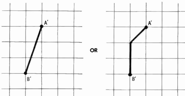
If the amount of deflection (in A29 above) to the left and down occurred so that each set of plates acted at the same time, the picture would be like the one on the left above. For example, if the vertical plates moved the beam downward at the rate of 1 unit per second and the horizontal plates moved it to the left at the rate of  $\frac{1}{3}$  unit per second, both movements would have been completed in 3 seconds at point B'. The result would be a straight line.
