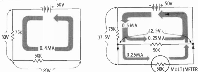
*A Multimeter Loads a Circuit*
