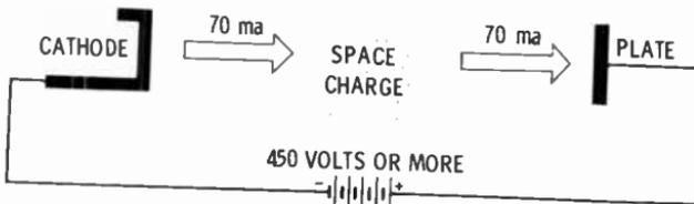
Any further increase in the plate voltage will result in reducing the space charge. Then the voltage on the plate acts directly on the cathode and forces the cathode to emit more electrons than it is designed to emit. This results in rapid destruction of the emitting material and reduced life of the tube.
