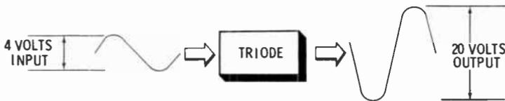
$$\text{AMPLIFICATION} = \frac{\text{OUTPUT}}{\text{INPUT}} = \frac{20 \text{ VOLTS}}{4 \text{ VOLTS}} = 5$$
