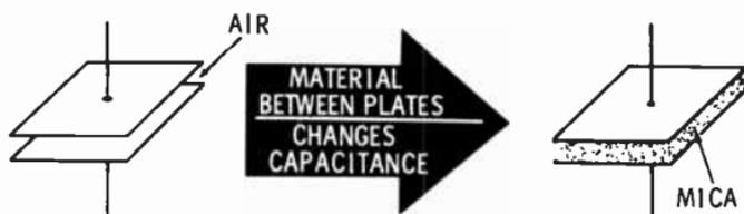
Dielectrics such as mica, glass, oil, and Mylar are a few of the materials that can sustain a high electric stress without breaking down. This property is called **dielectric constant**. The higher the dielectric constant is, the better the dielectric. Air has a dielectric constant of 1, glass about 5, and mica 2.5 to 6.6.
