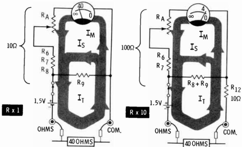
$R_s$  is in the meter branch for  $R \times 1$  and in the shunt branch for  $R \times 10$ . The ratio of meter-branch to shunt-branch resistance for  $R \times 10$  is smaller than for  $R \times 1$ . This means that if  $I_T$  were equal in both parallel networks,  $I_M$  for  $R \times 10$  would be larger than  $I_M$  for  $R \times 1$ . Therefore, a larger part of the total current would flow through the meter in the  $R \times 10$  circuit than in the  $R \times 1$  circuit.
