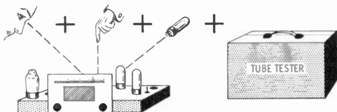
**Q5. Which of the above methods (in addition to a tube tester) can be used to determine whether the heater of a glass vacuum tube is operating?**
