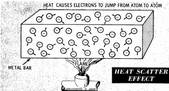
of value, the energy must be applied in such a manner as to move a relatively large number of electrons in the desired direction.
