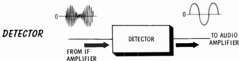
**The Detector**—The purpose of the **detector** is to remove the audio component from the IF waveform. The audio envelope is the same (although reversed) at the top of the waveform as it is at the bottom. The detector circuit is so designed that it accepts only the audio frequency at the top and rejects the IF frequency in the waveform.
