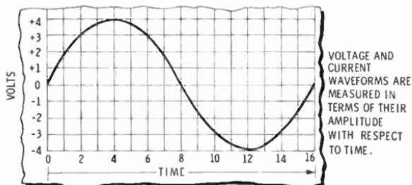
The illustration shows a single cycle of a voltage waveform. The AC sine wave, as this particular waveform is called, is continually changing at the rate indicated by its curvature.
