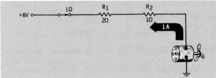
**Q30.** What is the resistance of the motor when the switch is in the MED position?
