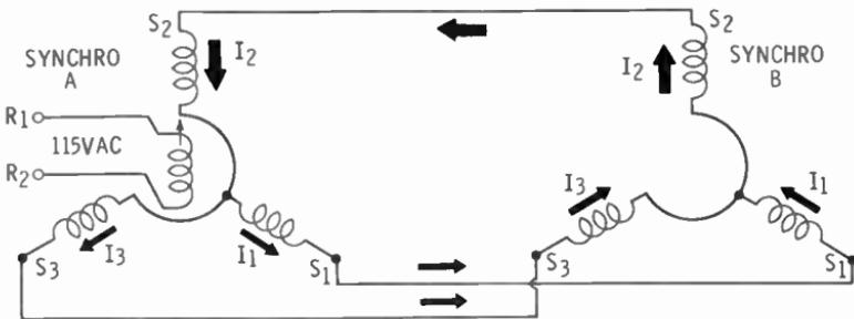
rotor in the left-hand synchro unit, maximum voltage is developed across  $S_2$  and lesser voltages across  $S_1$  and  $S_3$ . The voltages are such that induced current  $I_2$  is equal to the sum of  $I_1$  and  $I_3$  induced in  $S_1$  and  $S_3$ , respectively. Identical currents are flowing through the respective stators of synchro B. As a result, the voltages developed across the synchro-B stator windings are equal to those across the respective windings of synchro A.
