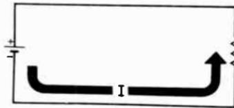
*Electrons Reverse Direction Regularly in an AC Circuit*
