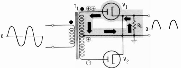
Two diodes are employed in this circuit. A special transformer is used with its center tap connected to one side of  $R_L$  and to ground. When the dot side of  $T_1$  is positive with respect to the center tap,  $V_1$  will conduct. The plate of  $V_2$  is connected to the other end of  $T_1$ , which is negative with respect to the center tap. Thus  $V_2$  will not conduct. The output of the circuit is as shown in the figure. Compare this output with that of the half-wave rectifier.
