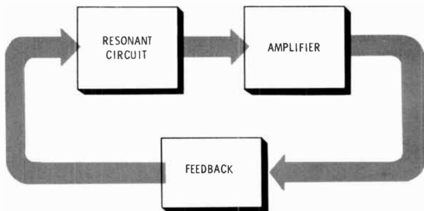
The type of oscillator discussed in this chapter produces an output waveform that is considered to be a sine wave. An oscillator producing such an output is sometimes called a sinusoidal oscillator. You will learn about nonsinusoidal oscillators later in this volume.
