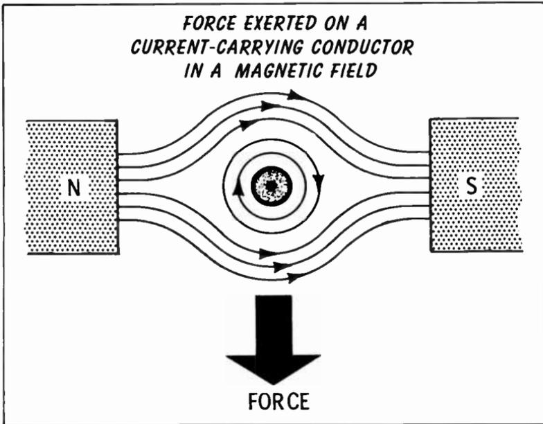
The magnetic field around the conductor in the above figure is clockwise. The current appears to be coming out of the page. The direction of the magnetic field of the permanent magnet is from the north-seeking pole to the south-seeking pole, or from left to right in the figure above. Notice that the lines above the conductor and the lines around the conductor are going in the same direction, reinforcing the field above the electron path. Below the conductor the fields are opposing each other.
