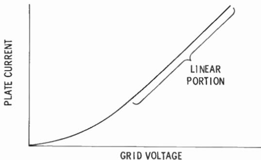
The DC operating point should be located on the **linear portion** of the curve.
