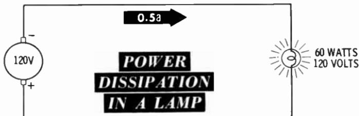
Connected to 120 volts, the 60-watt lamp will draw 0.5 amp. If  $P = IE$ ,  $I$  is equal to  $P$  divided by  $E$ . If the filament has been properly constructed, the lamp will burn for many hours with  $\frac{1}{2}$  ampere flowing through it. What will happen if the lamp is connected across 240 volts? Since the voltage is doubled, current will also double. The power ( $IE$ ) that the lamp must now dissipate is 1 ampere multiplied by 240 volts, which is equal to 240 watts. The filament, con-
