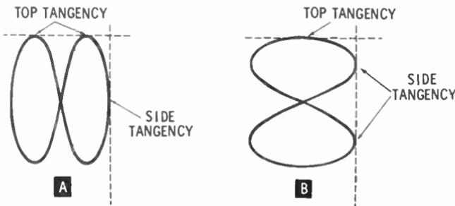
In figure A (above) one cycle of standard frequency appears on the horizontal plates at the same time that two cycles of the unknown are on the vertical plates. There are two points (loops) of top tangency and one point of side tangency. Frequency ratios should be expressed in terms of vertical (unknown) to horizontal (standard). The frequency ratio of figure A is 2/1.
