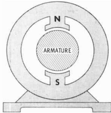
More than one pair of poles are sometimes used in order to produce a stronger magnetic field. When this is done, opposite poles are always next to each other. You can see from the following illustration how this arrangement creates the strongest magnetic field through the armature.
