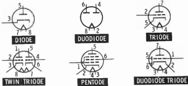
The tubes shown above are just a few of many combinations of tube elements. To conserve space, equipment manufacturers use multipurpose tubes as much as possible. The duodiode, twin triode, and duodiode triode are just three of many examples. A number next to an element indicates the number of the pin to which it is connected. This is normal practice in most schematic diagrams.
