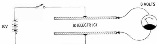
The open switch prevents the battery voltage from being applied across the capacitor. A voltmeter will show a zero voltage between the plates. This is normal, since all matter tends to seek a natural balance when no forces are applied.
