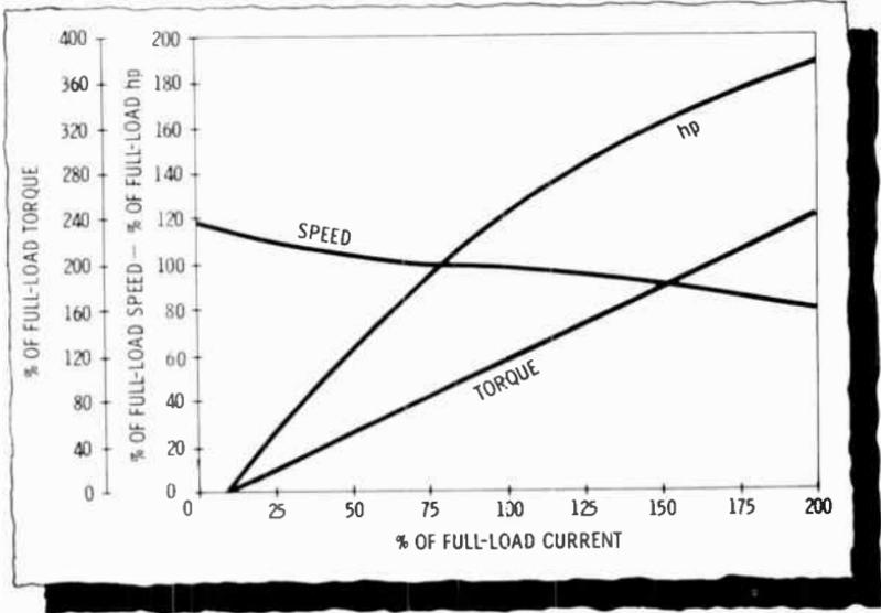
The compound motor has two field windings. For this reason, a compound motor is usually more expensive than either a series or shunt motor of the same capacity.
