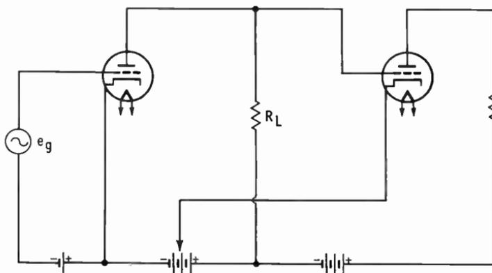
One of the main difficulties encountered with DC amplifiers is **drift**, the gradual change in output voltage without a change in the input. It is, of course, desirable to have no output voltage at all when the input is zero. Drift can be caused by a gradual change in the values of circuit components or even by replacement of a tube.
