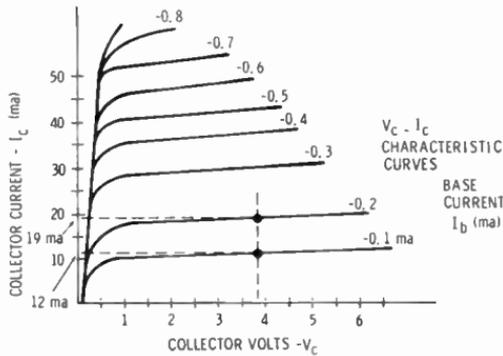
$$\beta = \frac{\Delta I_c}{\Delta I_b} = \frac{19 - 12 \text{ ma}}{0.2 - 0.1 \text{ ma}} = \frac{7 \text{ ma}}{0.1 \text{ ma}} = 70$$
