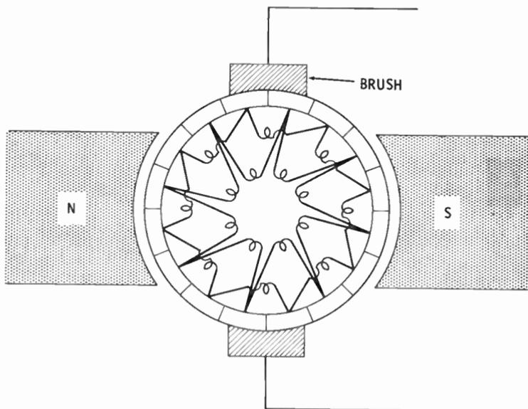
Similarly, a **triplex lap winding** is in effect three separate sets of series-connected coils. In a simplex lap winding, a single brush shorts the two ends of a single coil.
