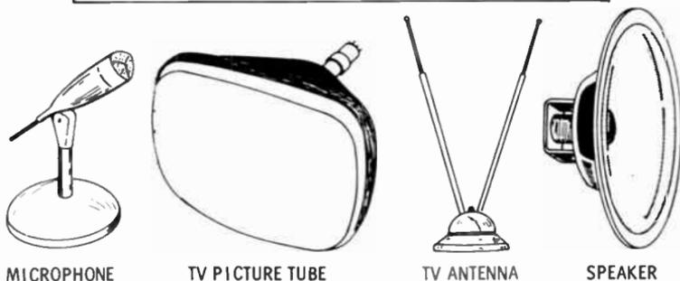
Many complex jobs are performed by combinations of simple devices. That is, two or more simple devices work together to perform a complex job. These devices fall into three categories: (1) input converters, (2) processing devices, and (3) output converters.
