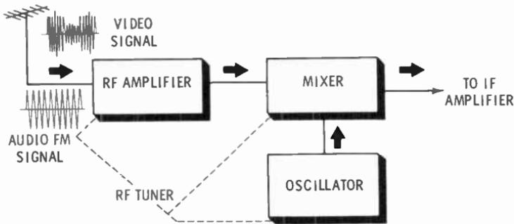
Dashed lines to two or more circuits in a diagram indicate that a single control has an effect on each circuit or part indicated.
