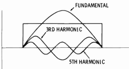
The lowest frequency contained in a train of rectangular pulses is called the fundamental frequency. This frequency has a period equal to that of the square wave. All the other
