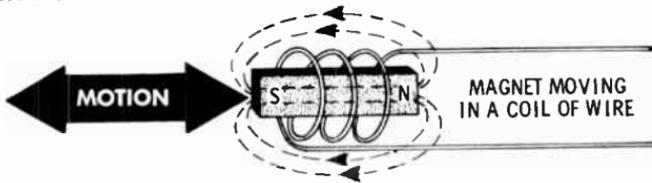
The current reverses direction each time the motion of the magnet changes direction. The amount of current that flows depends on the strength of the magnetic field, the number of turns in the coil, and the speed at which the magnet is moving. Increasing any of these factors increases the amount of current.
