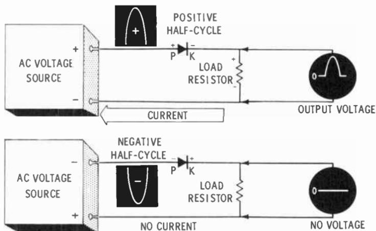
During a positive half cycle, the upper terminal of the source is positive with respect to the lower terminal. This means the lower terminal may be at zero volts, but it is negative when compared to the positive upper terminal. Therefore, the plate of the diode is positive with respect to the cathode. A changing half cycle of current flows.
