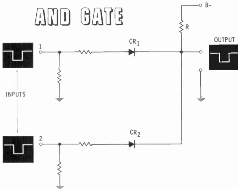
the negative battery terminal for the duration of the input pulses. Therefore, to produce an output, pulse 1 AND pulse 2 must be present. The condition necessary to produce an output from this AND gate is that two negative input pulses must occur at the same time.
