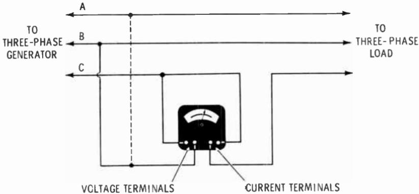
is taken with one voltage lead connected to line B. The lead is then moved to line A, and another reading is taken. The sum of the readings gives the total power. A power factor less than 0.5 produces the same result in the one-wattmeter system as in the two-wattmeter system.
