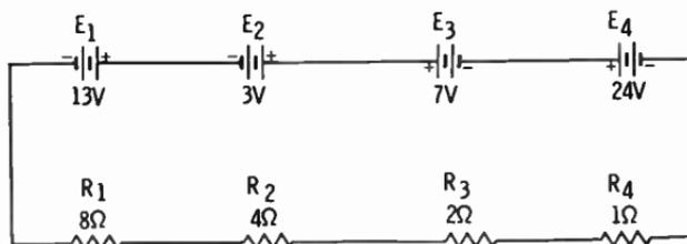
**Q8. In which direction will current flow in the circuit above?**
