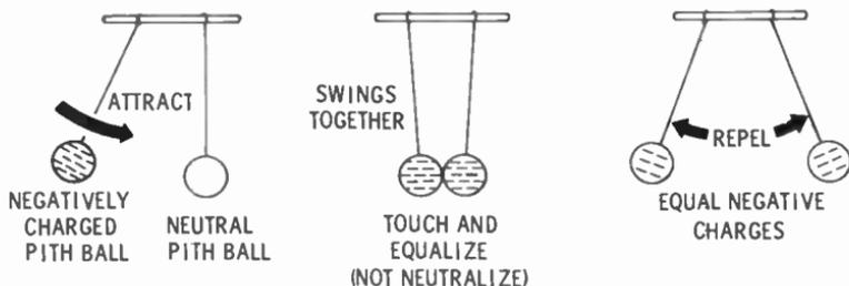
You can perform another experiment using an electroscope to illustrate the principle of attraction and repulsion between static charges.
