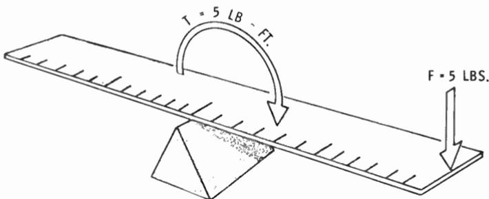
of five pounds is applied to the right end of the ruler, the resulting torque is calculated as follows:
