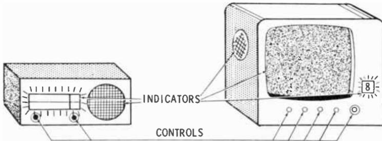
Many radio receivers have two output indicators, a speaker and a light (usually illuminating the dial); the receiver also has at least two controls. The change from desired performance can be registered in many ways—hums, squeals, squawks, low volume, two stations instead of one, or no sound at all. The light is either on or off.
