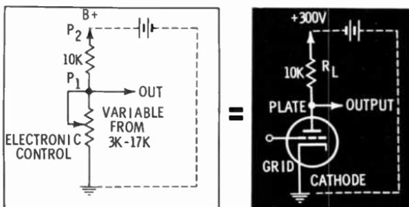
In effect, the grid varies the resistance of the vacuum tube. P<sub>2</sub> is always +300V (to ground). P<sub>1</sub> is a positive
