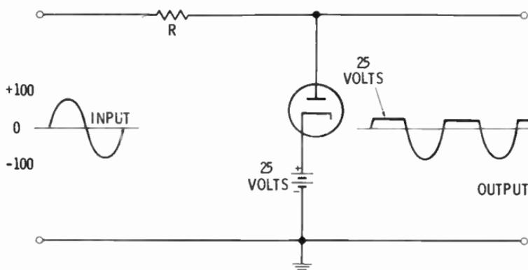
When a pair of diodes is biased so that one is negative and the other positive, both positive and negative limiting are obtained. The output waveform is referred to as a **trapezoidal** waveform.
