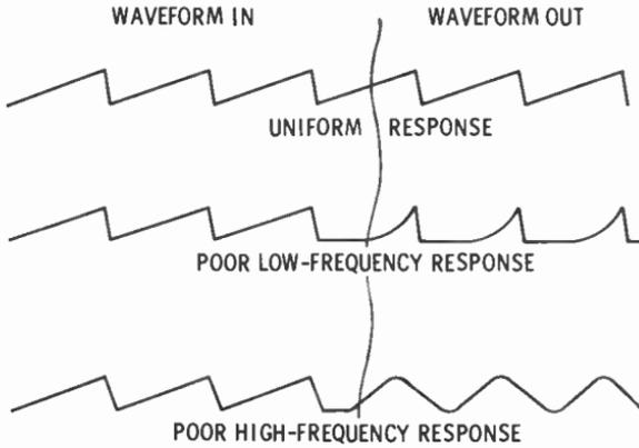
Poor low-frequency response produces a sag in the sloped portions of the wave, while poor high-frequency response rounds off the sharp corners of the wave.
