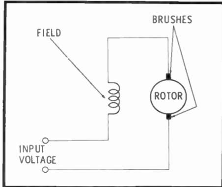
As you recall, a DC series motor will continue to turn in the same direction if the line connections are reversed. A series DC motor will therefore work on AC. In fact, a universal motor is simply a DC series motor whose windings and pole pieces are designed to operate efficiently with AC power.
