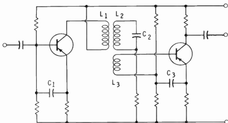
of the tuned circuit. Energy is easily transferred to  $L_3$  by transformer action. At all other frequencies the circulating current is much less, and the energy transfer is very low.
