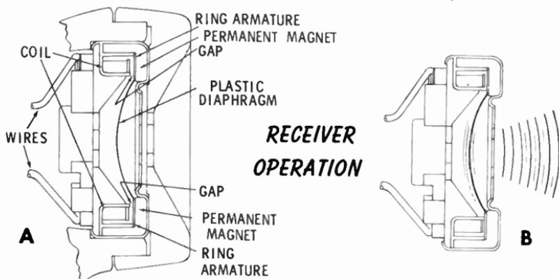
Part B shows that the diaphragm vibrates when a sound-varying current passes through the receiver. The current passing through the coil develops a magnetic field which varies in strength with the changes in current. Thus, the field developed by the current periodically repels and attracts the steady magnetic field of the permanent magnet, causing the magnet to which the diaphragm is fastened to move back and forth. This action reproduces the original sound.
