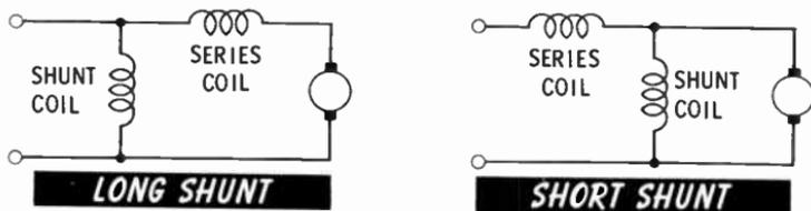
By proper control of the relative strength of the two field coils, the compound motor may be used to meet any requirement that can be met by a pure series motor or a pure shunt motor. The characteristics shown on the opposite page apply to a typical compound motor, but not necessarily to every compound motor.
