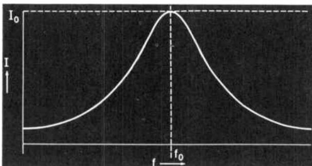
The quality of a resonant circuit can be measured by the Q factor. Q is the ratio of the energy stored in the capacitor and inductor divided by the energy dissipated in the resistor.
