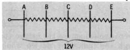
If the resistance, which shows a voltage difference of 12V from one end to the other, were divided into equal quarters, each quarter would represent 3V. Now divide both resistances of the parallel circuit into equal quarters.
