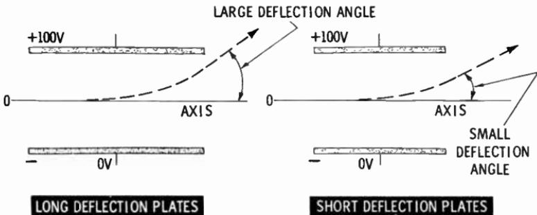
**Spacing Between Plates**—The closer together the plates, the more effect the electric force has on the electron beam.
