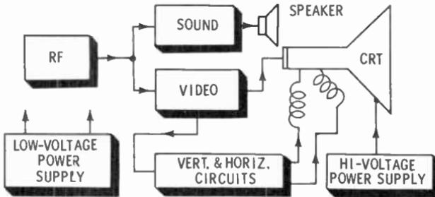
Suppose that during Step 1 you learned the following symptoms. Audio appears to be good, but the picture covers only half of the screen vertically. Width appears to be proper. Adjustment of the vertical control makes no apparent change in height, but does cause the picture to roll.
