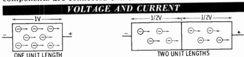
Do you recall the voltage distribution which occurs across a resistance? If one volt is applied across one unit length of wire, for example, what will happen to the voltage distribution across the same size wire that is twice as long? One-half volt will appear across each unit length. One-half the total voltage will be dropped across each of the two units. Since the resistance is doubled, the current will be one-half as much.
