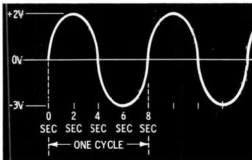
From zero to 2 seconds the voltage is rising in the positive direction. It decreases to zero volts, following the same shape curve, in the next 2 seconds. At this point it has completed one half of its full cycle. This portion of the waveform is called the **positive half cycle**.
