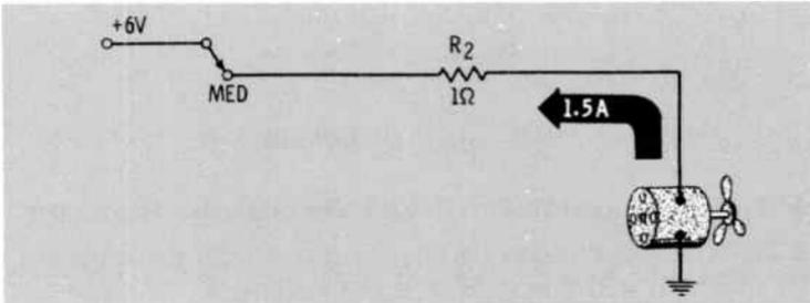
**Q31.** What is the resistance of the motor when the switch is in the HI position?
