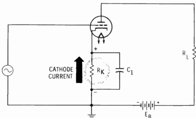
bias is provided by the use of a cathode-bias resistor. The circuit for this is shown above. There are other types of automatic bias that work on similar principles.
