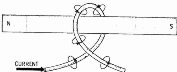
through them. A coil with a large number of turns has a magnetic field of greater strength than one with a small number of turns. The magnetic field is greater when a larger current flows through the coil.
