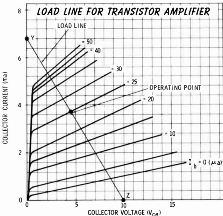
When designing a transistor amplifier, it is often important to make certain that the transistor will operate on a linear (straight-line) portion of the curve; otherwise, the output will be distorted.
