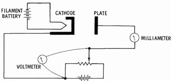
arm of the variable resistor is changed, read the voltage and the current. After recording several of these readings, plot a graph similar to the one on page 36.
