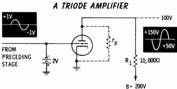
With this bias, plate current is 0.01 amp (10 ma). The cathode-to- $B+$  path contains  $R_1$  and  $r_p$  as resistances in series.  $R_1$  is the load across which the voltage for the next circuit is developed;  $r_p$  is a variable resistance existing between cathode and plate. This variable resistance is known as the **plate resistance**. When plate current increases,  $r_p$  decreases; when plate current decreases,  $r_p$  increases.
