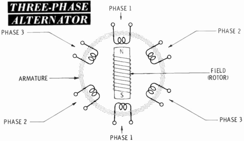
The three single-phase voltages of a three-phase alternator are usually 120 electrical degrees apart. As in the two-phase machine, it is possible to obtain single-phase voltages and also voltages between phases. The relationship
