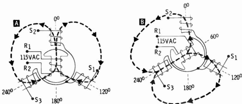
In part A, the rotor is positioned at zero degrees. When 115V AC is applied to the rotor winding (the primary), a magnetic field is developed. As in any transformer, lines of flux cut the secondary windings inducing a voltage in them.
