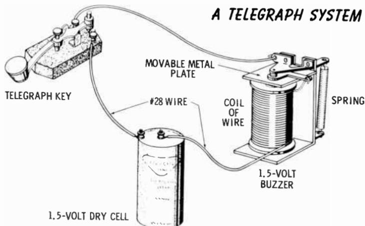
When the telegraph key is closed (pressed down), current flows from the battery through the coil of wire. The resulting magnetic force causes a movable metal plate to be attracted to the soft-iron core of the coil, producing a buzzing sound. In this manner dots and dashes (short and long buzzes) are transmitted.
