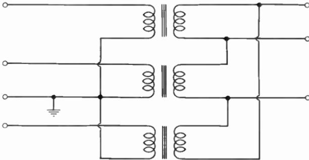
**A27.** The primary phase voltage is  $1,000\text{V}$ . The secondary phase voltage is  $1,000/10 = 100\text{V}$ . Since the secondary is wye-connected, the **secondary line voltage** is  $173\text{V}$ .
