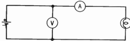
**A20.** Operating  $R = \frac{E \text{ applied}}{I \text{ drawn}} = \frac{9}{0.5} = 18 \text{ ohms}$
