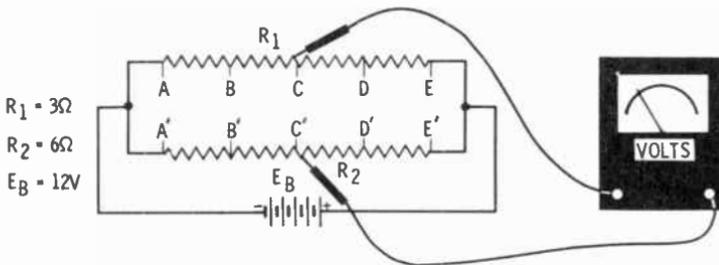
Suppose that a parallel circuit had unequal resistances, as shown above. The voltage across  $R_1$  or  $R_2$  would be identical, that is, 12V. Again assume quarter-section divisions.
