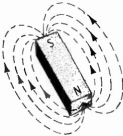
when the magnet is suspended in air, the north end of the magnet points toward the north geographic pole. Such a magnet has a magnetic field existing in the space surrounding it, with the lines of magnetic force taking the directions shown.
