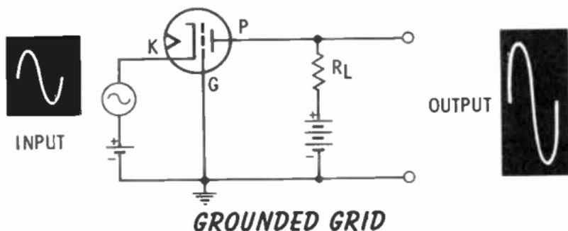
the emitter in the common-base circuit, and to the cathode in the grounded-grid circuit. The output signal is taken from the collector and the plate. The input and output signals of these amplifiers have the same polarity; that is, they are in phase. The common-base circuit is used mostly as a voltage amplifier. It has these characteristics:
