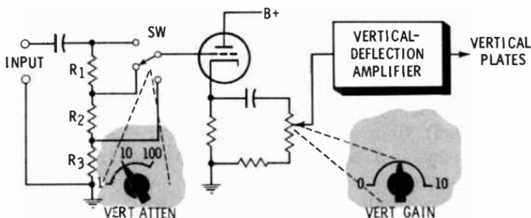
top tap of the switch in the schematic. The full voltage of the input is fed to the grid of the cathode follower. Attenuation equals  $1/10$  in position 10.  $R_1$ ,  $R_2$ , and  $R_3$  are selected so that  $1/10$  of the input voltage will arrive at the grid. Position 100 provides an attenuation of  $1/100$ .
