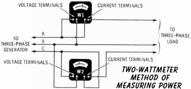
Total power is found by adding the two readings shown on the wattmeters. If the power factor of the load is less than 0.5, the wattmeter readings must be subtracted to obtain the total power. The sum (or difference) of the meter readings gives the total power because of the phase relationships of the voltages and currents in the three-phase system.
