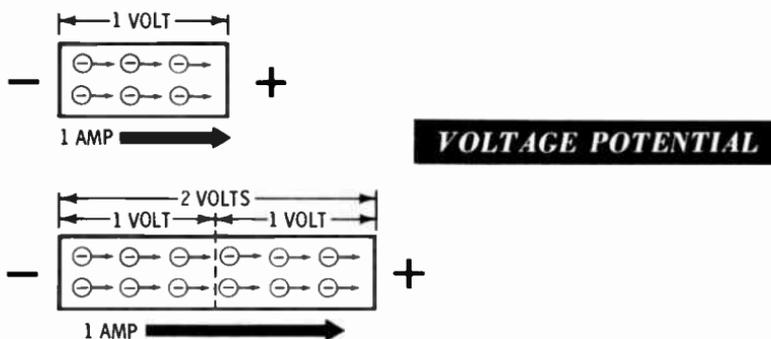
You can see that current will be the same through a conductor (with a specific voltage applied) as it is through a similar conductor twice as long but with twice the voltage
