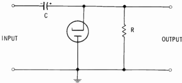
case the entire waveform is shifted above the zero level to clamp the bottom of the waveform to zero.
