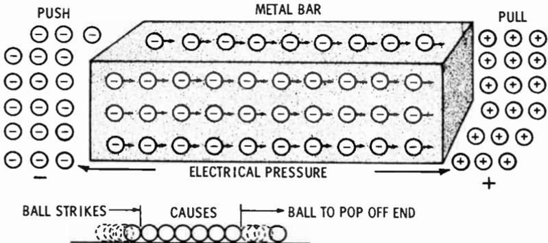
Electrical pressure is the most common form of control. This electrical pressure, or force, is made available by many forms of voltage sources.
