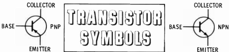
The only difference in the two symbols is the direction of the arrowhead. Be able to recognize either one. Current not only flows through the two types in different directions, but they are connected into a circuit differently.
