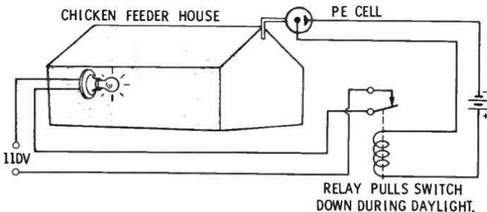
Selenium, used in solar and photoelectric cells, contains atoms that give up free electrons when struck by light. If iron is used as backing, the selenium will emit electrons into the iron. This will cause the iron to take on a negative charge, and the selenium to take on a positive charge. Wires connected to the two metals form the electrical source terminals.
