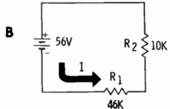
**Q7. What is the IR drop across each resistor in the following circuits?**
