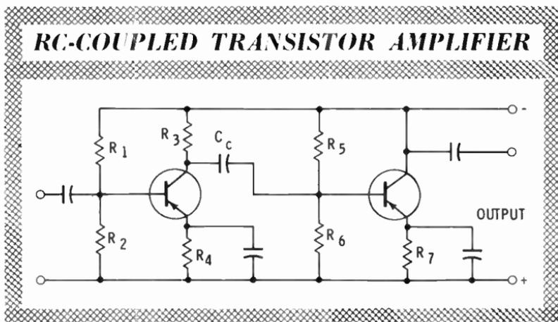
The output of the first stage is developed as a voltage across the load resistor ( $R_3$ ) and is fed to the base circuit of the second stage through coupling capacitor  $C_c$ . This capacitor represents an open circuit to all DC voltages. Thus, the biasing circuits of the two stages are not influenced by the DC voltages on the other elements.
