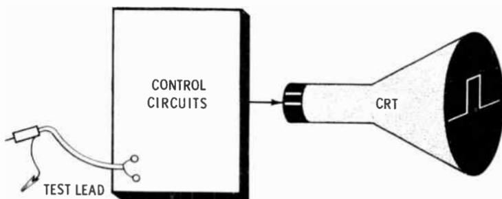
A typical oscilloscope will be described in terms of how the cathode-ray tube and the control circuits function. The test leads are only slightly different from those with which you are already familiar. Since the control circuits are designed to operate the CRT, the cathode-ray tube will be studied first.
