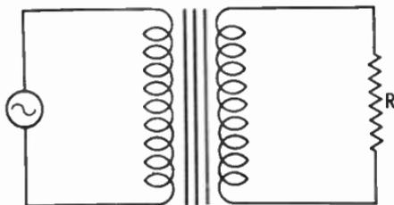
In the example above, the current was stepped down in exactly the same proportion as the voltage was stepped up. The power transferred from the primary to the secondary does not change, however, regardless of the turns ratio. This is true providing the rating of the transformer has not been exceeded and assuming 100% efficiency.
