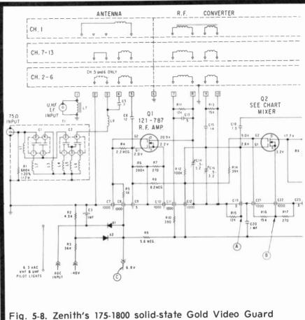
VHF turret tuner with two MOSFETs and a bipolar oscillator.
