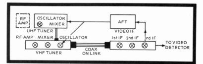
Fig. 5-1. Familiar block diagram of a tuner, AFT and IF system.
