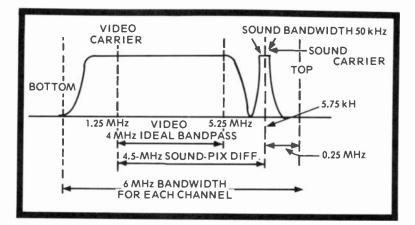
Fig. 1-2. Drawing of the 6-MHz bandpass response for all VHF-UHF TV channels showing the 4.5-MHz difference between sound and picture carriers and an ideal video bandpass of 4 MHz, something that's not realized with color.
