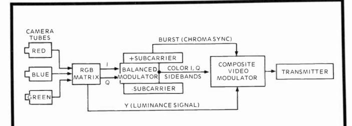
Fig. 1-10. Diagram illustrating how color signals are formed. I, Y and Q signals are combined with 90-degree out-of-phase subcarriers that are suppressed (cancelled) by balanced modulators. When there is no color, the two demodulators go to zero and only luminance is transmitted.
