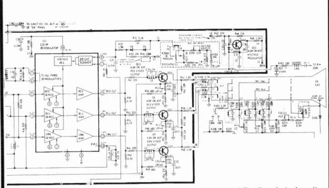
Fig. 12-10. Schematic of Motorola's color subsystem with two ICs and the discrete Instamatic circuits in between. Notice that luminance is added at the secondary centertap of T1 going into the demodulators. Other systems insert luminance after the demodulators.
