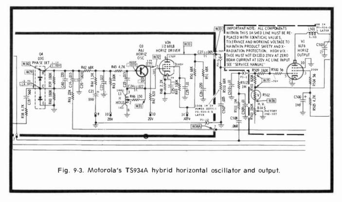
Later horizontal tube circuits have an output tube regulating device that is basically a pulse (and-or DC) feed from the flyback transformer through a capacitor and varistor that biases the output tube grid to keep it from going heavily positive and burning up the plate circuit should there be too heavy a high-voltage demand.
