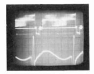
Fig. 14-5. Video and sync at 10 microseconds per division. Top amplitude 2v per division; the bottom is 0.5v per division.
