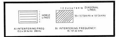
Fig. 13-12. How to tell difference frequency of interfering signals in multiples of vertical and horizontal sync rates. Notice that we said "difference" frequencies and not fundamentals. The interfering frequencies is 5 X 39.94 Hz. (A) At (B) the interfering frequency is 157.34 kHz.
