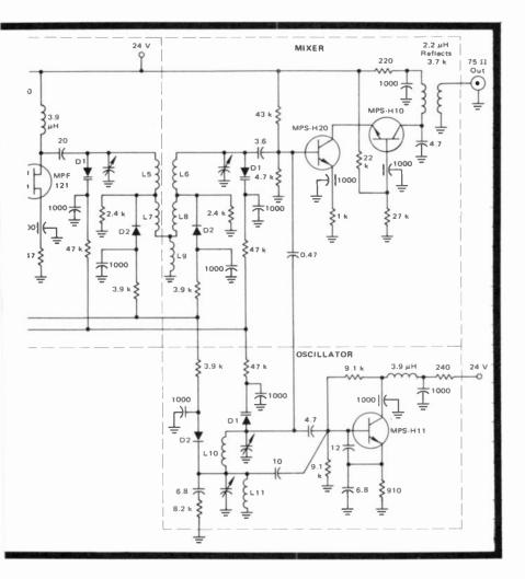
trapped 41.25-MHz audio carrier and the 45.75-MHz video carrier. Chroma is clustered at the 0.5-MHz sum and difference frequencies about the suppressed chroma subcarrier at 3.6 MHz. Video IF strips often develop a tilt that must be compensated by a reverse, equalizing tilt in the chroma amplifiers.
