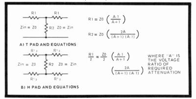
Fig. 13-9. Signal attenuating T and H pads where input and output impedances match. T pad (A) and equations; H pad (B) and equations.
