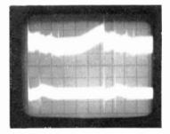
Fig. 14-9. Normal ripple of 0.5v per division in the 160v supply and 0.2v per division in the 30v supply; top and bottom traces, respectively.
