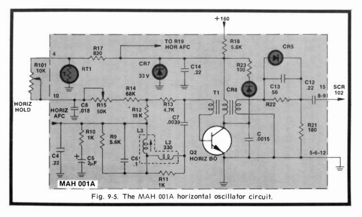
kHz; therefore, the period of one-half cycle is approximately equal to the duration of one scanning interval. Refer to Fig. 9-6.
