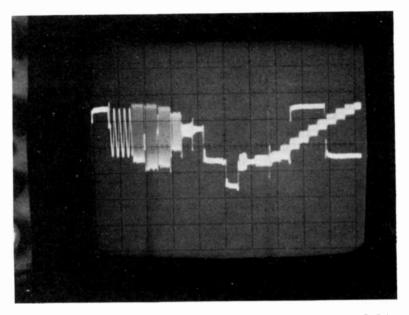
Fig. 3-9. Actual photo of a good resolution VIT on an RCA CTC46. Bandpass is 3.5 MHz.
