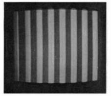
Fig. 14-55. Red demodulator output open.
