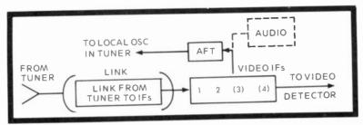
Fig. 1-14. Block diagram of the tuner and video IF link connector on many older sets, using 2, 3 or 4 stages of video IF. Automatic fine tuning (AFT) keeps the local oscillator in the receiver from drifting off proper tuning.
