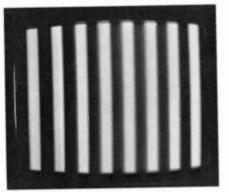
Fig. 14-61. Open input to the red demodulator.
