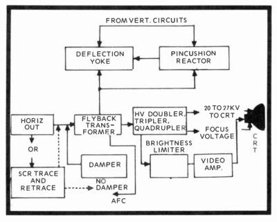
Fig. 10-9. Block diagram of a modern high-voltage subsystem.
