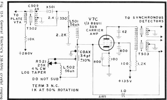
Fig. circuit. 12-9. (Courtesy General Bob Hannum) Electric's 3.58-MHz crystal ringing
