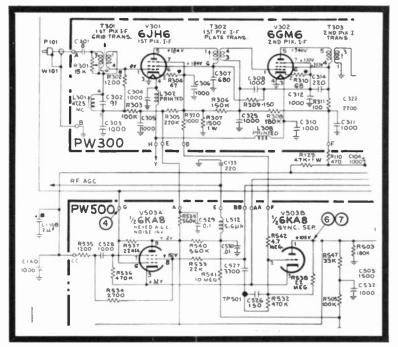
Fig. 7-2. Schematic of the vacuum tube keyed AGC, noise and sync circuits used in RCA receivers.
