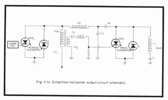
labeled S1. Retrace elements SCR2 and D2 comprise another SPST switch labeled S2. The relationship of the yoke current waveshape and the beam trace-retrace also is illustrated in Fig. 9-15.
