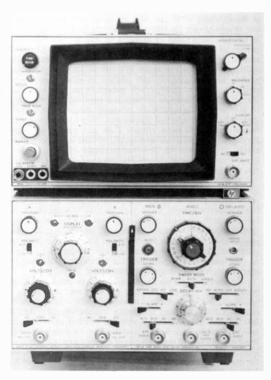
Fig. 14-1. H-P's 50-MHz dual-trace scope with A and B time bases, mixed sweep, and a time base that (with 10X magnifier), will display waveforms at 10 nanoseconds per division.
