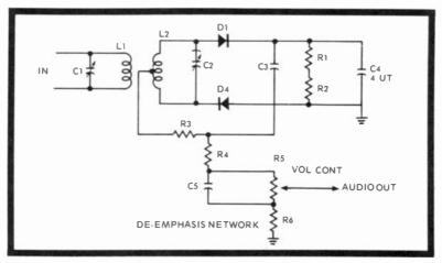
Fig. 6-15. An F-S successor, the unbalanced ratio detector which is less susceptible to AM noise.
