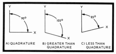
Fig. 12-3. Angles of demodulation used in the past and present to drive R-Y, B-Y and sometimes G-Y, although G-Y is always a function of the reds and blues. A) quadrature was Zenith's original; B) now the phase angle used by almost everybody; C) RCA's most copied X and Z original.
