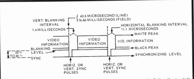
Fig. 1-8. A standard video waveform is very similar in appearance at both line (horizontal) and field (vertical) scope sweep frequencies. The difference is that at the line rate you're only viewing one or perhaps two lines of information, while at the field rate you see the entire raster scanned once for a field and twice (two complete cycles) for a frame (complete picture).
