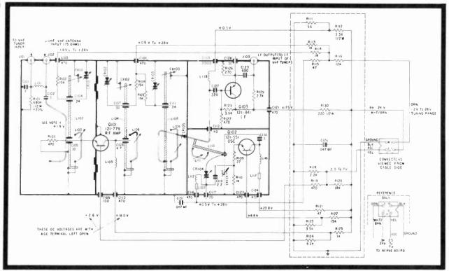
their MV3102, MV3141 varactor diodes and MPN3401, MPN-3402 pin switching diodes. The tuner has both a high and a low band, with diodes D2 (five of them) either being reversed or forward biased. The diode bias level and inductors L1, L4, L7 through L10 change the frequency response of the tuned circuits. Thereafter, the D1 series of varactors are programmed by tunable resistors.
