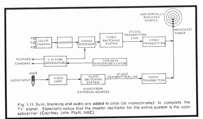
the overall system so you will have a workable mental picture of the entire process. The additional necessities in either color or monochrome are the vertical and horizontal sync signals and sound.
