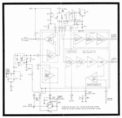
Fig. 5-16. Block diagram of the RCA CA3068 IC video IF, showing internal functions and external components.
