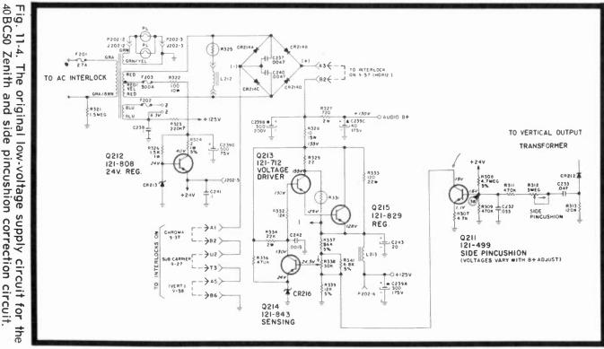
C50 4. The original low-voltage supply circuit for Zenith and side pincushion correction circuit.
