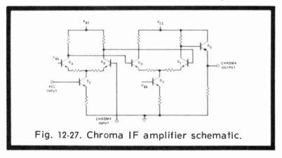
base of Qb from the video detector and the bandpass transformer at an amplitude of from 10 to 200 millivolts p-p. Automatic chroma control voltage at the base of Qc controls the DC gain of both transistors, with outputs to the bases of Qd and Qe, another differential amplifier supplied by constant current source Qf. Emitter follower Qg is the output with AC at about 2 volts p-p, and this voltage goes into the demodulators through an output that contains both level and tint controls.
