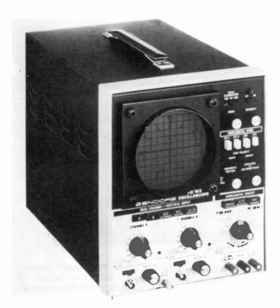
Fig. 14-22. Dual-trace, triggered and free-run sweep, Sencore PS163 scope with front panel vector inputs; deflection factor to 5 millivolts, sweep to 100 nanoseconds.
