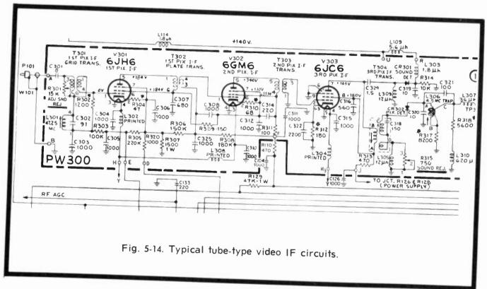
The 6JH6 is a semi-remote cutoff pentode used in gaincontrolled video IF stages and is an offspring of the old 6BZ6. Open transconductance is 8,000 micromhos, but with a control grid voltage of -4.5 volts, it drops to between 400 and 900 micromhos.
