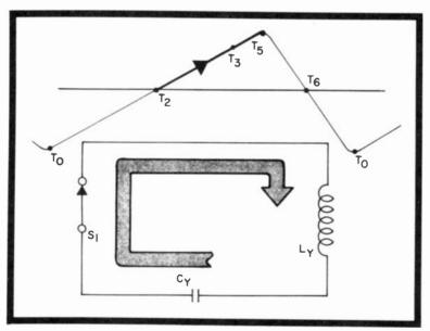
Fig. 9-17. Circuit current T2 to T5; during the second half of the trace, Cy discharges into the yoke windings.
