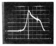
Fig. 14-39. Incorrect bias distorts the response curve.
