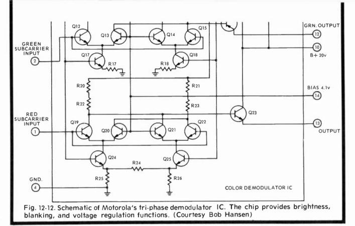
Q2), green (Q12 and Q13) and red (Q19 and Q20) demodulators, respectively. The DC bias for the bases of the differential amplifiers' synchronous switches already identified comes from the external 20-volt supply to Q2, Q3, Q13, Q14, Q20, Q21.
