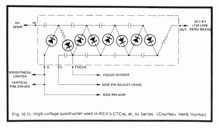
Unlike conventional high-voltage power supplies which rectify a positive pulse from the flyback transformer with a half-wave rectifier, the CTC49 uses a solid-state quadrupler to produce high voltage. This reduces the required pulse amplitude from about 23KV to nominally 6KV. The quadrupler itself is hermetically sealed and is not repairable; however, its schematic is shown in Fig. 10-11 as a means of identifying its external connections.
