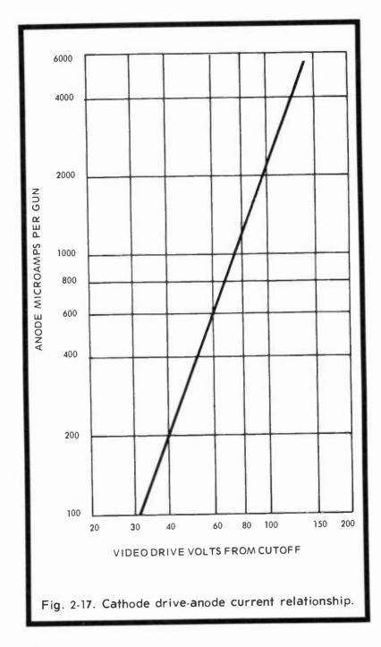
The maximum average current drain from the chassis high-voltage supply seldom exceeds 1500 microamperes which means that each of the three guns is delivering a maximum average current of about 500 microamperes or 0.5 ma. However, the external and internal coatings on the CRT form a capacitor which stores power for higher peak current requirements.
