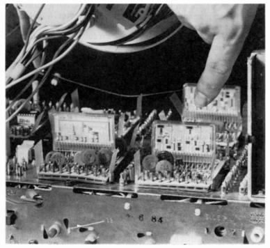
Fig. 9-22. Rear chassis view, showing thick film hybrid circuits serving as the horizontal, vertical, and subcarrier regenerator in Zenith's 25CC55 receivers.
