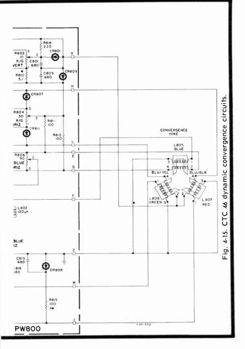
voltages, depending on the circuit positions and forward (anode-to-cathode) bias. In this newer arrangement, the red and green convergence portions parallel the blue in the top and bottom red-green convergence, while top and bottom blue convergence adjustments are simply in parallel with the blue convergence yoke coils. The various potentiometers determine current flow into the several portions of the convergence coil windings.
