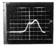
Fig. 14-43. With the 4.5-MHz marker cut off, the spurious one is on the left and is immediately recognizable.
