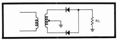
Fig. 6-3. Full-wave video detector diode circuit, which is not practical for color TV in the simple form.
