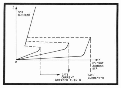
Fig. 9-12. SCR conduction and gate current relationship.
