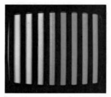
Fig. 14-56. Green demodulator output open.
