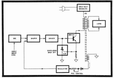
Fig. 11-8. Complete block diagram of the electronic power supply. (Courtesy Chuck Preston)
