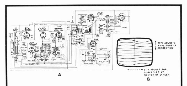
Fig. 10-2. A vacuum tube high-voltage subsystem with yoke and pincushion transformer circuits. The drawing illustrates the reason for center curvature and amplitude pincushion sweep corrections.
