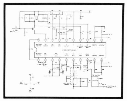
Fig. 12-31. Complete chroma circuit block diagram with all external connections. (Courtesy Fairchild Semiconductor)
