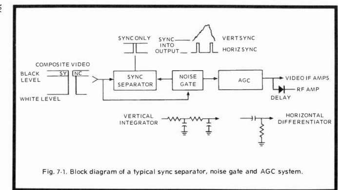
more interest in detecting increases in AGC action that affect a receiver front end and cause viewing problems that can be prevented by selected settings of the noise circuit.
