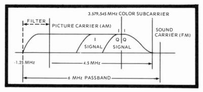
Fig. 1-3. The same monochrome characteristics in Fig. 1-2 are indicated here, but with color information now added. The drawing also shows the effect of a filter for negative vestigial sideband compression. Notice I and Q signals on either side of color subcarrier, plus the color sync subcarrier.
