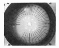
Fig. 14-48. One available color-bar generator produced a pattern with considerable smear.
