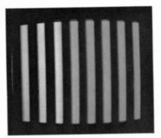
Fig. 14-62. Shorted green demodulator input.
