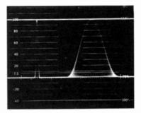
.250 µs HAD Sin<sup>2</sup> Pulse (left) and Modulated 20 T Sin<sup>2</sup> Pulse (right) with superimposed Bar Signal (top).
