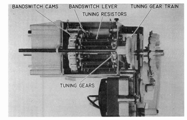
Fig. 5-9. resistors E. UHF-VHF 1 Zenith's a bandswitch, cams, all-varactor tuner. and tuning
