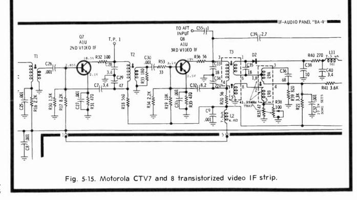
Yet, the considerably lower voltage power supplies (in this instance, 20 volts vs 405) and the relatively small currents, plus plug-board flexibility, makes the modular type solid-state chassis quite attractive from many standpoints. With transistors, impedances are lower, of course, and this usually increases noise immunity, but inductor and capacitance coupling between IF stages still exists as it did almost 20 years ago.
