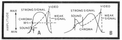
Fig. 7-5. The sound and video IF response characteristics rise ideally and proportionately with a shift from strong to weak incoming signals. Video rises in proportion to sound on a weak input at the video IF curve (A). Sound IF detector response (B) showing the sound and video rising and peaking on very weak signals. (Courtesy Karol Siwko)
