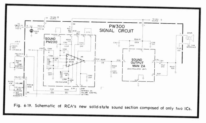
B (approximately) push-pull output coupled through a 150-mfd capacitor directly to the speaker.
