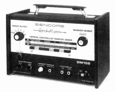
Fig. 14-19. Sencore's SM158 Speed Aligner for VHF TV RF, IF, and chroma alignment.
