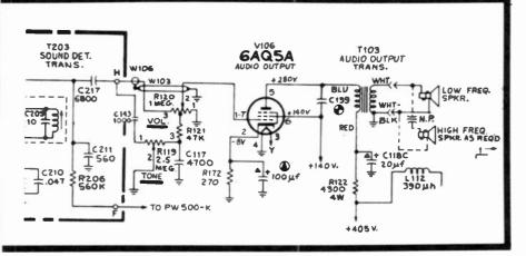
Fig. 6-16. RCA CTC25X vacuum tube sound subsystem circuits.
