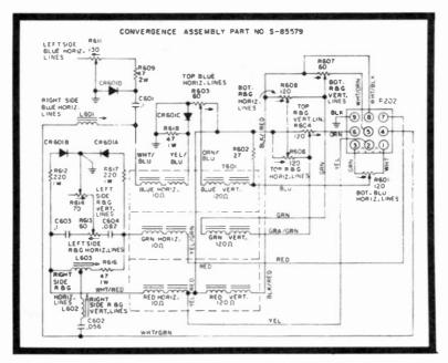
Fig. 4-16. Zenith 4B25C19 series dynamic convergence board schematic.
