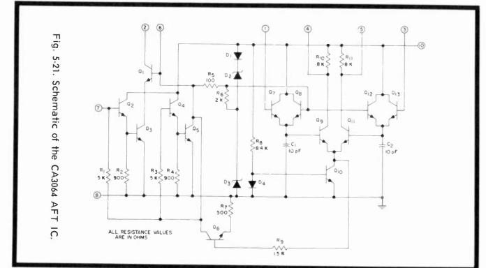
correction. For instance, a negative frequency deviation causes Q9 to conduct more and a positive frequency deviation turns on Q11 harder.
