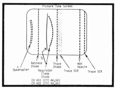
Fig. 14-16. Vertical interference lines are caused by trouble in a solid-state receiver's horizontal sweep system.
