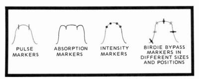
Fig. 14-17. Various types of markers are used. Markers must be added to the response curve only after the sweep has passed through all tuned circuits to prevent distortion.
