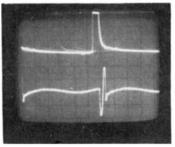
Fig. 14-7. The top trace is the horizontal sync pulse; the lower trace is the sine-wave horizontal oscillator output, 10 volts per division and 1 volt per division, respectively. Time base, 10 microseconds per division.
