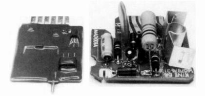
Fig. 12-21. Interior of MAD module from its beginning as a discrete, to thick film on ceramic substrate, then final encapsulation. (Courtesy RCA)
