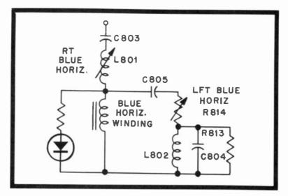
Fig. 4-13. RCA CTC 40 blue horizontal convergence circuit.
