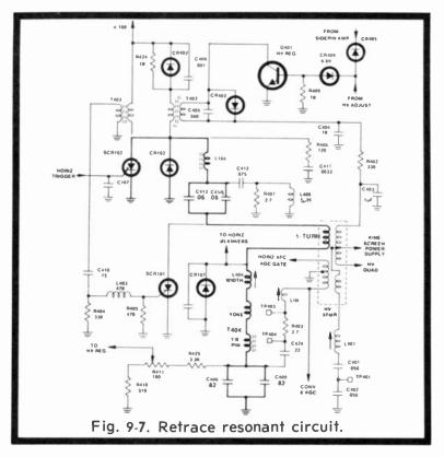
voltage regulator, to be explained. Current flowing through T403 generates a positive gate voltage for SCR101 during most of the scanning interval. Refer to Fig. 9-8.
