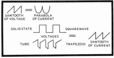
Fig. 4-9. Dynamic convergence currents developed by voltages from the horizontal output circuits.
