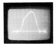
Fig. 14-27. Final IF alignment curve. Markers left to right in MHz are: 39.75, 41.25, 42.17, 44.25, 45.75, 47.25.
