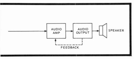
stages of audio amplification. The speaker in more recent receivers may be capacitor or transformer coupled.
