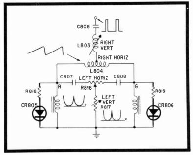
Fig. 4-12. RCA CTC 40 R-G horizontal convergence circuit.
