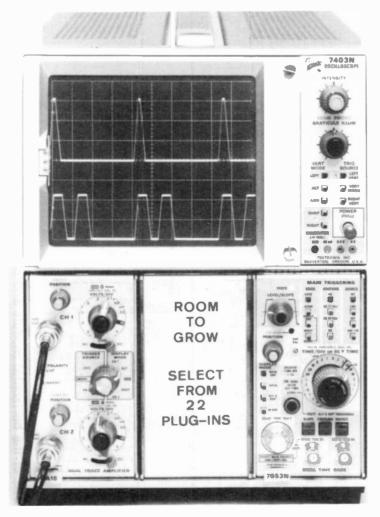
ig. 14-2. Tektronix 50-MHz oscilloscope with three plug-in nits. It is accurate to 2 percent, with 1.22 cm per division. The unit features an 8 x 10 graticule, 5 mv per division ertical sensitivity, two time bases, and room to grow.
