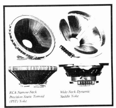
Fig. 2-12. RCA's new PST torrodial yoke compared with the wide-neck saddle type. As yoke and tube matches become closer, convergence problems diminish.
