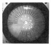
Fig. 14-37. Final vectorscope pattern after sweep alignment, an excellent verification of both procedures.
