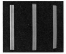
Fig. 14-69. The presence of R-Y, B-Y and G-Y permits a quickcheck of the chroma output.
