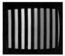
Fig. 14-68. This color-bar is useful for vectorscope analysis.
