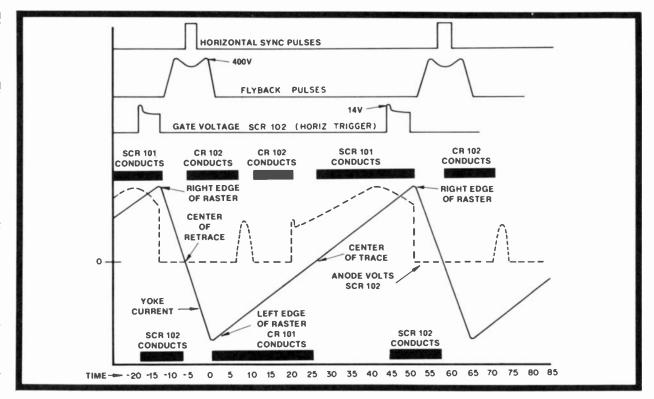
conducting, thus shorting the primary so that very little energy can enter. However, during retrace the flyback voltage pulse drives the transformer primary, and the transformer converts this voltage to a higher voltage, which is used to drive the quadrupler and CRT screen power supply. Energy transfer is optimized by tuning the transformer to the third harmonic of the retrace pulse. This is the function of L401.
