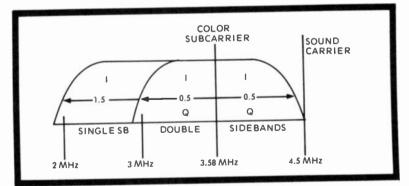
Fig. 1-5. Color I and Q double sidebands are shown on either side of color subcarrier at 0.5-MHz frequencies, with I extending to 1.5 MHz in the single sideband (to the left). The sound carrier is at upper right of diagram.
