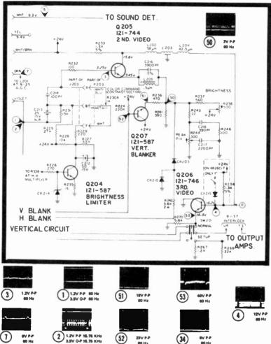
Fig. 10-5. A Zenith beam current brightness limiter circuit that controls the second video amplifier to prevent excess HV current drain.
