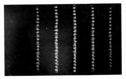
Fig. 3-3. When interference bars are vertical, divide by the line scanning rate of 52.4 microseconds to find the interfering frequency.
