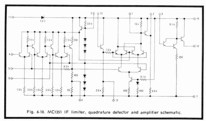
circuit. The IC input is terminal 4, since terminal 6 is actually a bypassed bias supply.
