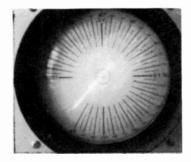
Fig. 14-46. Vector pattern indicating a need to adjust the receiver's contrast or brightness.
