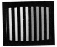
Fig. 14-63. Blue demodulator input failure.
