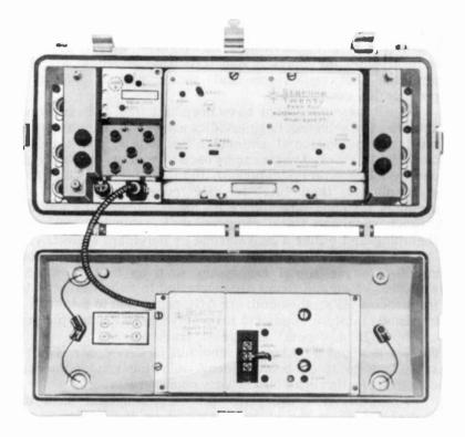
Fig. 15-6. A Jerrold Starline Twenty push-pull fully-loaded repeater amplifier station SP-1.
