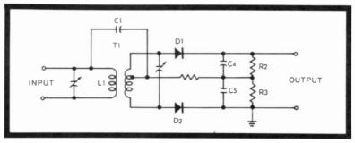
Fig. 6-14. Durable Foster-Seely discriminator circuit.
