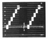
Modulated staircase signal. 2 H SWEEP, FLAT response.
