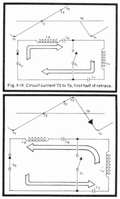
Fig. 9-20. Circuit current T6 to T0, second half of retrace.
