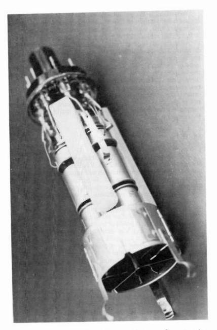
Fig. 2-15. Electron gun assembly for the Chromacolor tube showing the electrodes of the three guns. (Courtesy Rowland.)
