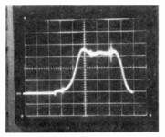
Fig. 14-38. Channel 4 response curve showing both markers. Video is on the right.
