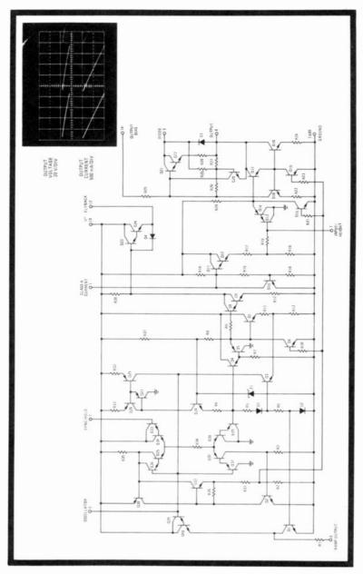
Fig. 8-4. Schematic of the Motorola Phoenix vertical output subsystem on a single IC chip. Waveforms show voltage and current outputs. (Courtesy Ben Scott)
