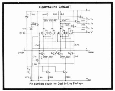
Fig. 12-17. Fairchild's uA746E synchronous demodulator IC schematic used by Zenith. (Courtesy Frank Hadrick)
