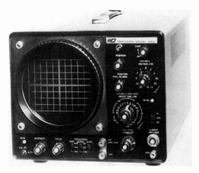
Fig. 14-23. Dynascan's B & K Type 1460 single-channel triggered sweep scope with 10 mv deflection factor, 10-MHz bandpass, and sweep 0.5 seconds to 500 nanoseconds.
