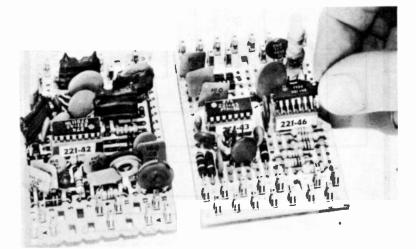
Fig. 12-13. Monolithic ICs in Zenith's 19CC19 and 25CC55 hybrid and solid-state color chassis. These three chips do all the chroma processing, and are hand-removable from their mounting sockets. (Courtesy Ed Polcen)
