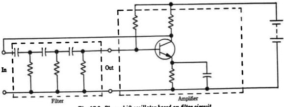
Fig. 17-9. Phase-shift oscillator based on filter circuit.
