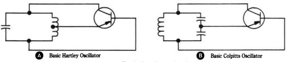
Fig. 17-4. Two basic oscillator circuits.
