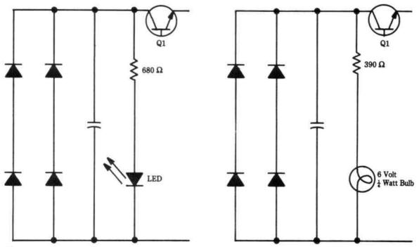
Fig. 24-3. Alternative arrangements for charging indicator lamps. A bulb of appropriate voltage could be used in one of the output leads without a dropping resistor.
