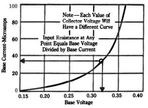
Fig. 15-1. Typical transistor input characteristics.
