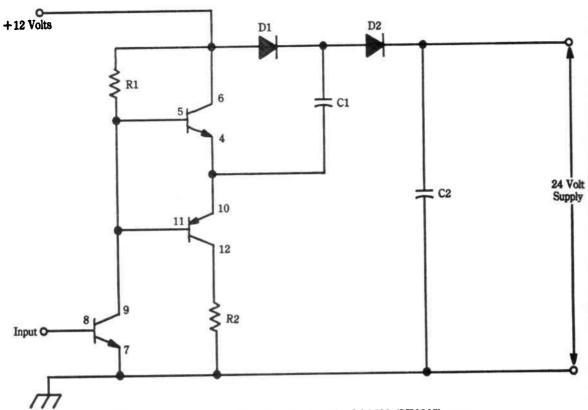
Fig. 14-5. A voltage doubler circuit using the CA3600 (SK9205) array.
