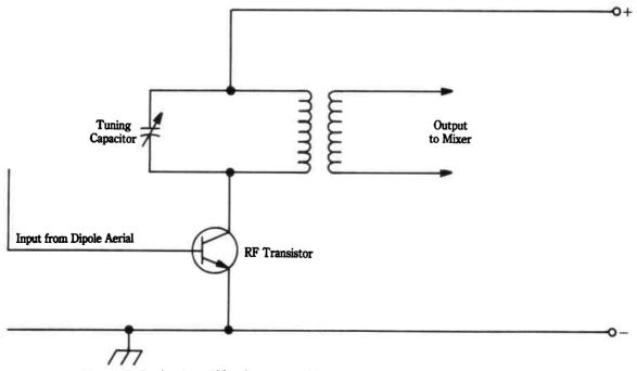
Fig. 21-3. Basic rf amplifier (or preamplifier) circuit as used in many FM receivers.
