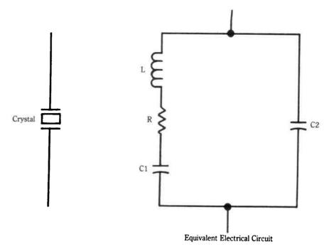
Fig. 17-7. Electrical circuit equivalent of a crystal.
