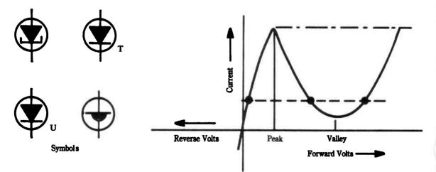
Fig. 11-3. Symbols (left) and characteristic performance of a tunnel diode. From peak to valley it exhibits negative resistance.
