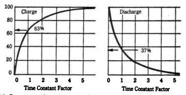
Fig. 6-1. Percentage voltage across capacitor related to time when being charged (left) and discharge (right).
