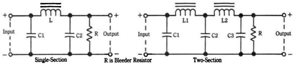
Fig. 25-3. Single and two-section smoothing filters.
