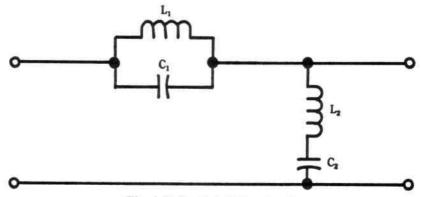
Fig. A-7. Band-stop filter circuit.
