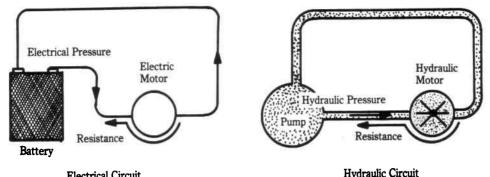
Electrical Circuit Hydraulic Fig. 2-1. An electrical circuit is similar to a hydraulic circuit.
