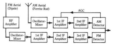
Fig. 21-10. Basic design of an AM/FM receiver shown in block form. The only common circuit is an af amplifier (usually a class B output) following the detectors.
