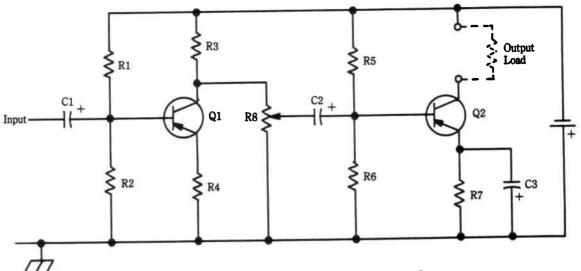
Fig. 16-7. Two stage amplifier with volume control.
