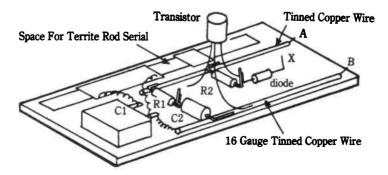
Fig. 19-2. The same circuit as Fig. 19-1 tackled by just connecting components together via their open leads, and using bare wire for top and bottom lines.
