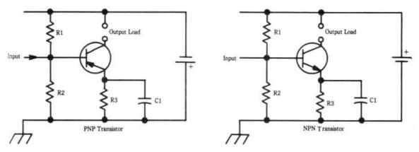
Fig. 9-9. Voltage bias circuits for transistor operation.
