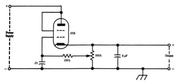
Fig. 25-11. Variable voltage supply.
