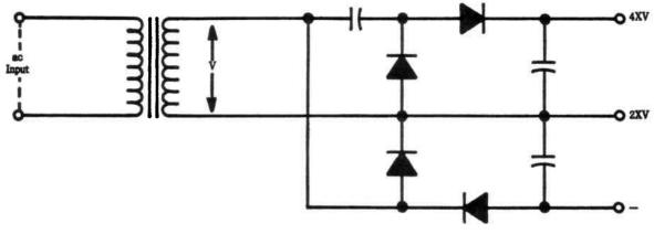
Fig. 25-10. Voltage-multiplier circuit using diodes.
