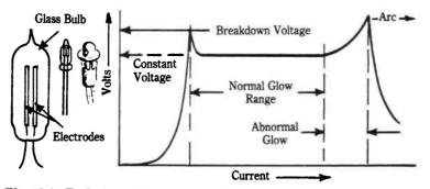
Fig. 10-1. Typical neon lamp construction and characteristic performance.
