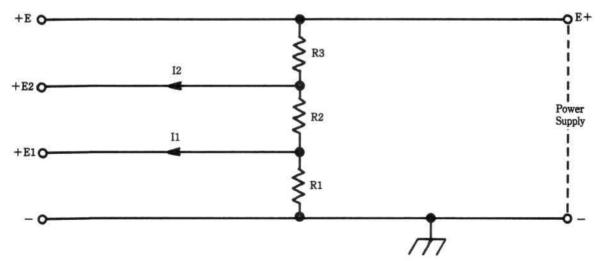
Fig. 25-8. Conventional voltage divider.
