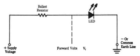
Fig. 10-8. LEDs are connected with a ballast resistor in series to drop the supply voltage in the required forward voltage. Note the symbol for an LED (light-emitting diode).
