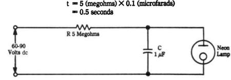
Fig. 6-3. Simple neon flasher circuit (note the symbol for a neon lamp). The values of the resistor (R) and capacitor (C) determine the flashing rate.
