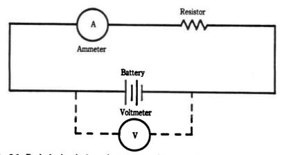
Fig. 3-1. Basic dc circuit shown in two ways, with meters for measuring current and voltage indicated.
