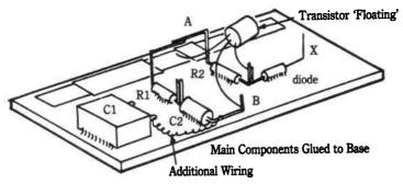
Fig. 19-3. Bonded mounting is similar to Fig. 19-2 but all components (except transistors) are glued down to a base panel. Turn up ends of leads to form connecting points.
