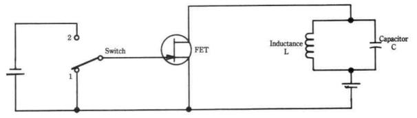
Fig. 17-1. Demonstration circuit for LC oscillator.
