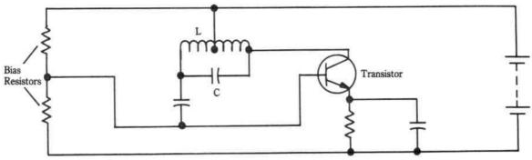
Fig. 17-5. Practical Hartley oscillator circuit.
