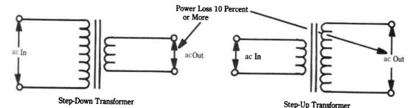
Fig. 8-2. Step-down and step-up transformers defined. In practice, transformers are often drawn in symbolic form with both coils of the same length, regardless of actual turns ratio.
