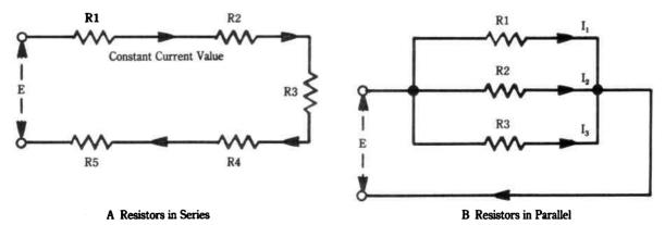
Fig. 3-2. Current has the same value through all resistors connected in series, but is different through each resistor connected in parallel.
