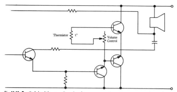
Fig. 11-13. Practical circuit incorporating a thermistor to counteract fluctuations in value of other resistors in the circuit due to heating effects or temperature changes.
