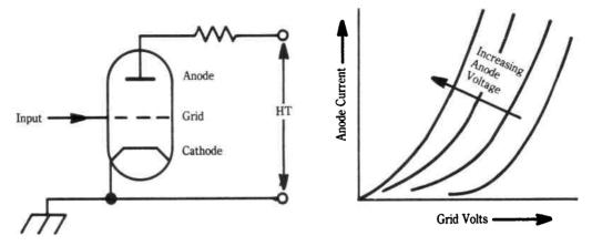
Fig. 12-3. A triode is a three-element tube. Anode current is controlled by the grid bias voltage.
