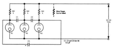
Fig. 10-6. Sequential flasher using NE-2 miniature neon lamps (or equivalent).
