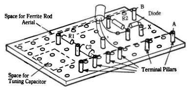
Fig. 19-6. Pegboard assembly is similar to Fig. 19-5 except that the board is predrilled to accept terminal posts. Locate these posts at suitable points to act as common connecting points. Connect components to posts, then complete the additional wiring as necessary. Note: all these constructional drawings show the same circuit — a simple single-transistor radio receiver with preamplifier. Components required are:
