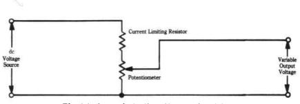
Fig. 4-4. A practical adjustable potential divider.
