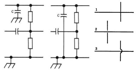
Fig. 18-5. The capacitor (C) is connected between top and bottom lines, but may be shown in a circuit diagram in either of these two ways. On the right are three ways of drawing crossing lines with no connection. Method 1 is the usual way; method 2 is clearer still.
