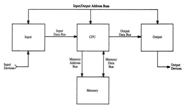
Fig. 13-4. Block diagram illustrating the basic operation of a computer.
