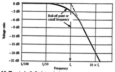
Fig. 6-8. The actual roll-off point on the frequency response curve of a filter is not sharply defined. The cutoff frequency is really a nominal figure and generally taken as the frequency at which there is a 3 decibel loss or a volts in/volts out ratio of 0.707. This is equivalent to a 50 percent loss of power.
