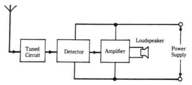
Fig. 18-1. Basic stages in a simple radio receiver.
