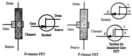
Fig. 9-11. Construction of field-effect transistors shown in simple diagrammatic form, together with appropriate symbols for FETs.
