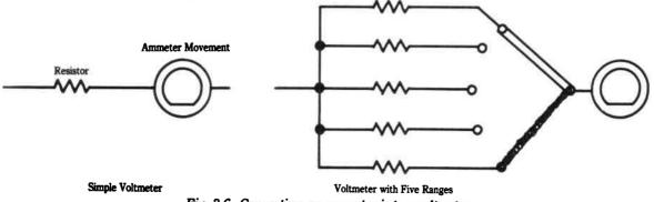
Fig. 3-6. Converting an ammeter into a voltmeter.
