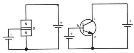
Fig. 9-6. Bias and supply connections to an NPN transistor, shown diagrammatically (left) and in symbolic form (right).
