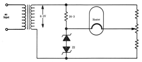
Fig. 25-12. Stabilized heater supply.
