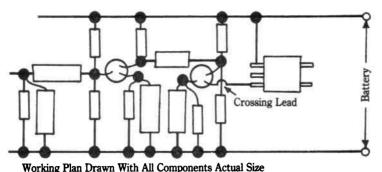
Fig. 18-7. Typical component layout drawing or working plan. This is the same circuit as Fig. 18-3, following the tuned circuit (which would be a ferrite rod aerial.
