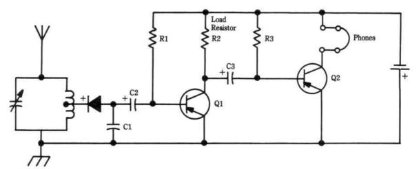
Fig. 16-3. Crystal set with two stages of amplification. Component values matching SK3007A or near equivalent for Q1 and Q2.
