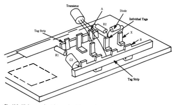
Fig. 19-5. All the connecting points are formed by tag strips or individual tags mounted on the panel. Solder components to appropriate tags, and complete with additional wiring as necessary.
