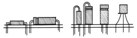
Fig. 20-1. Horizontal mounting of components on a PC board takes up more space, but is usually more convenient than vertical mounting (except for transistors).
