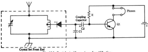
Fig. 16-2. Crystal set with one stage of amplification.
