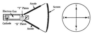
Fig. 12-5. Simplified diagram of a cathode-ray tube.
