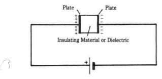
Fig. 5-1. Illustrating how a capacitor builds up a charge when connected to a dc voltage, blocking current flow.
