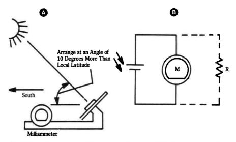
Fig. 11-11. Aligning a photocell to measure solar energy (left). The circuit on the right is a complete solar energy meter, a 0-500 milliamp type.
