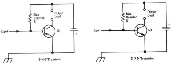
Fig. 16-1. Basic amplifier circuit.
