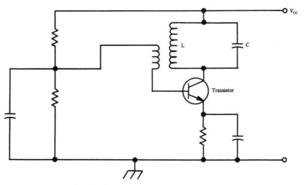
Fig. 16-11. Using an output transformer to balance the load.
