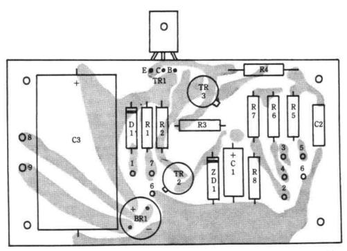
Fig. 20-5. Example of a printed circuit design with copper area shown shaded and position of components indicated.
