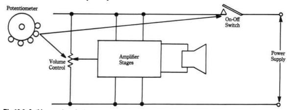
Fig. 18-6. In this example, a single component (the potentiometer connections) appears in two separate parts of the circuit diagram.
