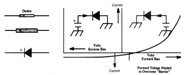
Fig. 9-7. Operational characteristics of a typical semiconductor diode.
