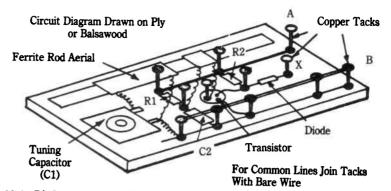
Fig. 19-1. Pinboard construction starts by drawing a working plan of the circuit on a panel of ply or balsa. Then drive in copper tacks at each connection point. Solder component leads to tacks, and complete circuit as necessary with any additional wiring.
