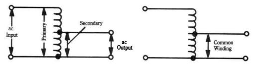
Fig. 8-6. The autotransformer is a single full-length coil with a tapping point.
