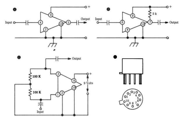
Fig. 13-2. Three amplifiers based on the CA 3035 IC, all giving a gain of about 100. All external capacitors are 10 microfarad.
