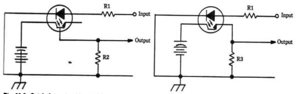
Fig. 11-9. Optoisolator (combined LED and phototransistor), operating as a photodiode (left) and phototransistor (right).
