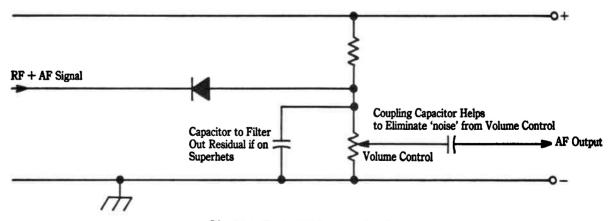
Fig. 21-4. Basic AM detector circuit.
