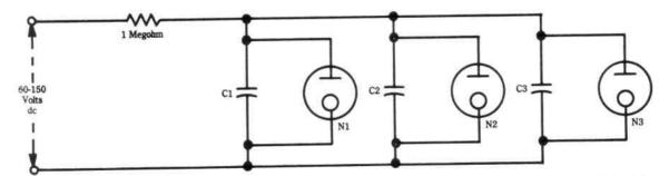
Fig. 6-4. Random cascade flasher circuit. Any number of lamps can be connected in this way and will flash in random order.
