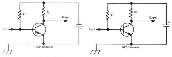
Fig. 9-8. Simple current bias circuits for transistor operation.
