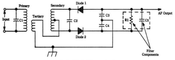
Fig. 21-5. Basic FM detector circuit.
