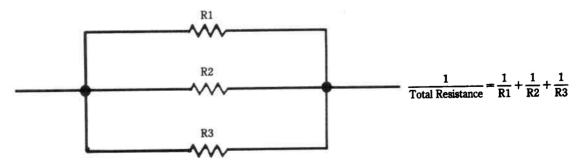
Fig. 4-7. Resistors in parallel.
