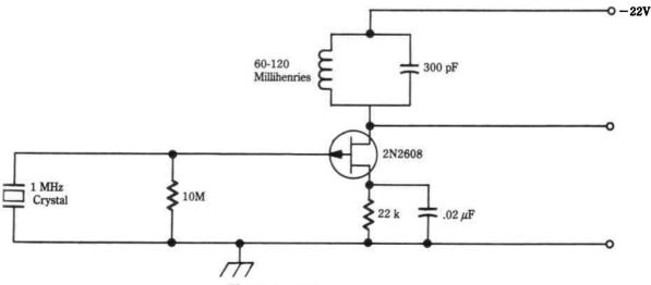
Fig. 17-8. 1 MHz crystal oscillator.
