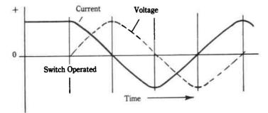
Fig. 17-2. Cycle of operation of LC oscillator.
