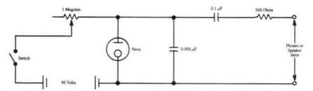
Fig. 10-5. Simple tone generator based on an NE-2 miniature neon lamp.
