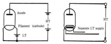
Fig. 12-1. Diode vacuum tubes with directly heated filament (left) and indirectly heated filament (right).
