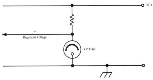
Fig. 25-5. Voltage stabilization with VR tube.
