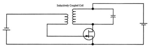
Fig. 17-3. Self-oscillating oscillator circuit.
