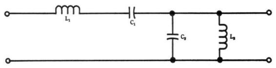
Fig. A-5. Band-pass filter circuit.
