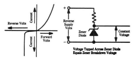
Fig. 11-1. A Zener diode, working with reverse bias, breaks down at a specific reverse voltage. Connected as shown, it can be used as a source of constant voltage supply. Note the symbol for a Zener diode.
