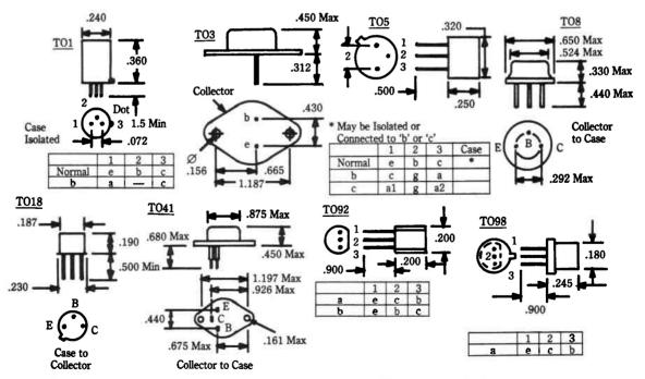
Fig. 9-10. Some common transistor outlines (diagrams by Electrovalue, all dimensions in inches).
