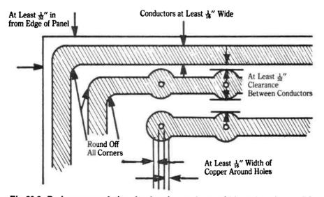
Fig. 20-3. Basic recommendations for planning conductor widths and spacings on PC boards.
