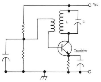
Fig. 17-11. Basic resonant circuit oscillator with transistor amplifier.
