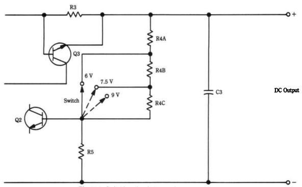
Fig. 24-2. Switching circuit for altering dc output voltage.
