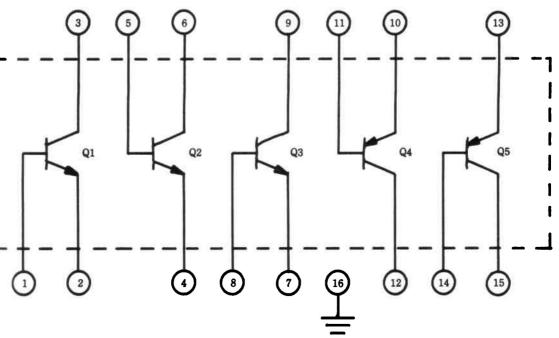
Fig. 14-4. Schematic diagram of CA3600 (SK9205) array.
