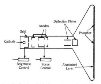
Fig. 22-1. The TV tube and its basic controls, shown in simplified form.
