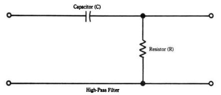
Fig. 6-10. (Right) High-pass or rumble filters cut off low frequencies but pass high frequencies. A typical value for the product RC in this case would be 125.
