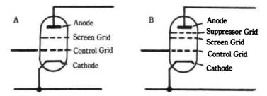
Fig. 12-4. Tetrode (left) and pentode (right) tubes shown in simple diagrammatic form.
