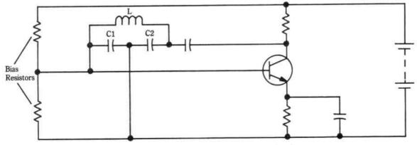
Fig. 17-6. Practical Colpitts oscillator circuit.
