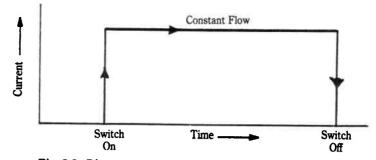
Fig. 2-2. Direct current flow with constant circuit resistance.
