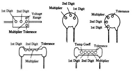
Fig. 5-5. Other coding systems used on capacitors.
