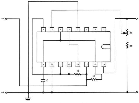
Fig. 14-3. Complete voltage regulator with wiring connections.
