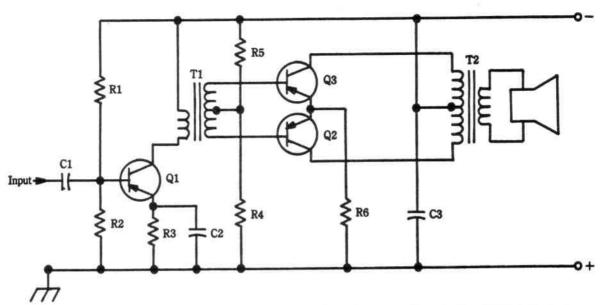
Fig. 16-10. Push-pull amplifier with transformer coupling. Q1 is the driver; Q2 and Q3 = SK3014. Typical component values:
