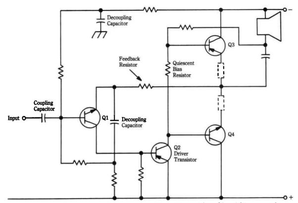
Fig. 21-8. Basic class B output circuit. Q1 acts as a preamplifier. Q2 is the driver. Q3 and Q4 are a complementary pair of transistors, working alternately in "push-pull." The two resistors shown by dashed lines may be added to improve the stability of the circuit. These only need to be of very low value (e.g., 1 ohm).
