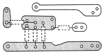
Fig. 20-4. Quite large areas of copper can be left on low voltage battery powered circuits. There is no need for consistent widths (or shapes) of conductors.
