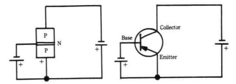
Fig. 9-4. Bias and supply connections to a PNP transistor shown diagrammatically (left) and in symbol form (right).
