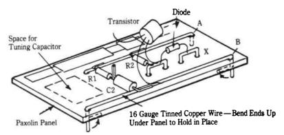
Fig. 19-4. Lay down the top and bottom lines in tinned copper wire, permanently mounted on the panel. Shorter lengths of bare wire can be used for other common connecting points. Complete by soldering component leads in place.
