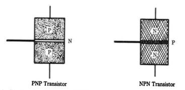
Fig. 9-3. Construction of PNP and NPN transistors, shown in simple diagrammatic form.
