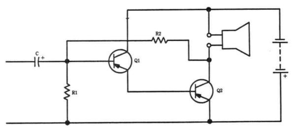
Fig. 16-4. Amplifier for loudspeaker output. Components:
