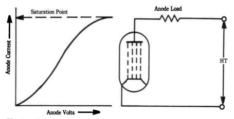
Fig. 12-2. Typical diode characteristics (left). To do useful work, the anode current must flow through a load resistor.
