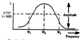
Fig. A-6. Band-pass filter-effect on frequency.
