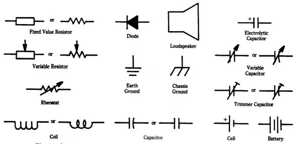
Fig. 1-1. Symbols for basic circuit components. Other symbols are given in later chapters.
