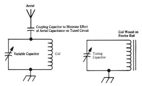
Fig. 21-1. A variable capacitor and coil form the usual tuned circuit. Strictly speaking this tunes the antenna, if an external aerial wire is used. Most AM receivers use a ferrite rod antenna which does not require an external antenna.
