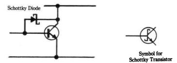
Fig. 11-4. Typical circuit for a Schottky diode (left) and the equivalent single component, a Schottky transistor.
