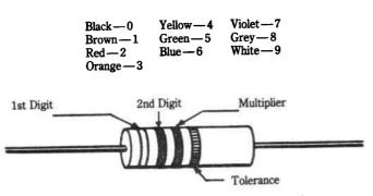
Fig. 4-1. Standard resistor color code marking.
