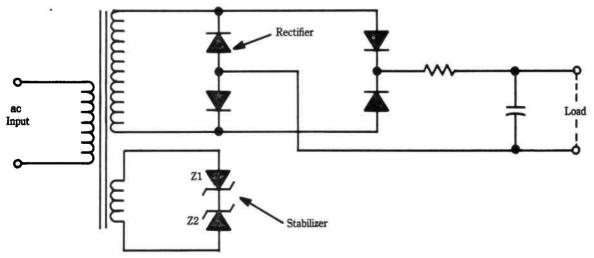
Fig. 25-6. Stabilization by Zener diodes.
