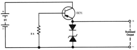
Fig. 25-15. Simple low-loss stabilizing circuit.
