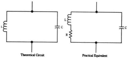
Fig. 7-4. Theoretically, only a capacitor and inductance are involved in a resonant circuit. In practice, some resistance is always present as well.
