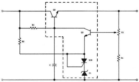
Fig. 14-2. Voltage regulator circuit using CA3097 (SK3613) array.
