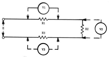
Fig. 3-3. Resistors drop voltage in a dc circuit.
