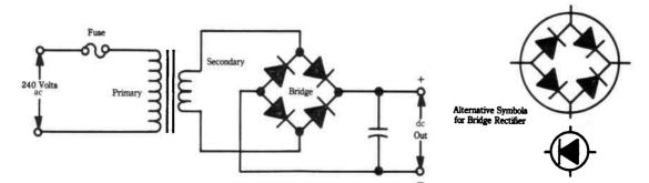
Fig. 8-5. Practical power-supply circuit. A high value capacitor is used. The four diodes are bought as a single component called a bridge rectifier.
