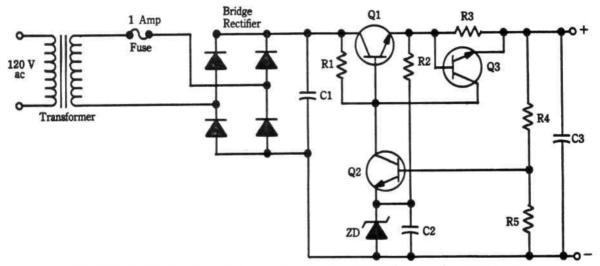
Fig. 24-1. Stabilized output dc charger operating from 120VAC power. Components are:
