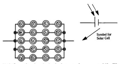
Fig. 11-10. Connections for a 2-volt solar battery to give a current of 15 milliamps through a 100 ohm load.
