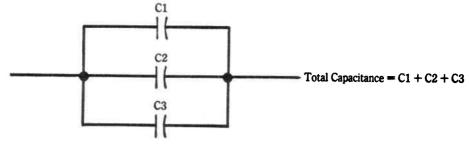
Fig. 5-7. Capacitors in parallel.
