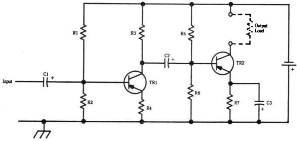
Fig. 16-6. Two stage amplifier circuit.
