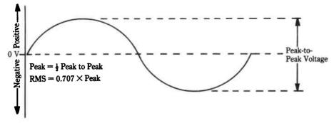
Fig. 2-4. Peak-to-peak, peak, and root mean square voltages defined and compared.
