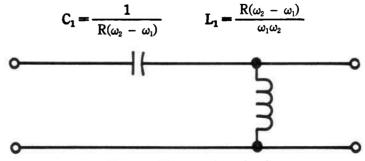
Fig. A-3. High-pass filter circuit.
