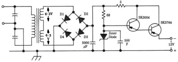
Fig. 25-13. Transistor power supply.
