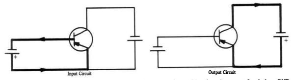
Fig. 9-5. The two separate circuits involved in operating a transistor. Direction of current flow is for a PNP transistor.
