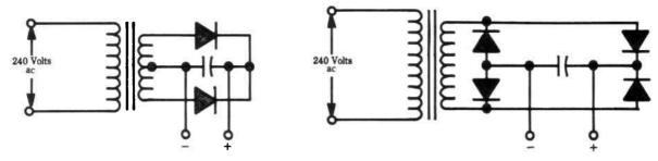
Fig. 8-4. Full-wave rectification of ac.
