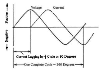
Fig. 2-5. Current usually lags behind voltage in an alternating current circuit.
