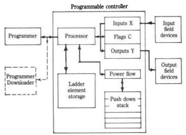
Fig. 23-1. Block diagram of Texas 510 programmable logic controller.
