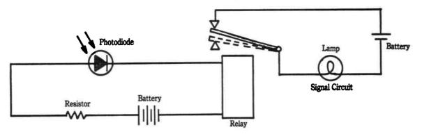
Fig. 11-6. Photodiode used as a light switch. The rise in current when the diode is illuminated makes the relay pull in completing an external circuit through the relay contacts.
