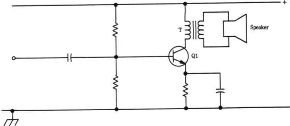
Fig. 16-8. Basic Class A amplifier circuit.
