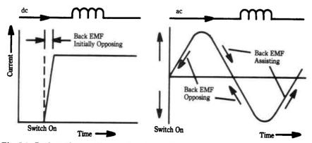
Fig. 7-1. Back emf induced in a dc circuit on switching on exists only momentarily. In an ac circuit, the back emf is continually changing.
