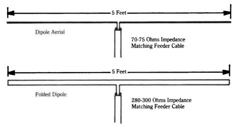
Fig. 21-2. FM antennas need connecting to the set via a correctly matched feeder cable.
