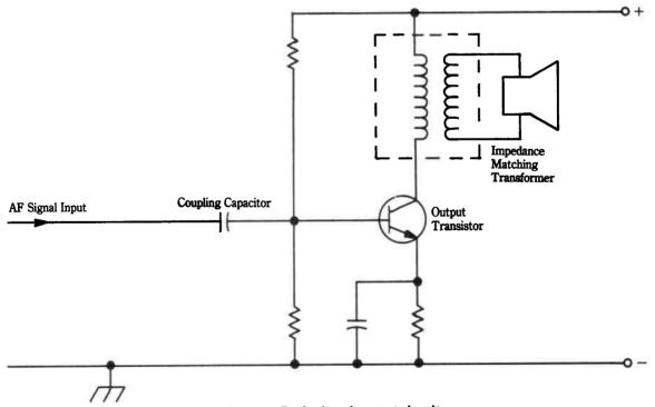
Fig. 21-7. Basic class A output circuit.
