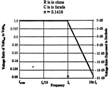
Fig. 6-7. Simplified diagram of how the ratio of volts in/volts out drops rapidly as the cutoff frequency of a filter is exceeded. All signals below the cutoff frequency are passed without attenuation.
