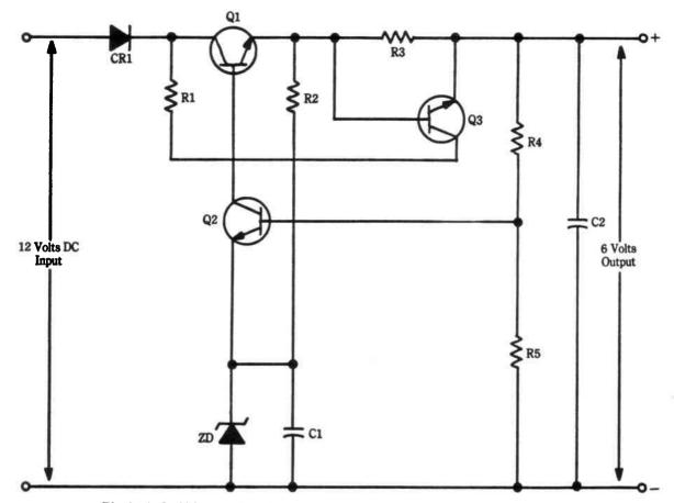
Fig. 24-4. Stabilized 6 volt dc charger operating from a 12 volt battery. Components are:
