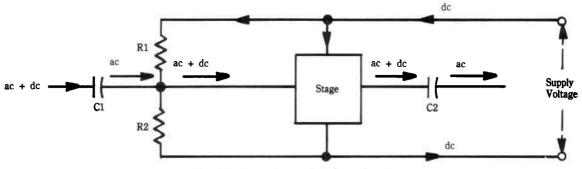
Fig. 3-8. Flow of ac and dc in a circuit.
