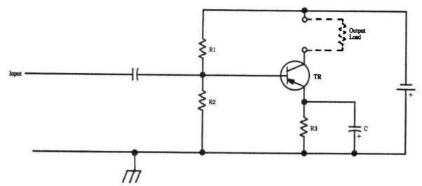
Fig. 16-5. Transistor amplifier stage with stabilized bias. Typical values for low/medium power transistors:
