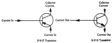
Fig. 18-8. Direction of current flow through PNP and NPN transistors.
