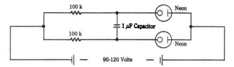
Fig. 10-7. Astable multivibrator circuit, each neon flashing in turn.
