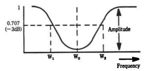
Fig. A-8. Band-stop filter-effect on frequency.
