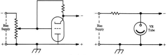
Fig. 25-7. Stabilization by bias voltage.
