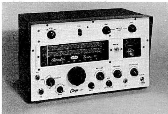
The Clegg Zeus is a special 2-band a-m transmitter, putting out 185 watts on 2 and 6 meters. The modulator and power-supply sections are in a separate cabinet, which can be put out of the way on a shelf.
