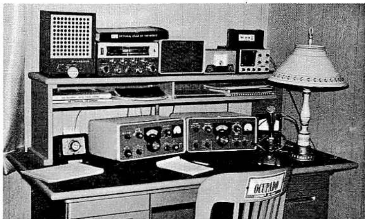
Main units on the desk of a neat ham shack in a corner are matching Collins 75S-3 ssb receiver (left) and 32S-1 transmitter, (right). Built-up shelf holds Heathkit 2-meter transceiver (left), power supply and speaker for Collins gear, antenna indicator, and a Heathkit monitor scope. This is the home station of the author of this book.
