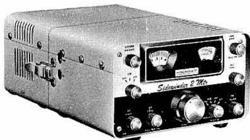
Operating on ssb, am, and cw, the Gonset "Side-winder" 2 is a versatile 2-meter transceiver for mobile or fixed use. Separate transistorized power supplies latch on to the back of the chassis to form a neat package, or can be connected remotely. Receiver section is all-transistor; transmitter section uses mixture of transistors and tubes.
