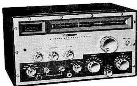
An advanced ssb transmitter for 6 meters only, the Heathkit HX-30 will appeal to hams who like to concentrate on this interesting band. Large slide-rule dial gives accurate frequency readings.
