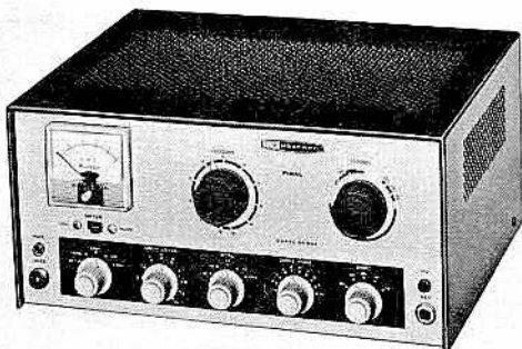
The Heathkit DX-60 is a general-utility cw/am-phone transmitter, rated at 90 watts. It has four positions for crystal control, and provision for connection of an outboard variable-frequency oscillator (vfo).
