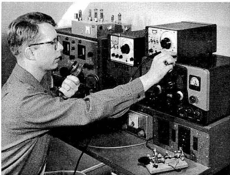
For operation on 6 meters, Herbert F. Holtje, W2TQS, of Tenaflly, N. J., uses the "Li'l Lulu" receiver, the small unit in the center of the photo above his call letters. He is adjusting the controls of the matching "Li'l Lulu" transmitter. These are products of Whippany Labs., Inc., West Caldwell, N. J. For the other ham bands, Bert has a Hammarlund HQ-150 receiver (far left) and a Johnson Ranger transmitter (under his right hand).
