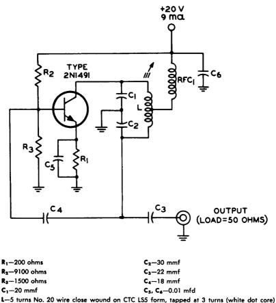
L—5 turns No. 20 wire close wound on CTC LS5 form, tapped at 3 turns (white dot core) RFC1—radio-frequency choke, 10μh
