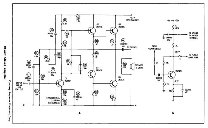
This circuit, as shown, has a low level of distortion. If this low level of distortion is not required, the components used for feedback (resistor R-4 and capacitor C-3) can be changed to increase the gain. It is possible that with an increase in gain, the amplifier might not require the preamplifier, depending on the driving source.
