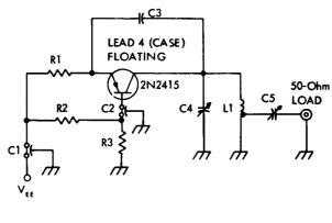
C1 and C2: 1000 pf C3: 1.0 pf C4 and C5: 1.8 - 13 pf L1: 1 1/4" of 3/8" dia. silver-plated brass stock tapped 1 3/16" from ground. R1: 510 Ω, 1/2 W R2: 470 Ω, 1/2 W R3: 2.7 kΩ, 1/2 W
