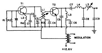
R1-4300 ohm, 1/2 watt R2-820 ohm, 1/2 watt R3-120 ohm, 1/2 watt R4-56 ohm, 1/2 watt C1-100 pf ARCO type DM 10 C2-30 pf ARCO type DM 10 C3, C4, C6-.005 mfd ceramic Lafayette C-611 or Centralab DDM-502 C5-75 pf ARCO type DM 10 C7-50 pf ARCO type DM 10 C9-200 pf ARCO type DM 10 C9-200 pf ARCO type DM 10
