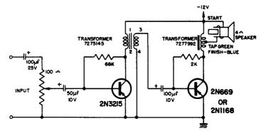
Courtesy Delco Radio Div., General Motors Corp. 2.5-watt audio amplifier.
