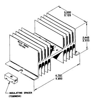
Courtesy Delco Radio Div., General Motors Corp. Fig. C. Delco 7281366 heat sink.
