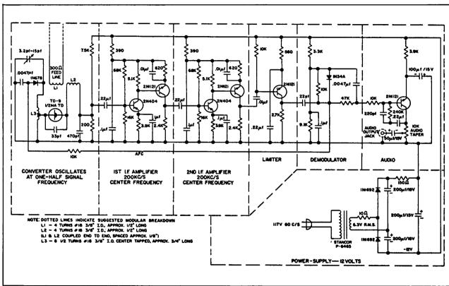
The limiter uses a type 2N1121 transistor as a single-stage limiter feeding the demodulator, a 1N34A diode. The output from the demodulator is fed to the audio module which uses a type 2N1121 transistor as an audio amplifier to provide an audio output to the necessary amplifier. The power-supply module provides 12 volts from a standard a-c line.
