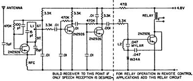
LI - 15 TURNS #24 AWG TAPPED AT 6 TURNS, PROPORTIONED AS SHOWN 6 TURNS/9 TURNS ON CTC #SPCII-4L (CAMBRIDGE THERMIONICS CORPORATION )
