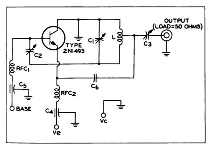
C1-5-50 mmf, variable C2, C3-7-100 mmf, variable C4, C5-feedthrough capacitor, 1500 mmf C6-0.01 mfd L-31/2 turns No. 14 wire, 3/4" diameter, tapped at 2 turns
