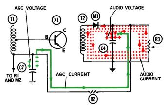
Fig. 5-9. AGC portion of the circuit in Figs. 5-4 and 5-5-modulation peak during a period of strong signal.
