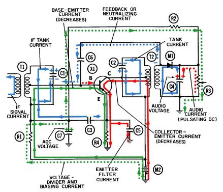
Fig. 5-5. An IF amplifier with AGC diode—positive half-cycle during a period of normal signal strength.
