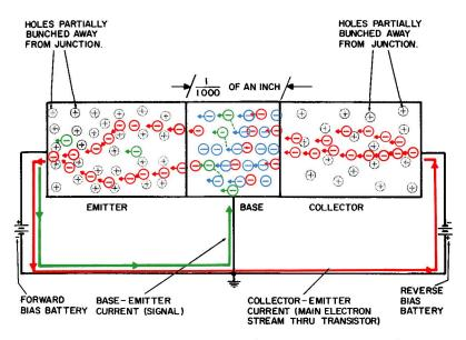
Fig. 1-8. The common-base PNP transistor circuit-no signal current.
