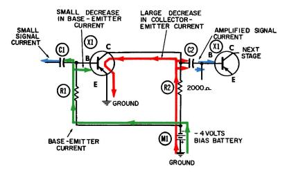
Fig. 1-13. A common-emitter PNP transistor circuit—positive half-cycle.
