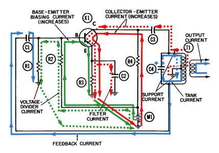
Fig. 3-1. Operation of the Hartley oscillator-negative half-cycle.
