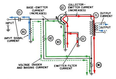
Fig. 4-2. Operation of the Class-A amplifier-positive half-cycle.
