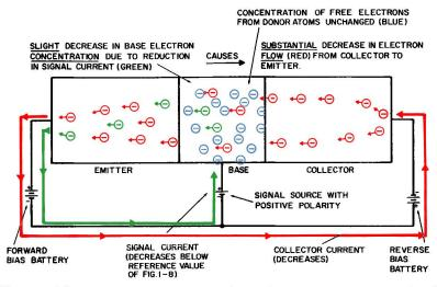
Fig. 1-10. The common-base PNP transistor circuit—positive half-cycle of operation.
