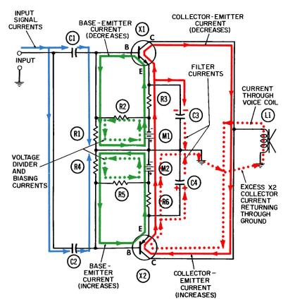
Fig. 4-8. Operation of the complementary symmetry push-pull amplifiernegative half-cycle.
