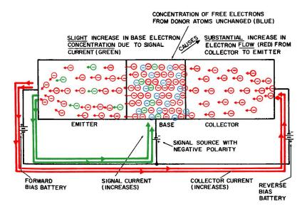
Fig. 1-9. The common-base PNP transistor circuit—negative half-cycle of operation.
