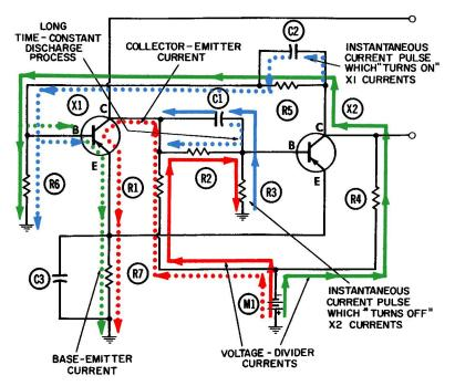
Fig. 3-5. Operataion of the free-running multivibrator-first half-cycle.
