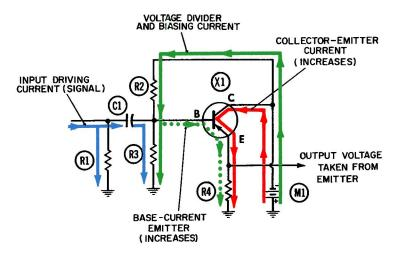
Fig. 2-3. Operation of the common-collector configuration-negative half-cycle.
