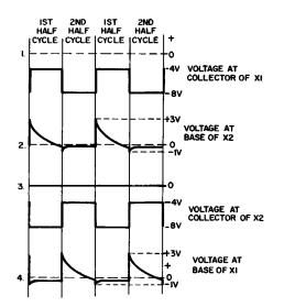
Fig. 3-7. Voltage waveforms in the free-running multivibrator.
