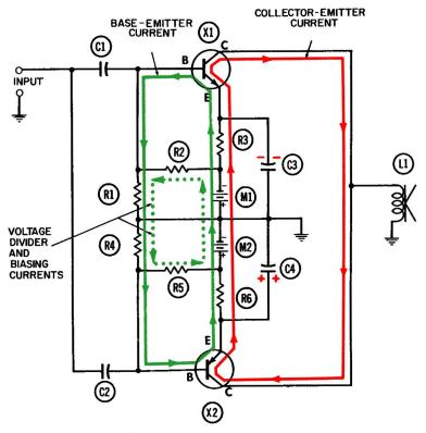
Fig. 4-7. Current conditions in the complementary symmetry push-pull amplifier—static operation with no signal currents.
