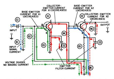
Fig. 4-3. Operation of the direct-coupled amplifier-negative half-cycle.
