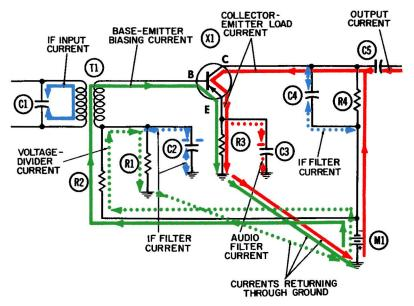
Fig. 5-1. The transistorized detector circuit—conditions leading up to an audio modulation trough.
