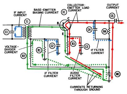
Fig. 5-2. The transistorized detector circuit—conditions leading up to an audio modulation peak.
