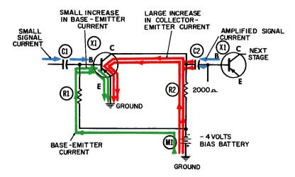
Fig. 1-12. A common-emitter PNP transistor circuit-negative half-cycle.
