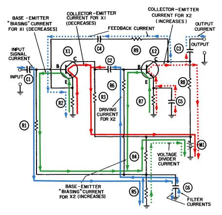
Fig. 4-5. Operation of the resistance-capacitance coupled amplifier with negative feedback—negative half-cycle.
