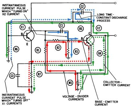
Fig. 3-6. Operation of the free-running multivibrator-second half-cycle.
