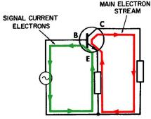
Fig. 1-7. The NPN transistor, with external circuitry.
