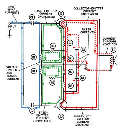
Fig. 4-9. Operation of the complementary symmetry push-pull amplifier positive half-cycle.
