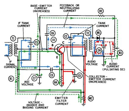
Fig. 5-4. An IF amplifier with AGC diode—negative half-cycle during a period of normal signal strength.
