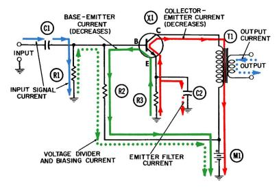
Fig. 4-1. Operation of the Class-A amplifier-negative half-cycle.
