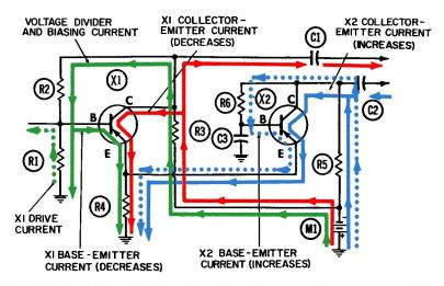
Fig. 2-1. Operation of a two-stage phase inverter using common-emitter and common-base configurations—positive half-cycle.
