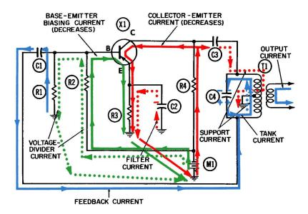
Fig. 3-2. Operation of the Hartley oscillator—positive half-cycle. 52
