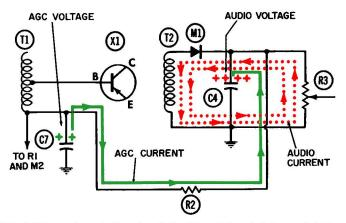
Fig. 5-7. AGC portion of the circuit in Figs. 5-4 and 5-5—modulation peak during a period of weak signal strength.
