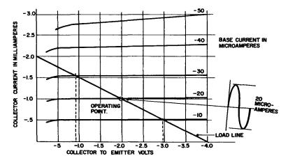
Fig. 1-11. Characteristic curve for a PNP transistor in a common-emitter configuration.
