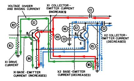
Fig. 2-2. Operation of a two-stage phase inverter using common-emitter and common-base configurations-negative half-cycle.
