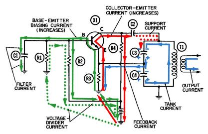
Fig. 3-3. Operation of the Colpitt's oscillator-negative half-cycle.
