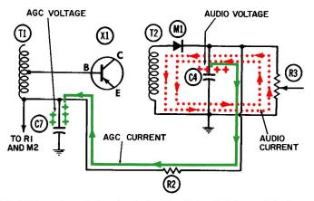
Fig. 5-8. AGC portion of the circuit in Figs. 5-4 and 5-5---modulating trough during a period of strong signal.
