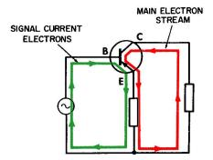
Fig. 1-6. The PNP transistor, with external circuitry.
