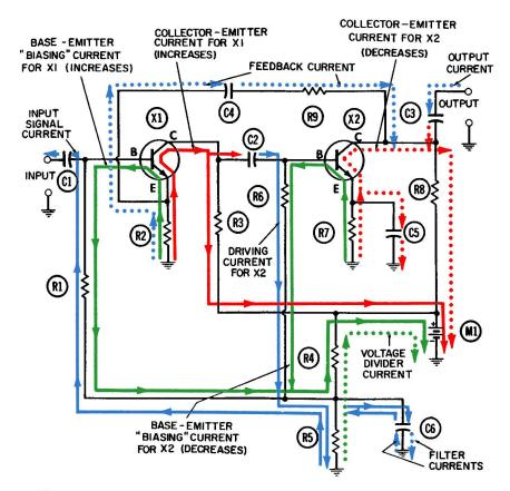
Fig. 4-6. Operation of the resistance-capacitance coupled amplifier with negative feedback-positive half-cycle.
