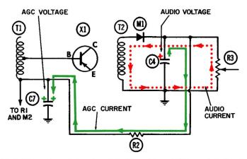
Fig. 5-6. AGC portion of the circuit in Figs. 5-4 and 5-5—modulation trough during a period of weak signal strength.
