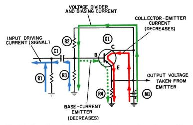
Fig. 2-4. Operation of the common-collector configuration—positive half-cycle.
