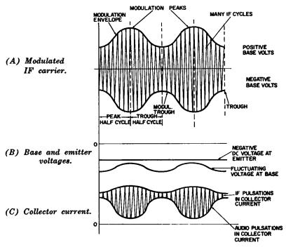
Fig. 5-3. Waveform diagrams for the transistorized detector.
