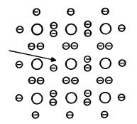
Fig. 1-2. A boron atom tied to four germanium atoms.
