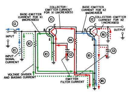
Fig. 4-4. Operation of the direct-coupled amplifier-positive half-cycle.
