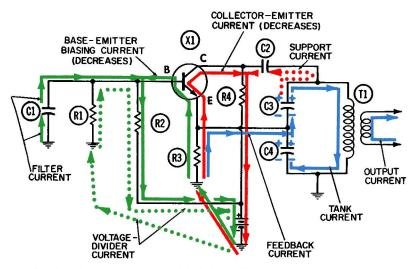
Fig. 3-4. Operation of the Colpitt's oscillator-positive half-cycle.
