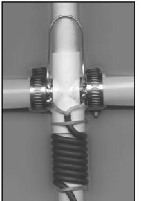
Fig 45—Photo of driven-element mounted to PVC tee using hose clamps. The hairpin match wires is shown here soldered to the tapemeasure elements, along with the RG-58 feed line.
