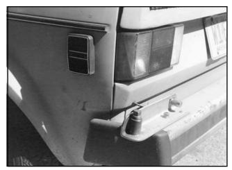
Fig 36—The mount for the mobile J is made from stainless-steel angle stock and secured to the bumper with stainless-steel hardware. Note the <sup>1</sup>/<sub>2</sub>-inch pipe plug and a PL-259 (with a copper disc soldered in its unthreaded end). These protect the mount and connector threads when the antenna is not in use.
