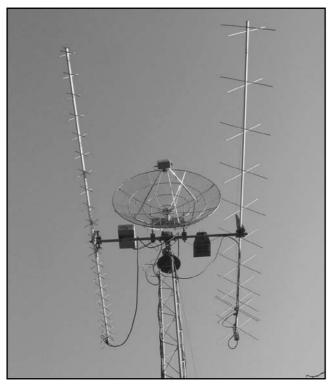
Fig 22—Wilfred Carey, ZS6JT, constructed this cluster of satellite and EME antennas. Left to right:  $2 \times$ 23-element offset feed Yagi for U band; 1.64-meter dish with 2<sup>1</sup>/<sub>4</sub>-turn helix feed for S band;  $2 \times 11$ -element coplanar feed Yagi for V band. (*ZS6JT photo.*)
