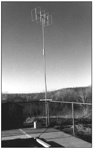
Fig 56—The 4-element 144-MHz portable quad, assembled and ready for operation. Sections of clothes closet poles joined with pine strips make up the mast. (*Photo by Adwin Rusczek, W1MPO*)
