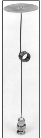
A combination of top and center loading offers improved efficiency over continuously loaded antennas such as the "stubby" pictured at the beginning of this chapter. This antenna also offers low construction cost. The only materials needed are a length of stiff wire and a scrap of circuit-board material, in addition to the appropriate connector.
