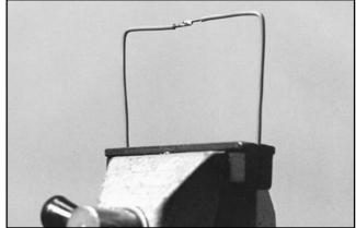
Fig 67—These photos show the construction method used for the 1296-MHz quad type parasitic elements. The two ends of the #18 bell wire are brought together with an overlap of  $1/_8$  in. and soldered.
