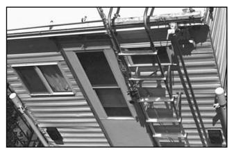
Fig 13—Photo showing the back of the camper, with the antenna in the lowered position, parallel to the ladder. The "Outback" standby mobile antenna is shown clamped to the left side of the ladder.
