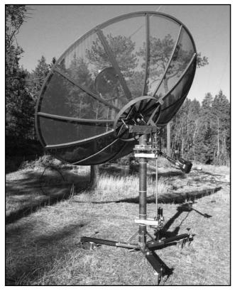
Fig 69—A completed TVRO dish Az-El mounting system is shown, using a jackscrew elevation drive. (*WØLMD photo.*)
