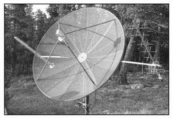
Fig 24—WØLMD graduated to this 8-foot dish with patch feed for S band for AO-40. On the left is a helical antenna for L band and on the right is a 2 × 9-element offset-feed Yagi for U band. A home-brew Az-El mount is provided. (*WØLMD photo*.)
