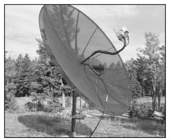
Fig 25—WØLMD increased to this 10-foot dish for AO-40 operations, with a triband patch feed for U, L, and S bands on an Az-EI mount. (*WØLMD photo.*)
