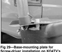
Screw-driver installation on KO4TV's truck. Note the quick-disconnect dc motor con-nections and the SO-239 coax connector.
