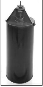
Fig 16—A coaxial cavity filter of the type used in many amateur and commercial repeater installations. Centerconductor length (and thus resonant frequency) is varied by adjustment of the knob (top).
