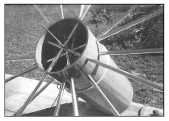
Fig 54—Photo showing details of the hub assembly for the large discone, including the threaded brass rod that connects the radial spreaders together. The 10-inch PVC pipe is drilled to accommodate the radial spreaders. Each spreader is reinforced with a three-foot long wooden dowel inside for crush resistance. Note the row of holes drilled below the lowest spreader. Each of the 36 cone wire passes through one of these holes.
