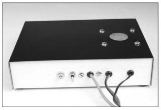
Fig 43—The rear panel of the DF unit supports the two DPDT PHASE toggle switches. Grommets in the panel holes allow abrasion-free passage of the antenna, dcpower and audio cables. The dc power cord is outfitted with an inline fuse holder and a male Jones plug. A sixpin female Molex connector (five pins are used) feeds the four antennas. The audio-input cable is terminated in a 1/<sub>8</sub>-inch diameter male plug.
