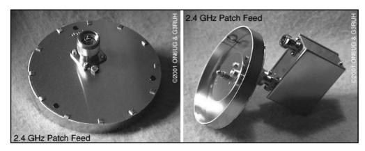
Fig 47—Details of CP-patch feed for short f/D dish antennas by G3RUH and ON6UG.
