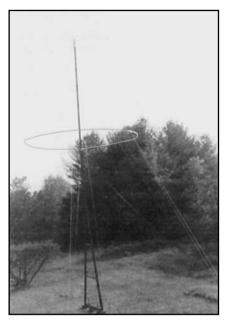
Fig 50—Photo of W8NWF's original A-frame mounted HF discone.
