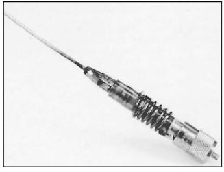
Fig 51—The 220-MHz  $5/6-\lambda$  mobile antenna. The coil turns are spaced over a distance of 1 inch, and the bottom end of the coil is soldered to the coax connector.
