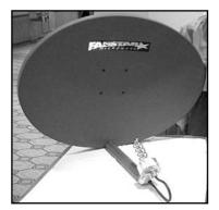
Fig 30—PrimeStar offset-fed dish with WD4FAB's helix-feed antenna. NØNSV was so pleased with the modification that he renamed the dish "FABStar," and made a new label! (NØNSV photo.)
