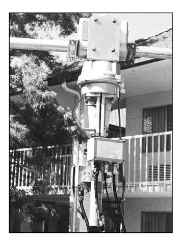
Fig 65—At left, Yaesu Az-El antenna-rotator mounting system is shown. Note that antenna loads must be more carefully balanced on this rotator than in the previously shown systems. At right, VE5FP has a solution for his Az-El rotators by bolting two of them together in his "An Inexpensive Az-El Rotator System", *QST*, December 1998.
