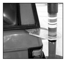
Fig 30—The support Plexiglas plate. (*Photo courtesy of Gary Pearce, KN4AQ.*)
