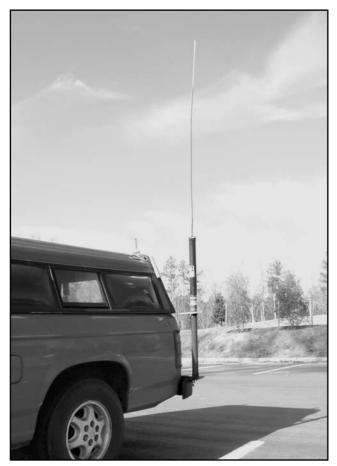
Fig 23—The completed Screwdriver antenna mounted on KO4TV's truck rear bumper. (*Photo courtesy of Gary Pearce, KN4AQ.*)
